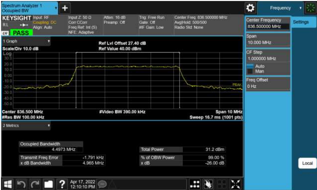
Sub6 n5. Occupied Bandwidth Plot (5 M BW Ch.167300 QPSK_ Full RB _0)
