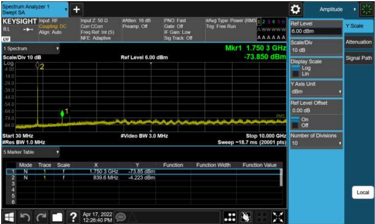
Sub6 n5. Conducted Spurious Plot (168800ch_10 MHz_BPSK_RB 1_1)
