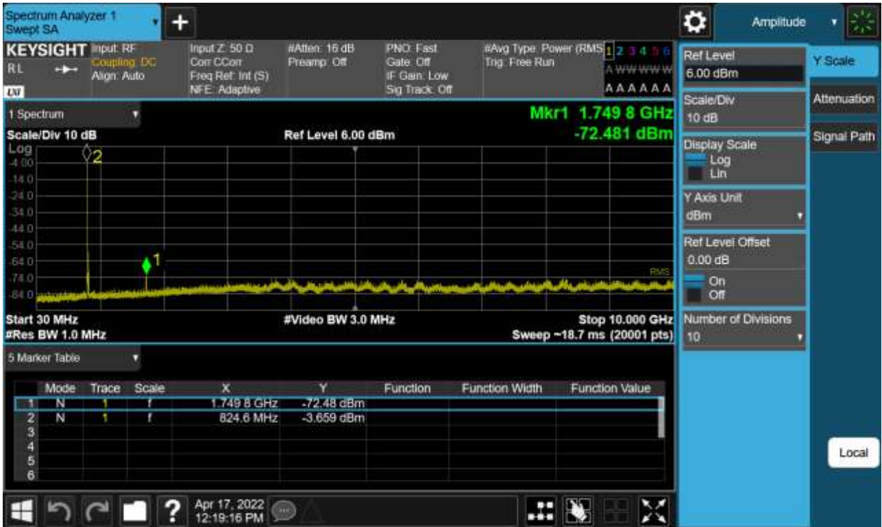
Sub6 n5. Conducted Spurious Plot (165800ch_10 MHz_BPSK_RB 1_1)
