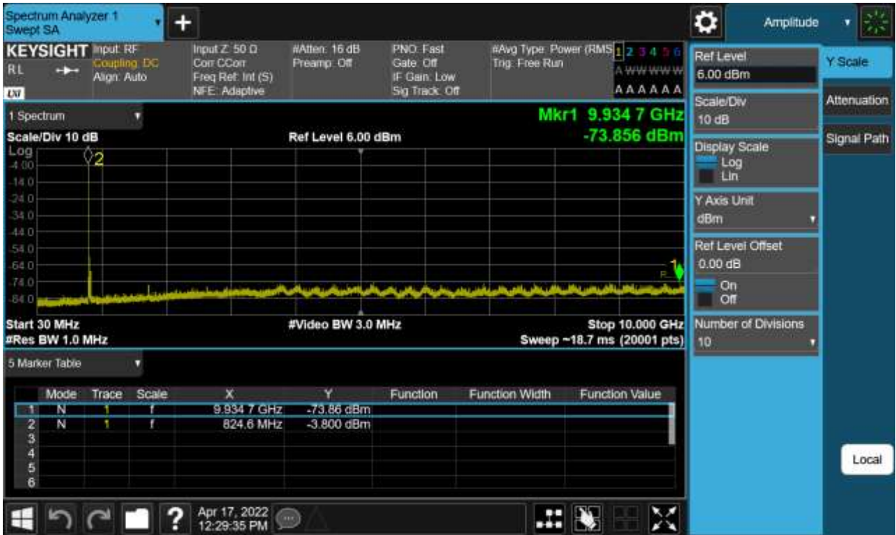
Sub6 n5. Conducted Spurious Plot (166300ch_15 MHz_BPSK_RB 1_1)
