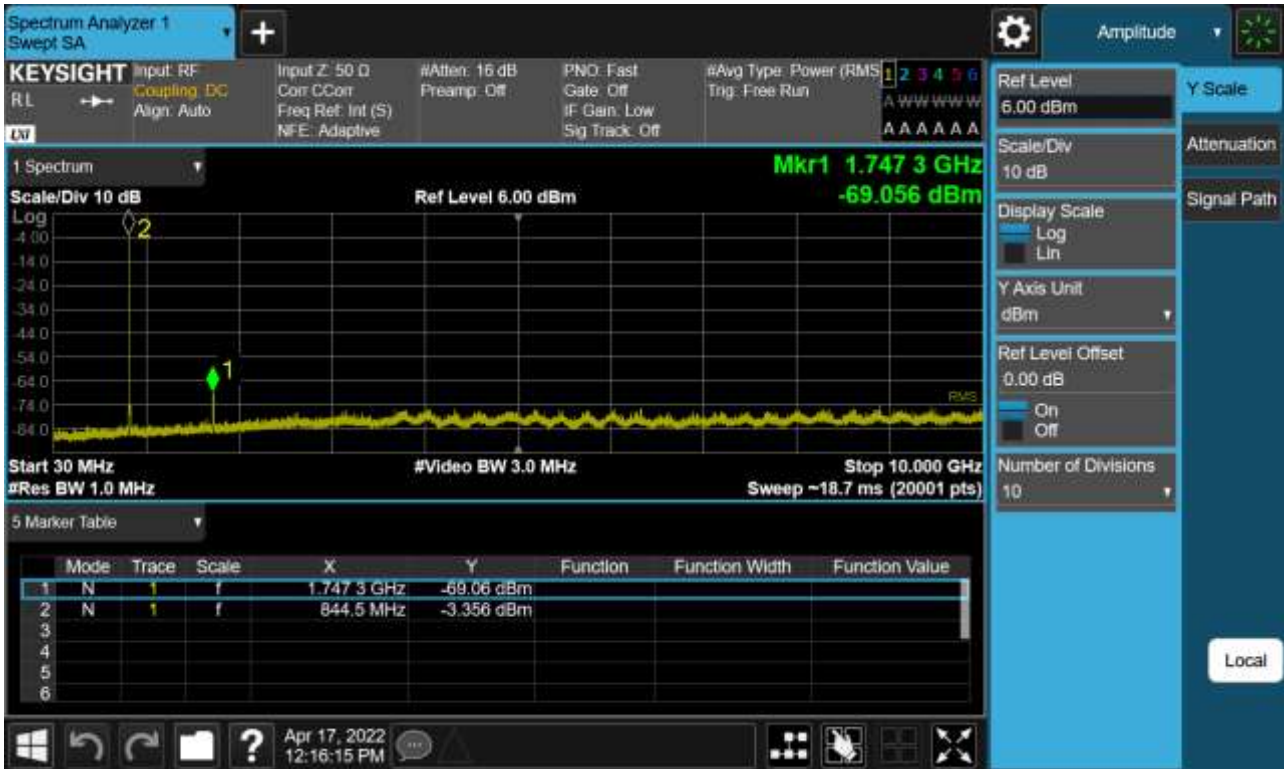
Sub6 n5. Conducted Spurious Plot (169300ch_5 MHz_BPSK_RB 1_1)
