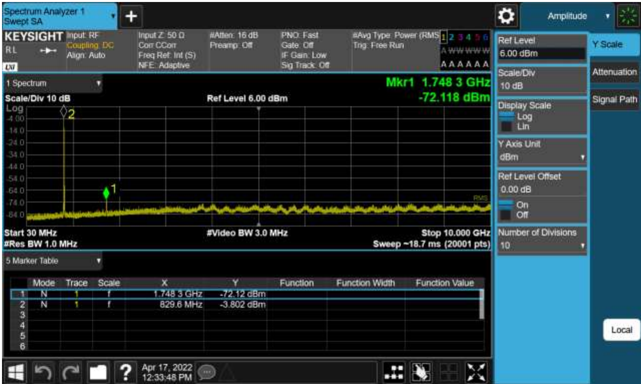
Sub6 n5. Conducted Spurious Plot (167300ch_15 MHz_BPSK_RB 1_1)
