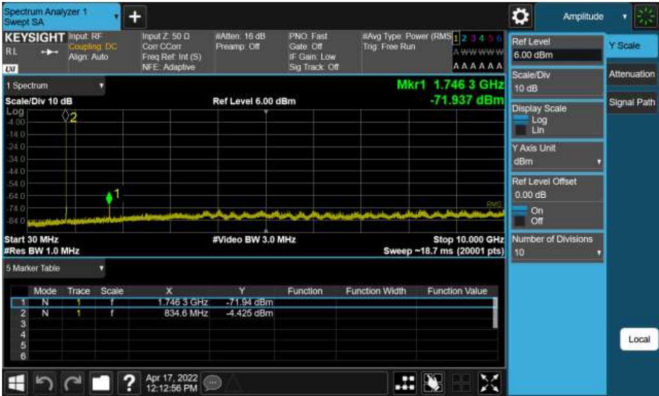
Sub6 n5. Conducted Spurious Plot (167300ch_5 MHz_BPSK_RB 1_1)
