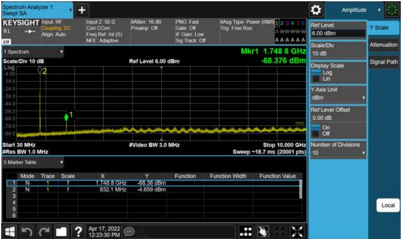
Sub6 n5. Conducted Spurious Plot (167300ch_10 MHz_BPSK_RB 1_1)
