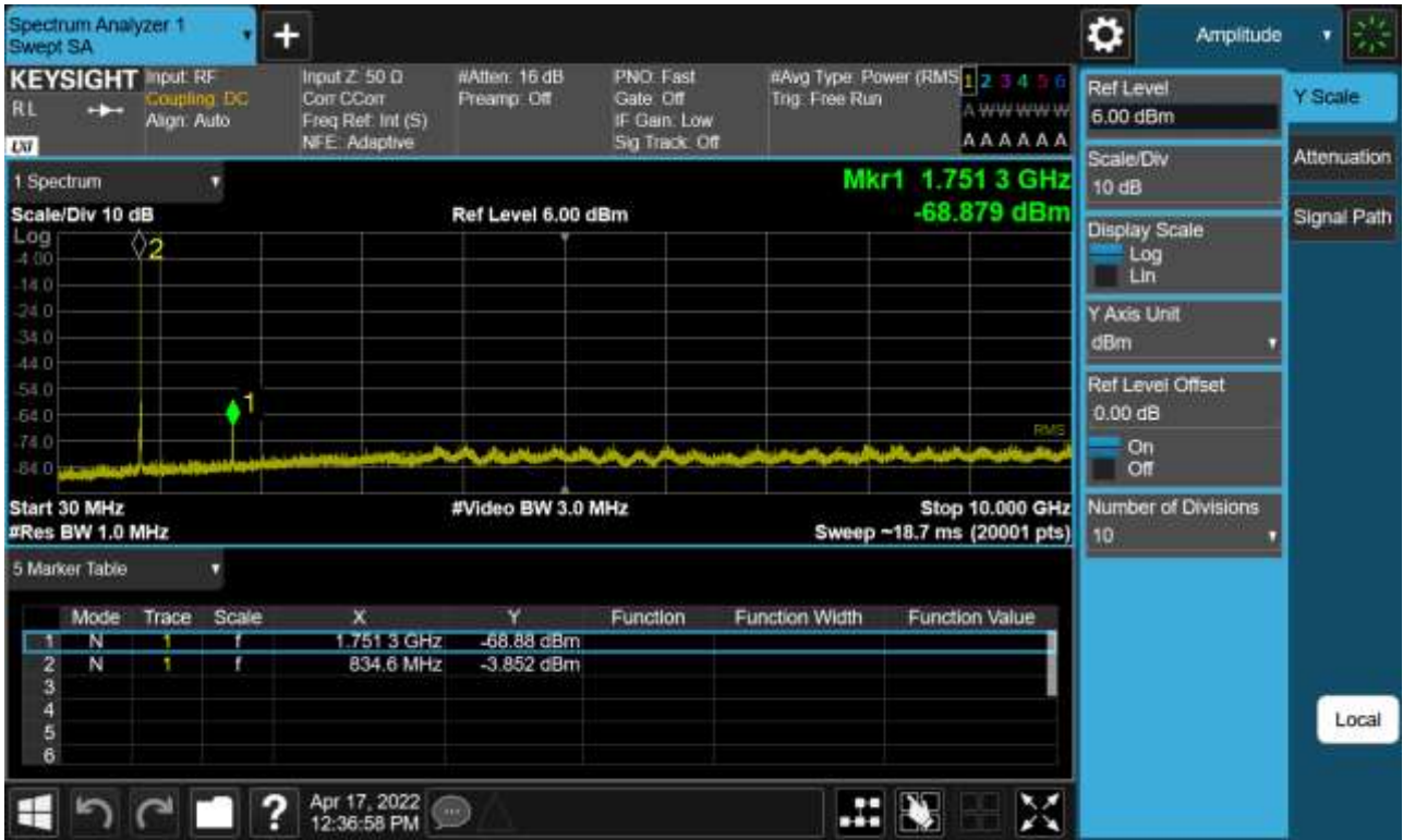
Sub6 n5. Conducted Spurious Plot (168300ch_15 MHz_BPSK_RB 1_1)
