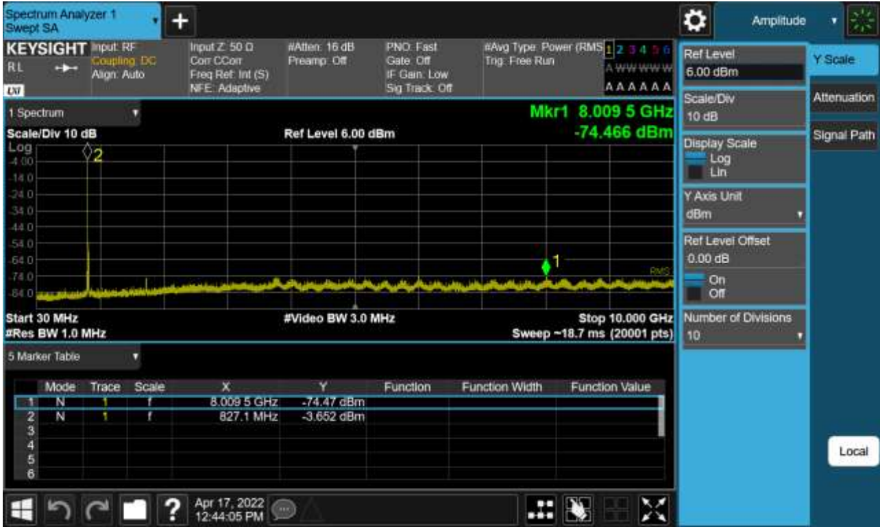
Sub6 n5. Conducted Spurious Plot (167300ch_20 MHz_BPSK_RB 1_1)
