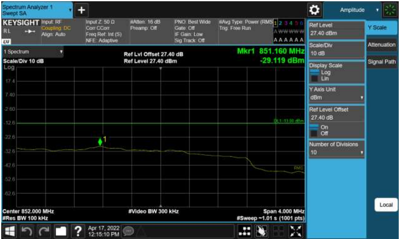
Sub6 n5. Upper Extended Band Edge Plot (5 M BW Ch.169300 BPSK_RB25_0)
