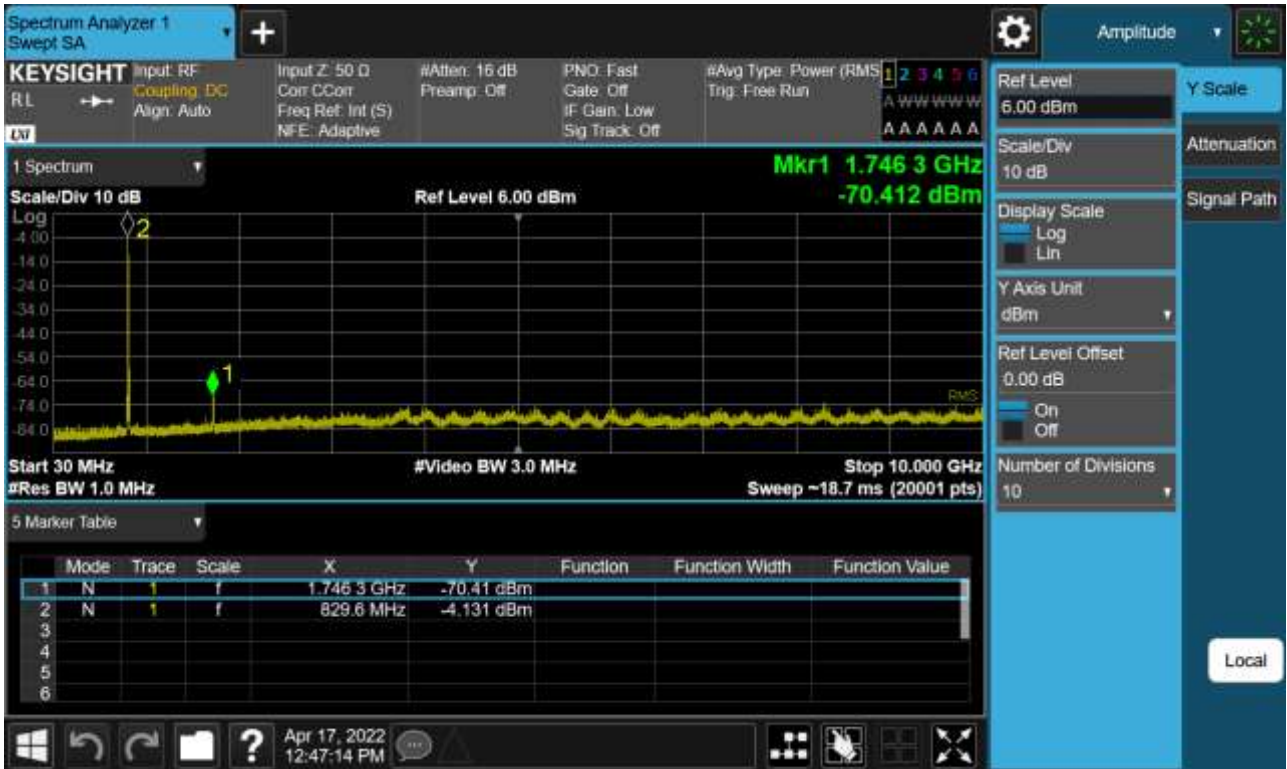
Sub6 n5. Conducted Spurious Plot (167800ch_20 MHz_BPSK_RB 1_1)
