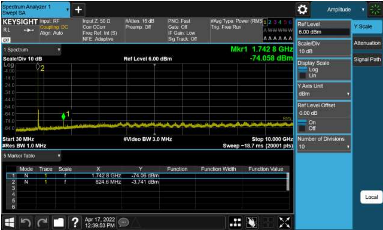
Sub6 n5. Conducted Spurious Plot (166800ch_20 MHz_BPSK_RB 1_1)
