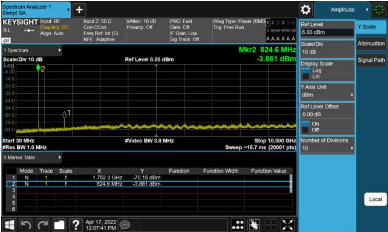
Sub6 n5. Conducted Spurious Plot (165300ch_5 MHz_BPSK_RB 1_1)
