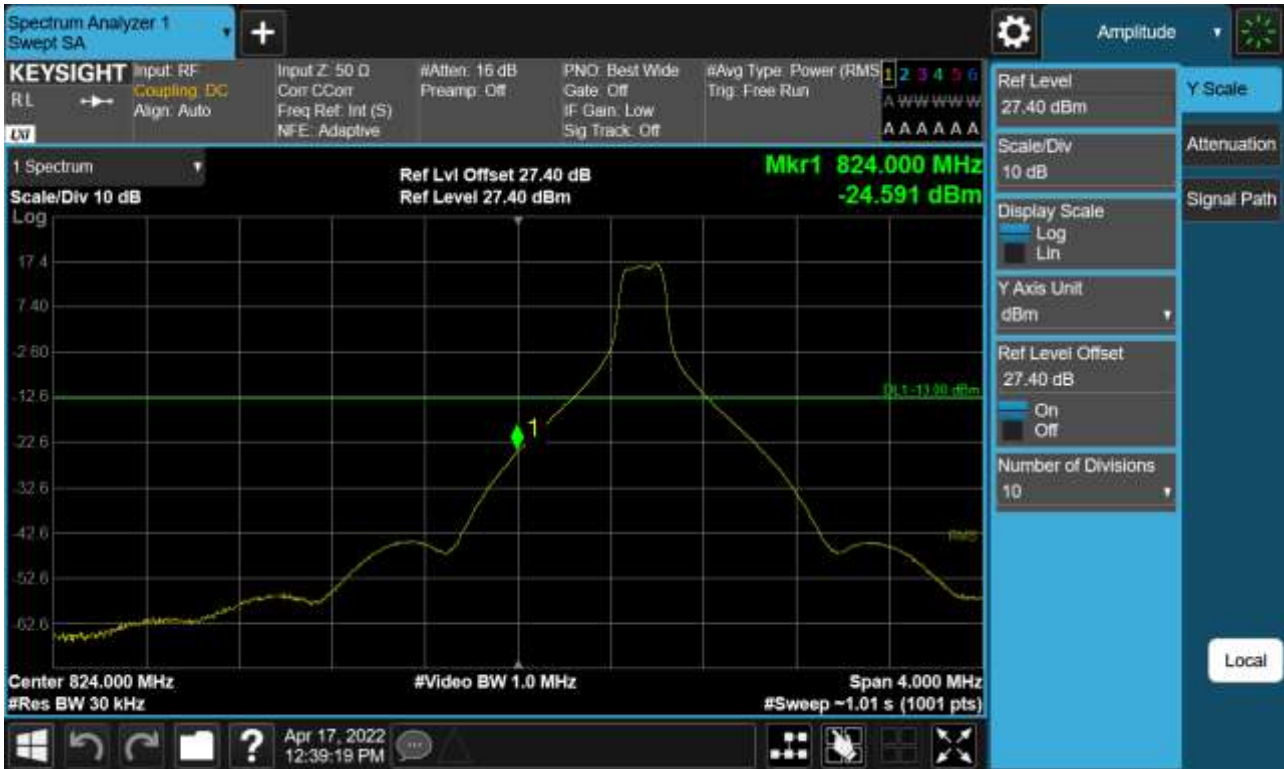
Sub6 n5. Lower Band Edge Plot (20 M BW Ch.166800 BPSK_RB1_Offset 0)
