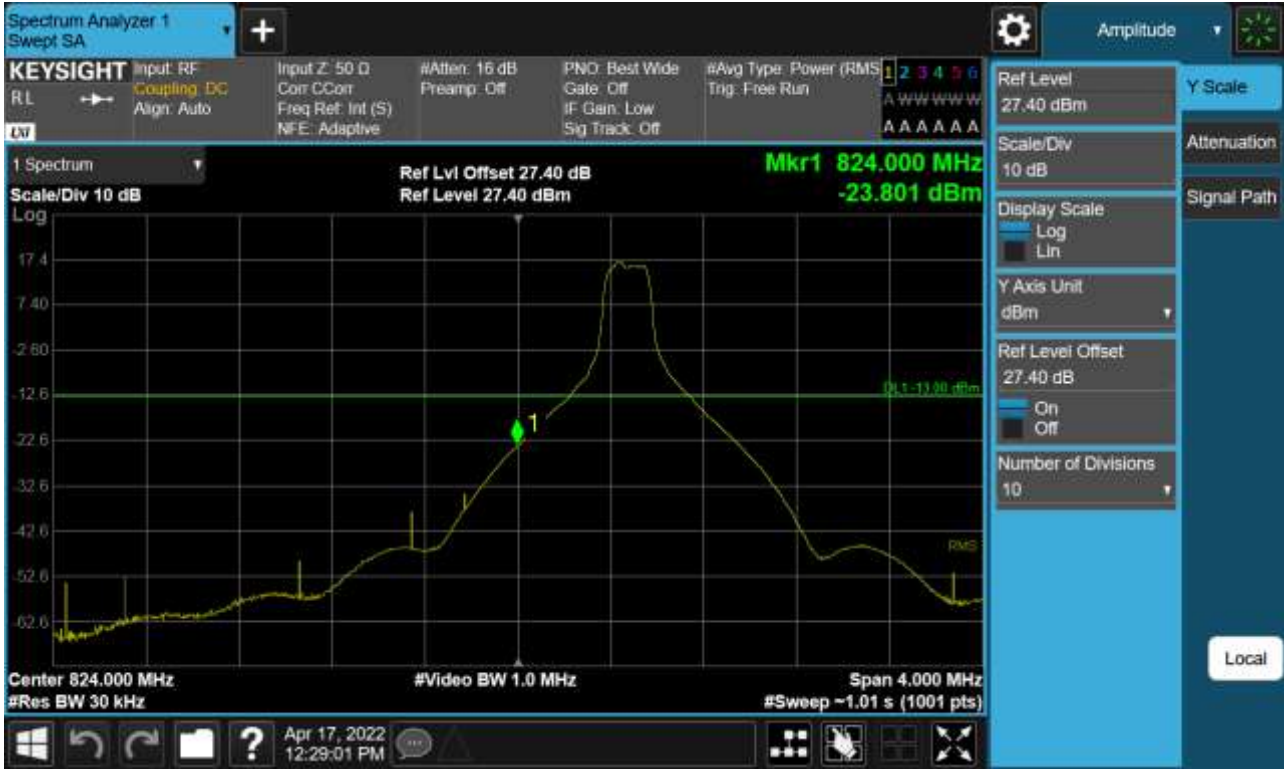
Sub6 n5. Lower Band Edge Plot (15 M BW Ch.166300 BPSK_RB1_Offset 0)
