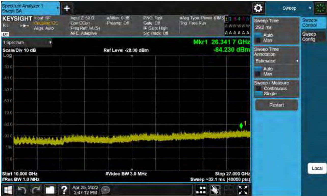
Sub6 n41. Conducted Spurious Plot 2 (60 MHz Ch.506004 BPSK RB 1)
