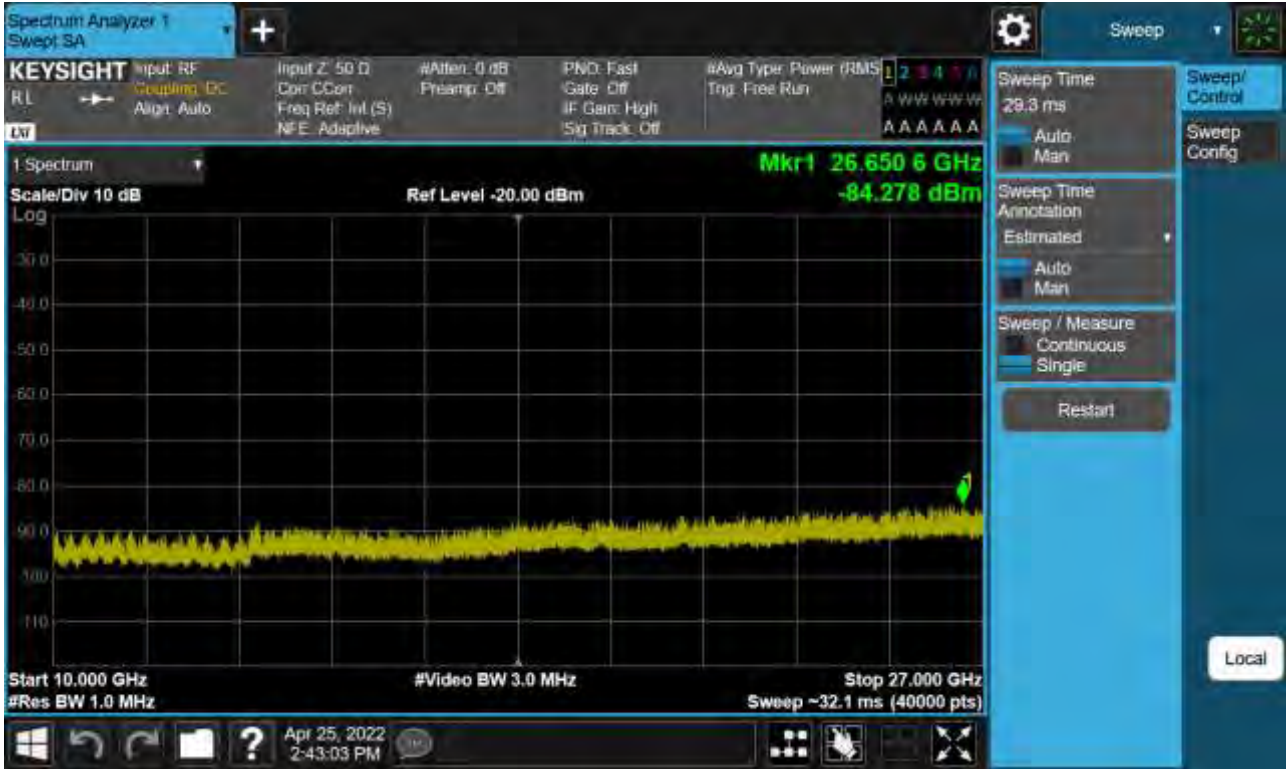
Sub6 n41. Conducted Spurious Plot 2 (50 MHz Ch.505002 BPSK RB 1)
