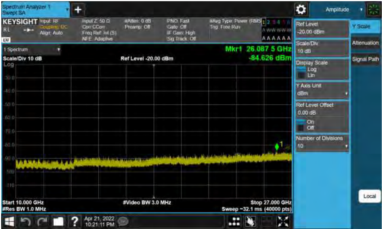
Sub6 n41. Conducted Spurious Plot 2 (80 MHz Ch. 518598 BPSK RB 1)
