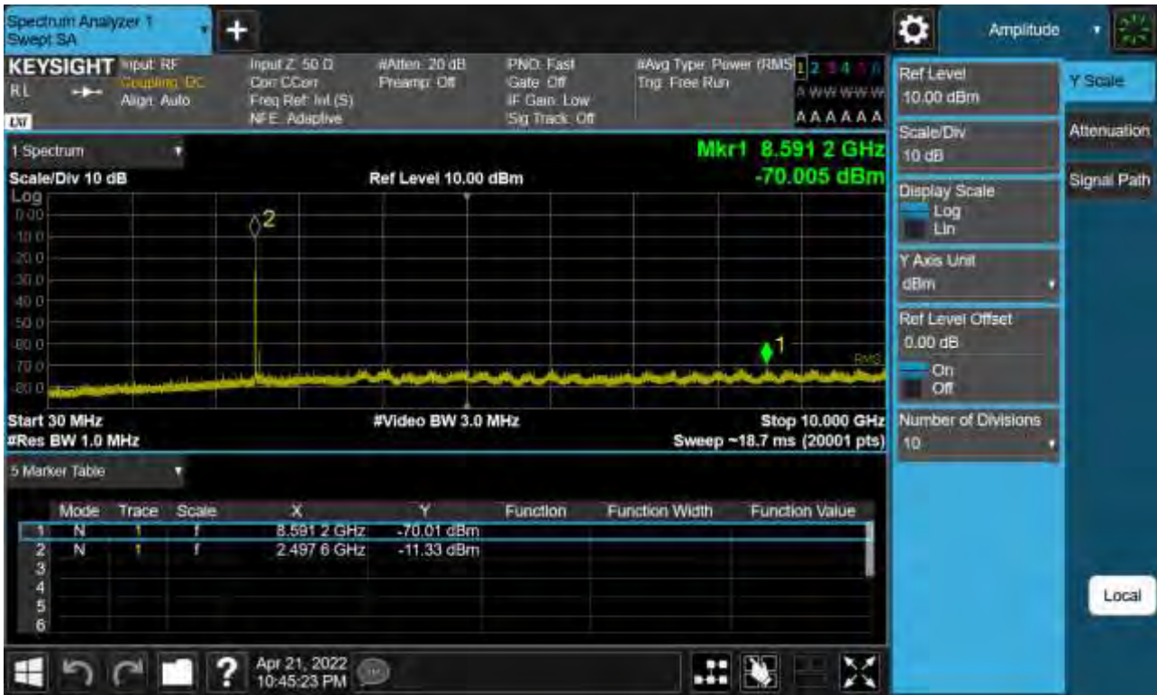
Sub6 n41. Conducted Spurious Plot 1 (100 MHz Ch.509202 BPSK RB 1)
