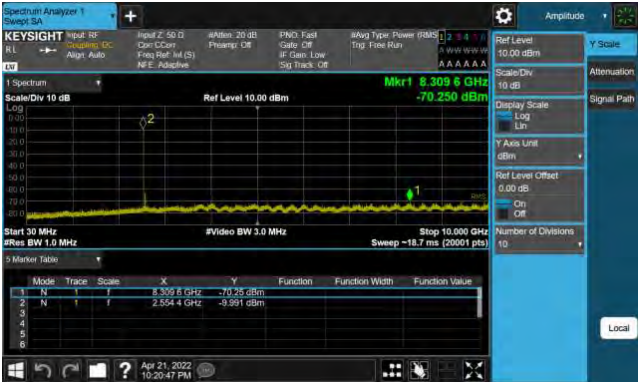
Sub6 n41. Conducted Spurious Plot 1 (80 MHz Ch.518598 BPSK RB 1)
