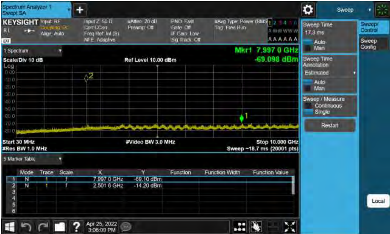
Sub6 n41. Conducted Spurious Plot 1 (100 MHz Ch.510000 BPSK RB 1)
