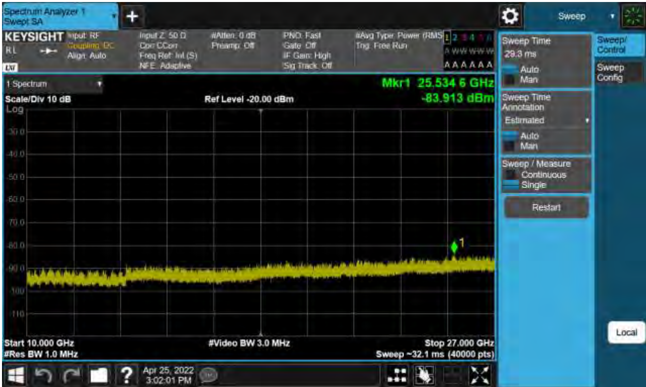
Sub6 n41. Conducted Spurious Plot 2 (90 MHz Ch.509004 BPSK RB 1)
