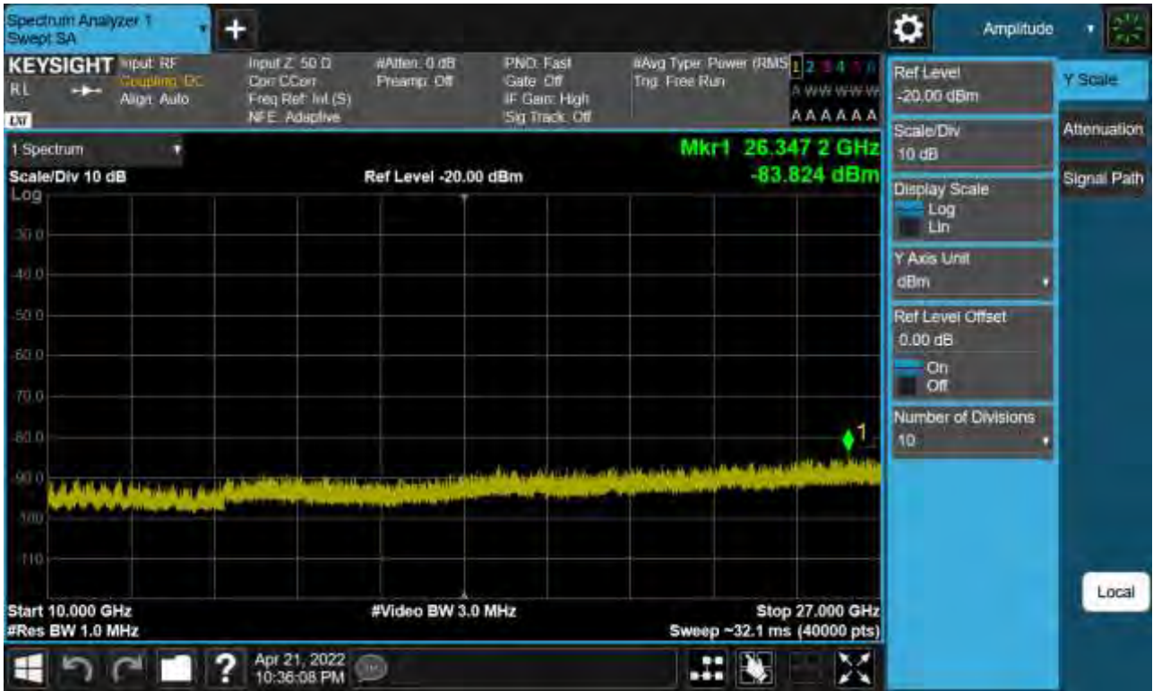
Sub6 n41. Conducted Spurious Plot 2 (90 MHz Ch. 518598 BPSK RB 1)
