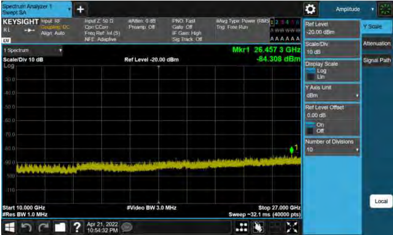
Sub6 n41. Conducted Spurious Plot 2 (100 MHz Ch.528000 BPSK RB 1)
