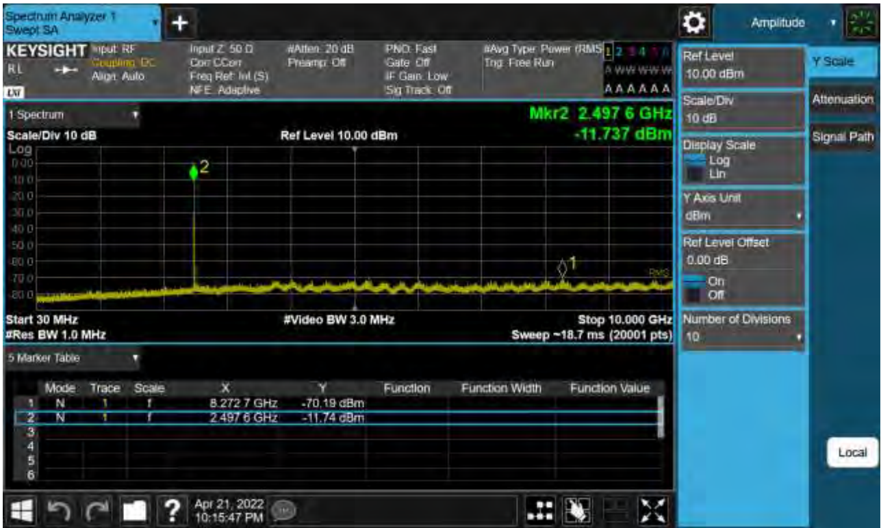
Sub6 n41. Conducted Spurious Plot 1 (80 MHz Ch.507204 BPSK RB 1)
