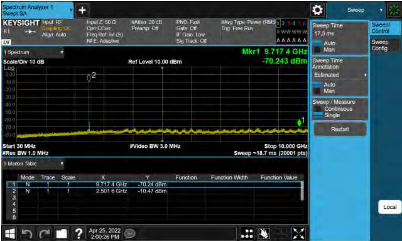
Sub6 n41. Conducted Spurious Plot 1 (40 MHz Ch.504000 BPSK RB 1)
