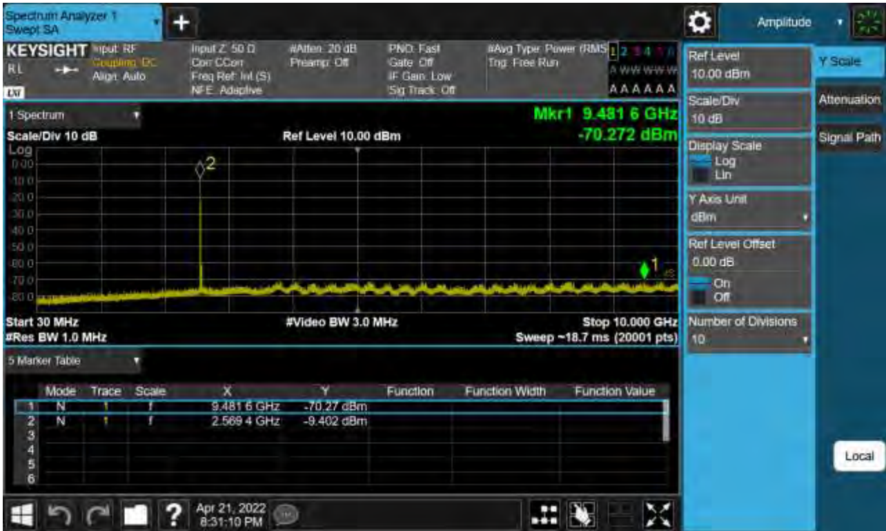
Sub6 n41. Conducted Spurious Plot 1 (50 MHz Ch.518598 BPSK RB 1)
