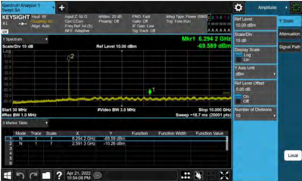
Sub6 n41. Conducted Spurious Plot 1 (100 MHz Ch.528000 BPSK RB 1)
