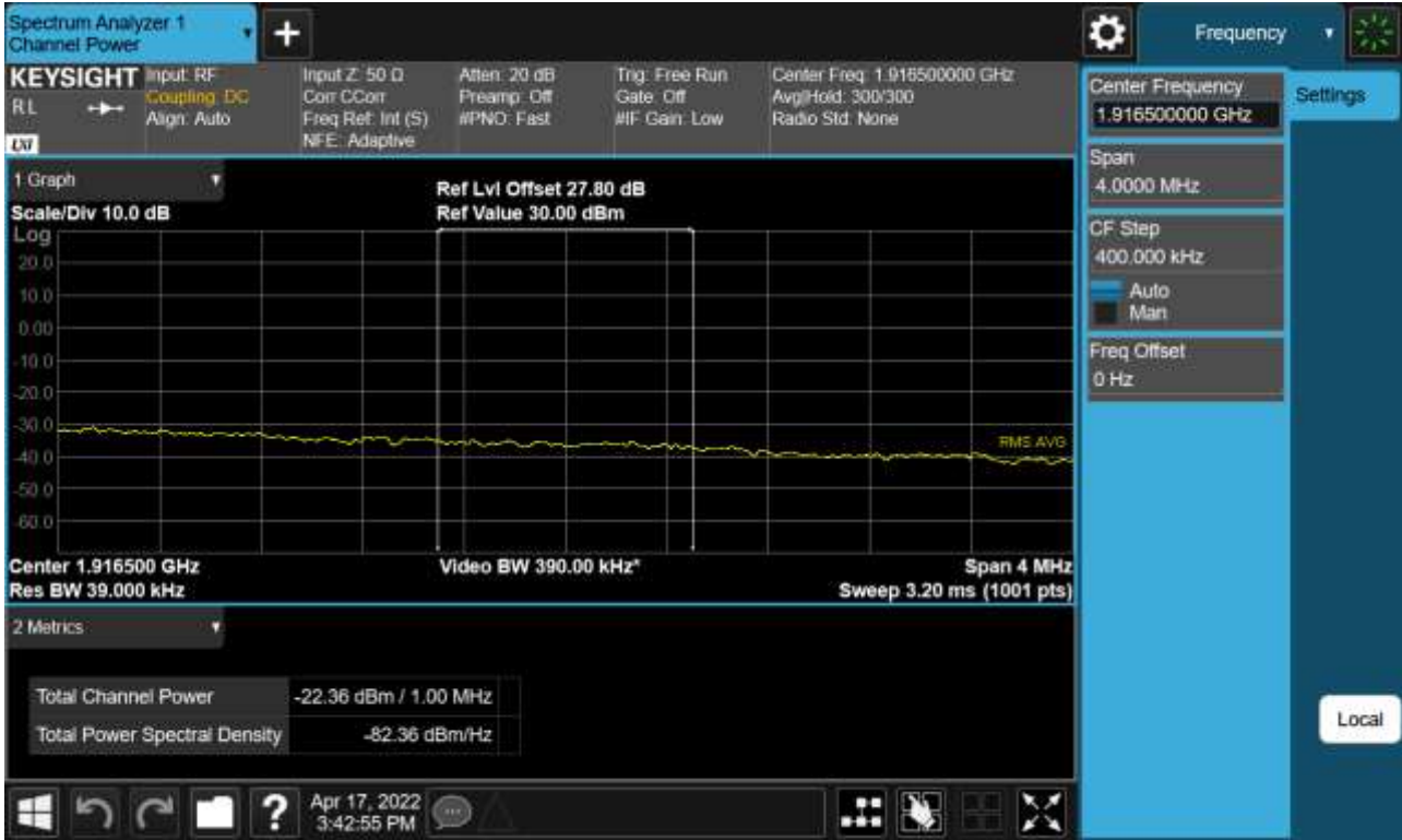
Sub6 n25(2). Upper Extended Band Edge Plot (20 M BW Ch.381000 BPSK_RB100_0) -2
