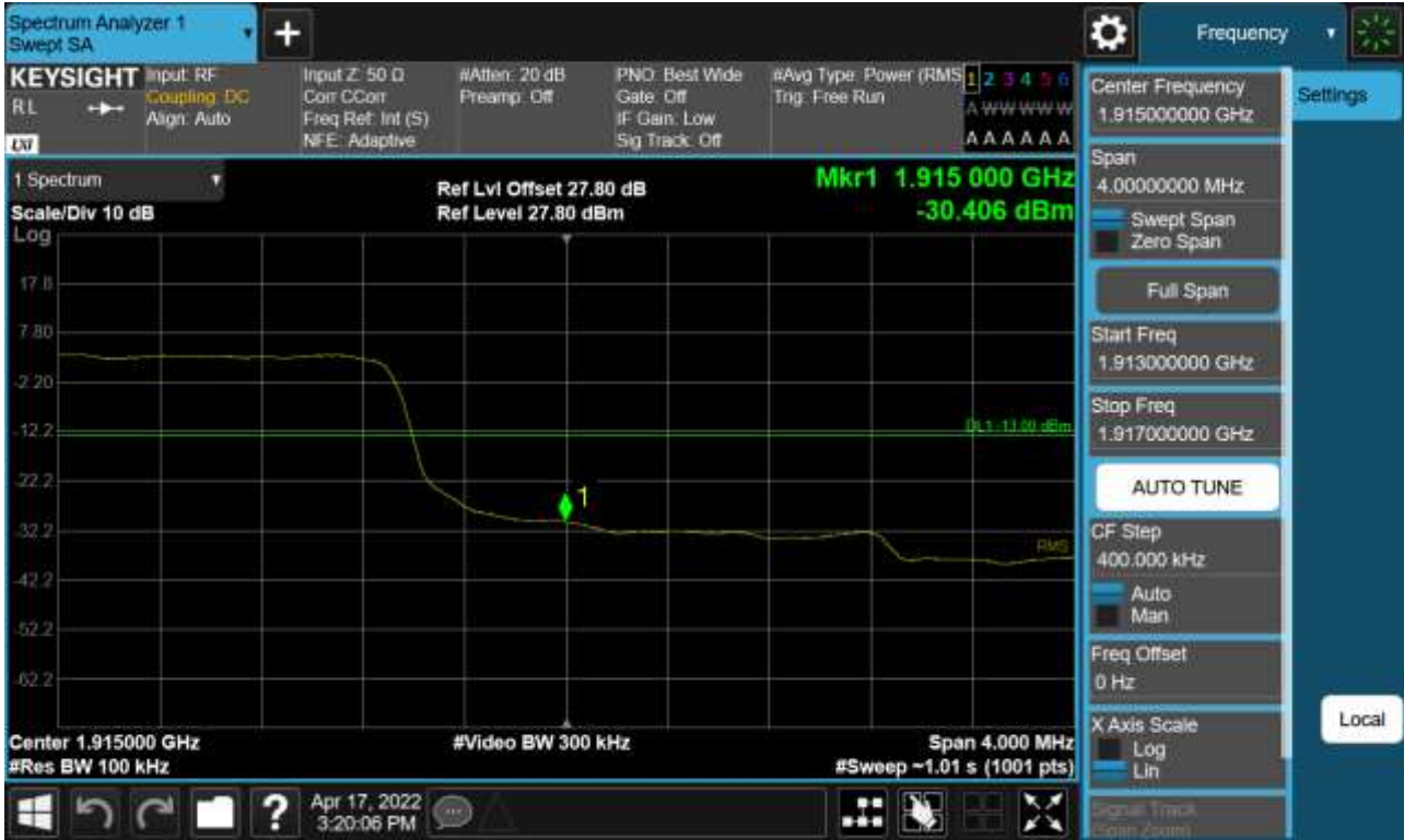
Sub6 n25(2). Upper Band Edge Plot (10 M BW Ch.382000 BPSK_RB50_Offset 0) -1
