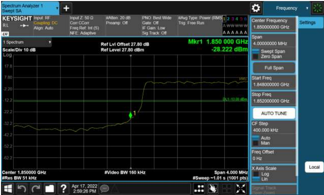
Sub6 n25(2). Lower Band Edge Plot (5 M BW Ch.370500 BPSK_RB25_Offset 0) -1
