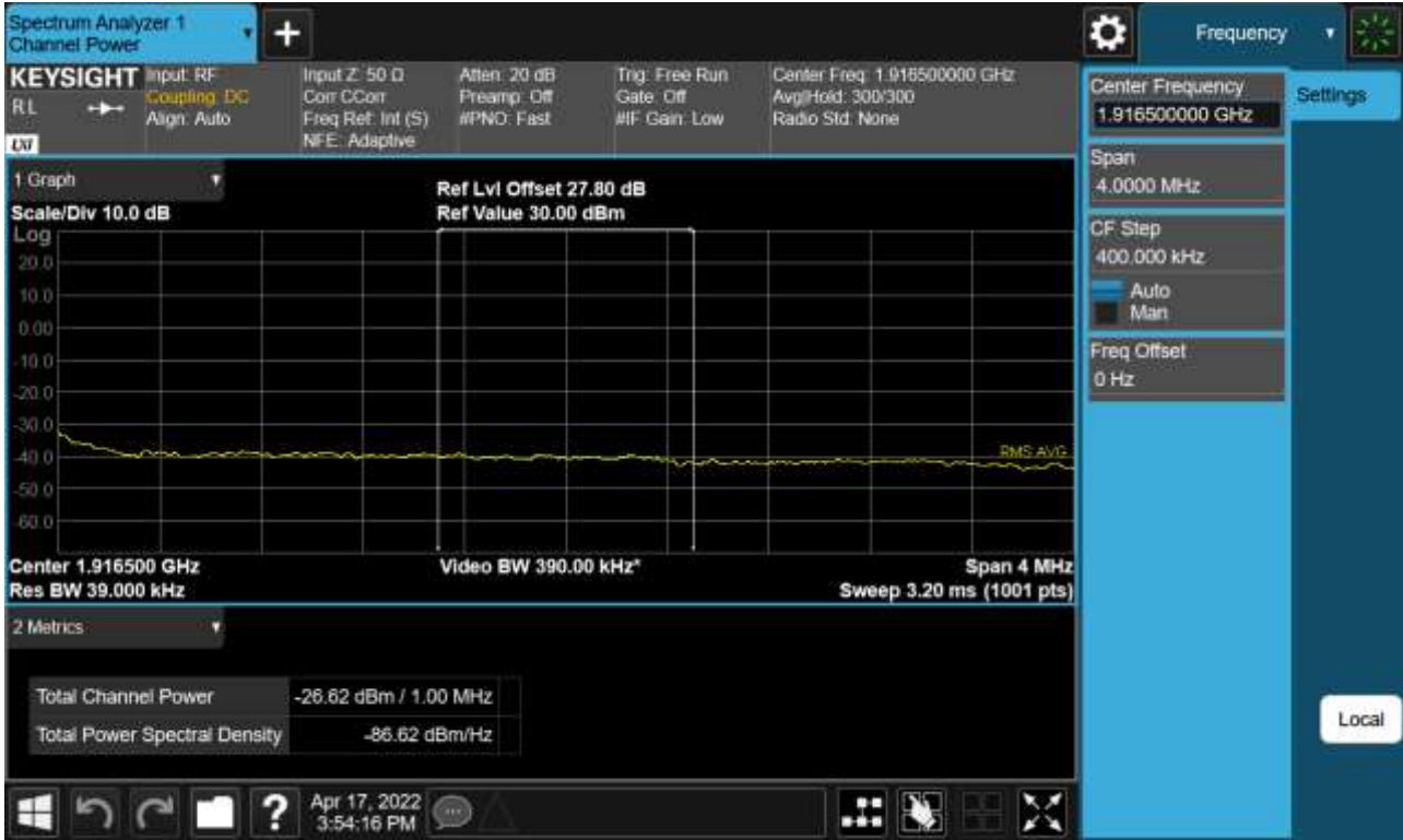
Sub6 n25. Upper Extended Band Edge Plot (30 M BW Ch.380000 BPSK_RB160_0) -2
