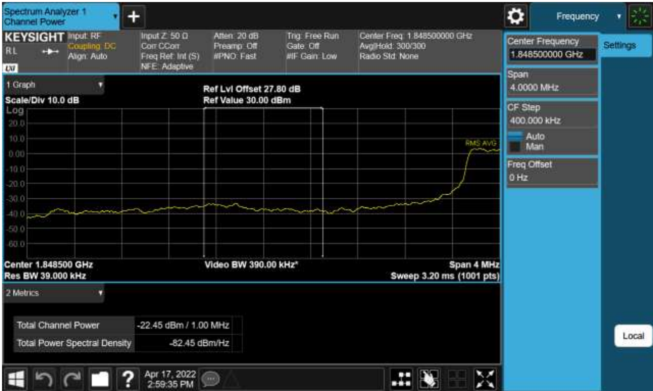
Sub6 n25(2). Lower Extended Band Edge Plot (5 M BW Ch.370500 BPSK_RB25_0) -2
