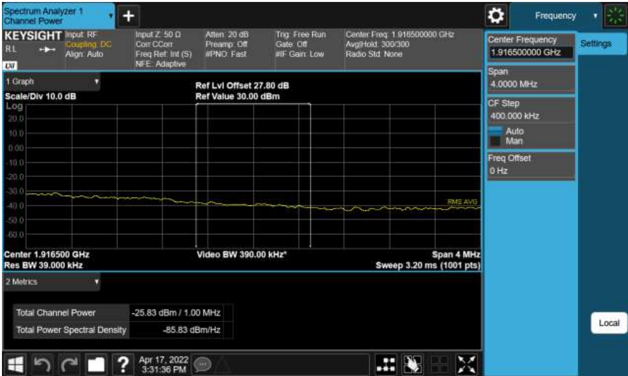
Sub6 n25(2). Upper Extended Band Edge Plot (15 M BW Ch.381500 BPSK_RB75_0) -2
