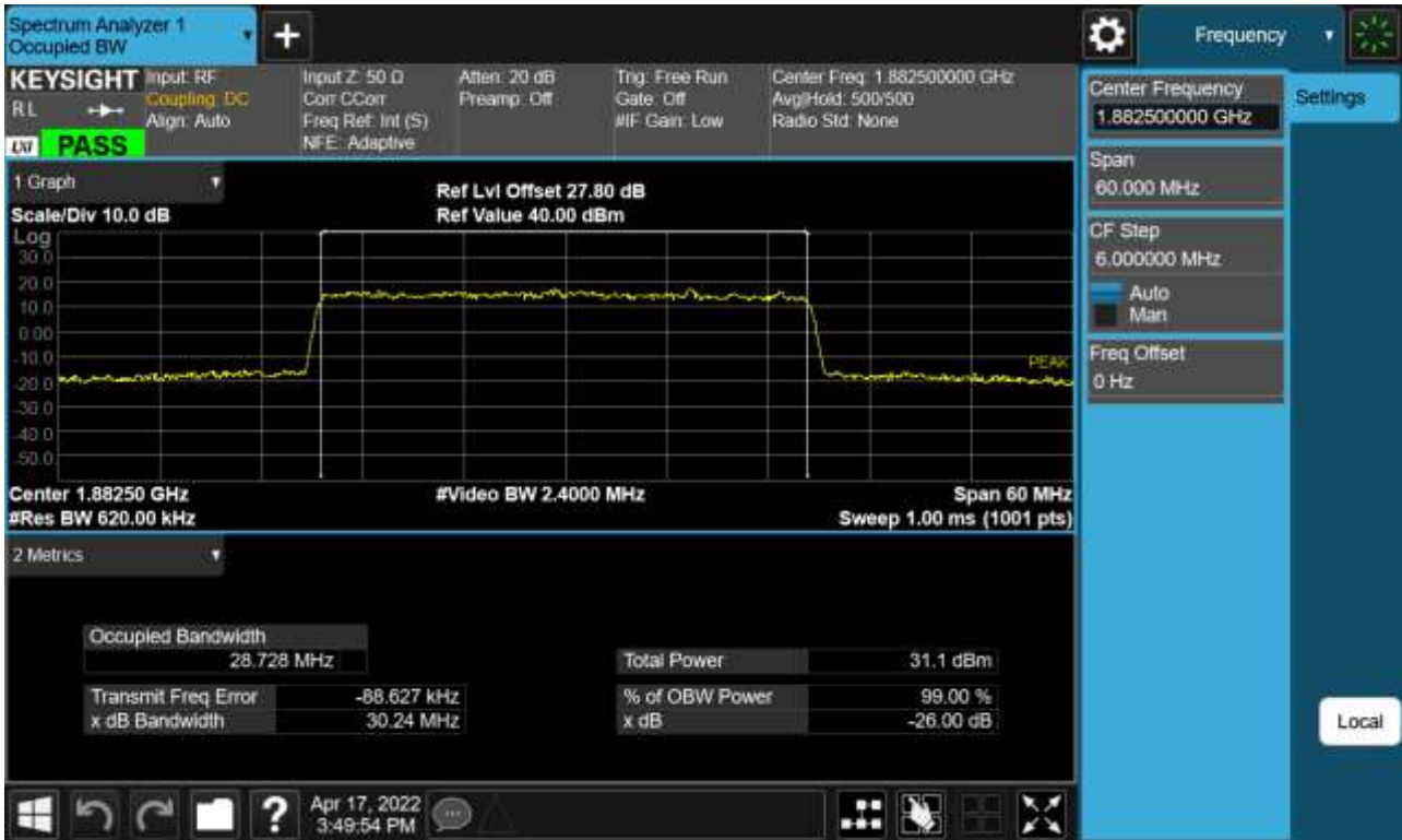
Sub6 n25. Occupied Bandwidth Plot (30 M BW Ch.376500 QPSK_ Full RB_0 )
