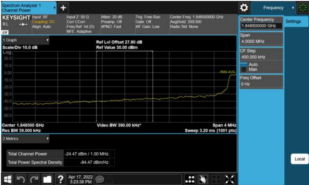
Sub6 n25(2). Lower Extended Band Edge Plot (15 M BW Ch.371500 BPSK_RB75_0) -2
