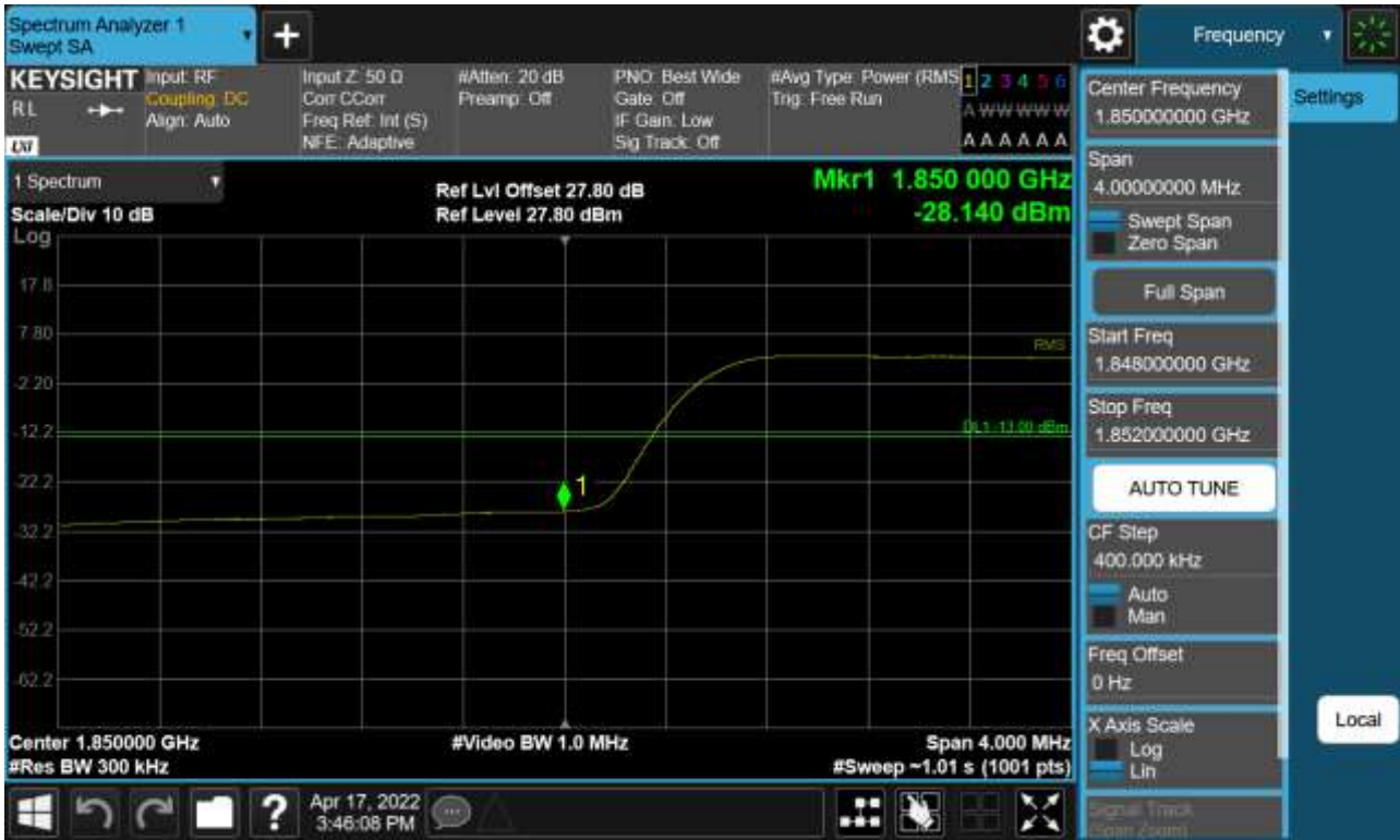
Sub6 n25. Lower Band Edge Plot (30 M BW Ch.373000 BPSK_RB160_Offset 0) -1
