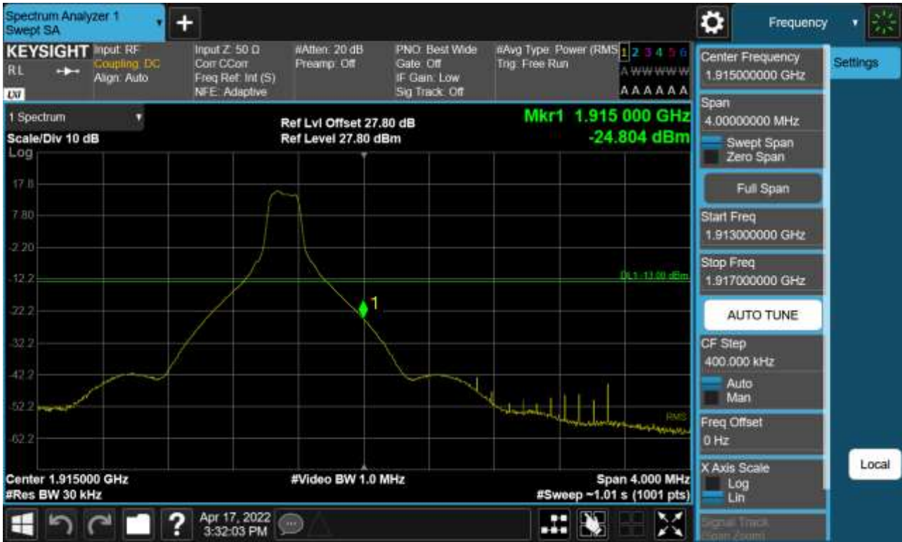
Sub6 n25(2). Upper Band Edge Plot (15 M BW Ch.381500 BPSK_RB1_Offset 74)
