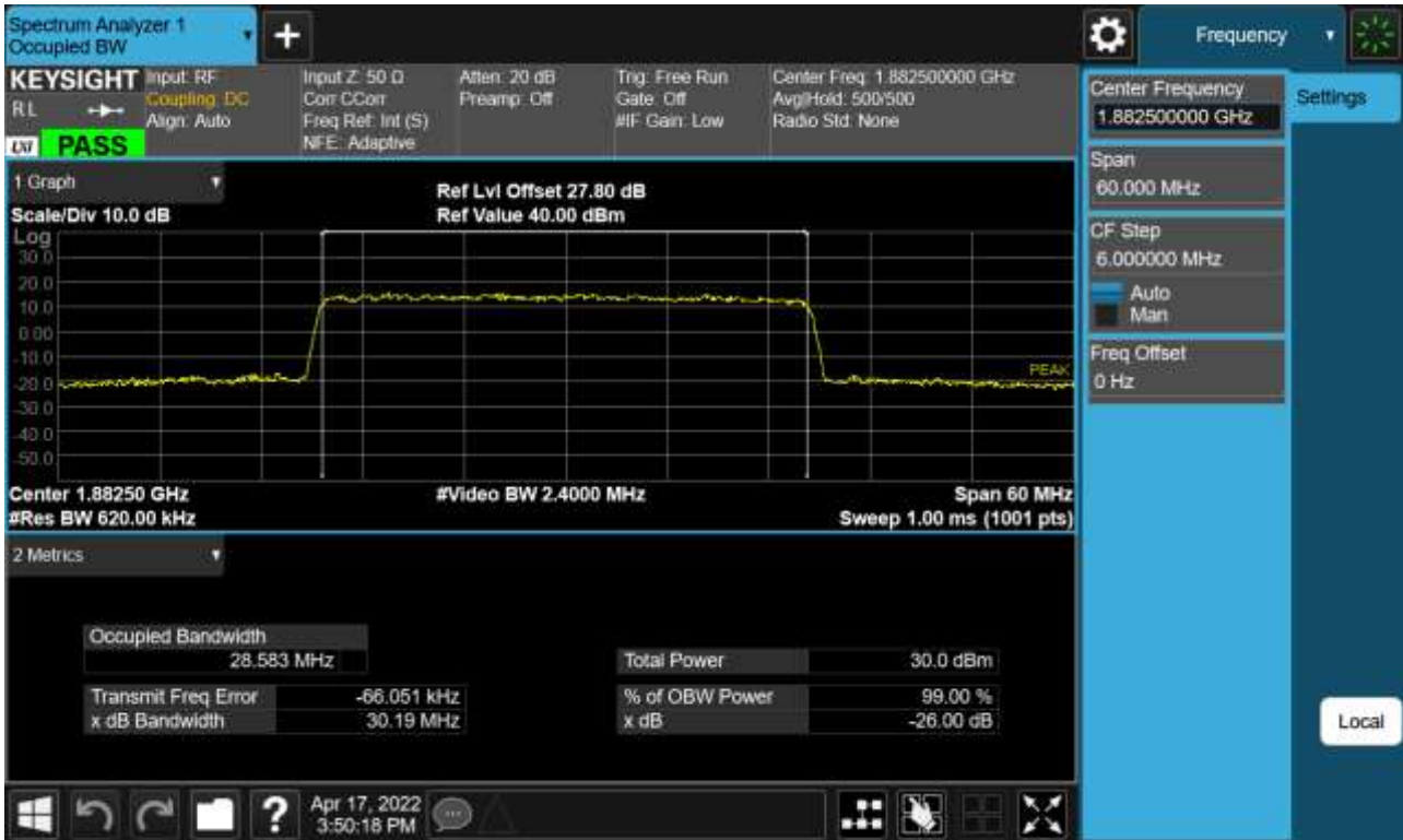
Sub6 n25. Occupied Bandwidth Plot (30 M BW Ch.376500 16QAM _ Full RB _0)
