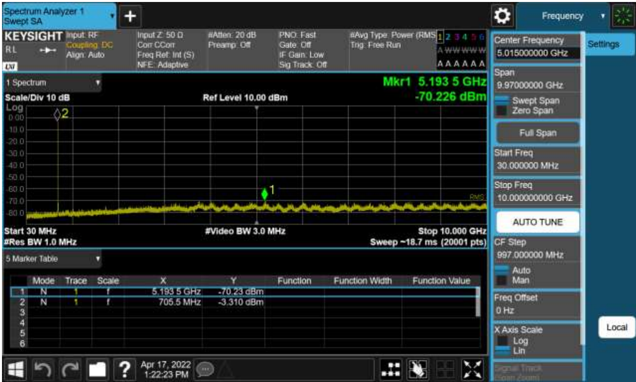
Sub6 n12. Conducted Spurious Plot _ (141500ch_5MHz_BPSK_RB 1_1)
