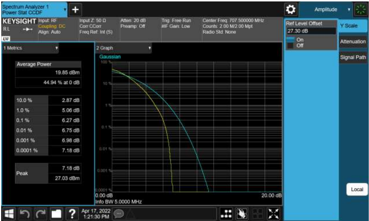
Sub6 n12. PAR Plot (5M BW Ch.141500 256QAM_RB25_0)
