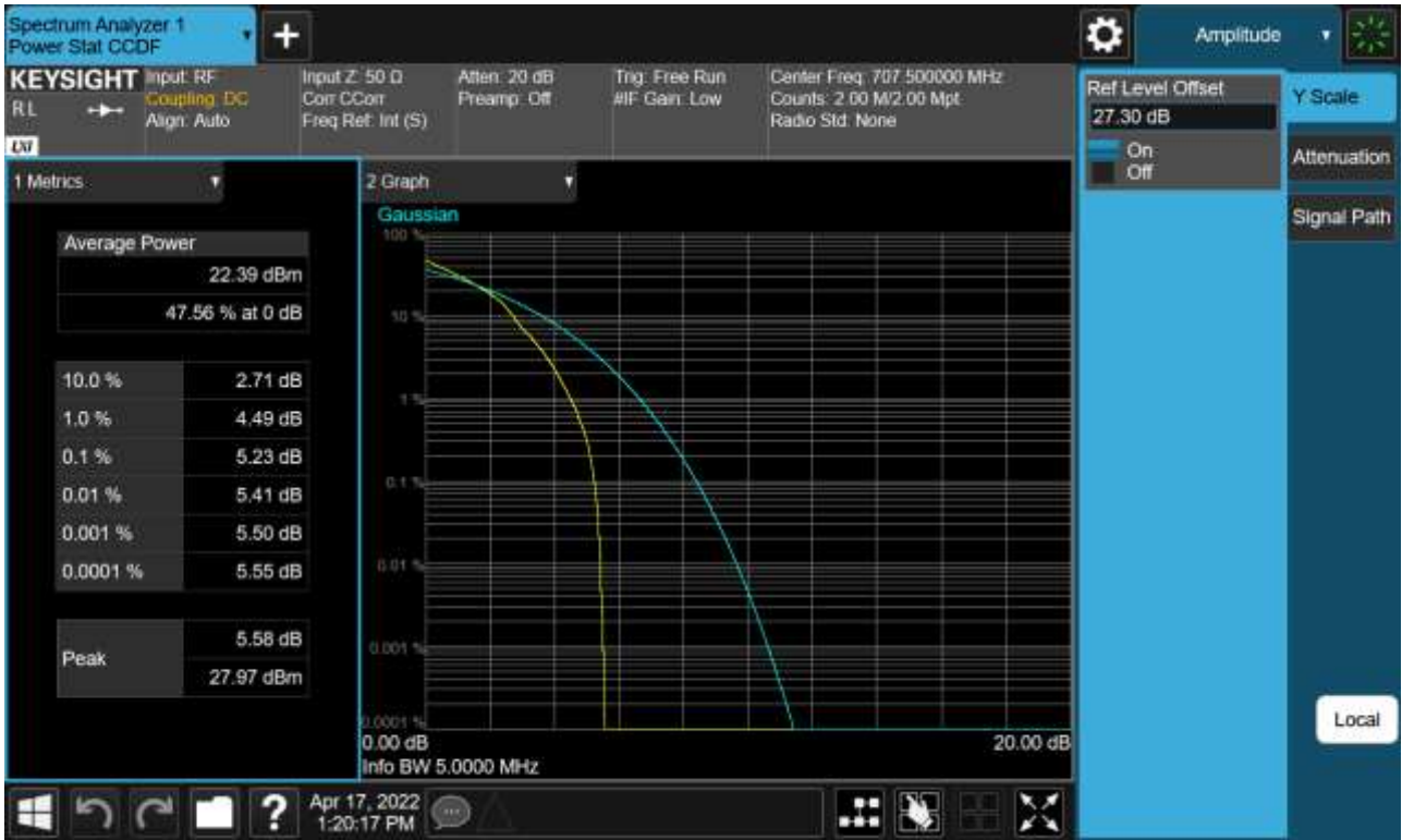
Sub6 n12. PAR Plot (5M BW Ch.141500 16QAM_RB25_0)
