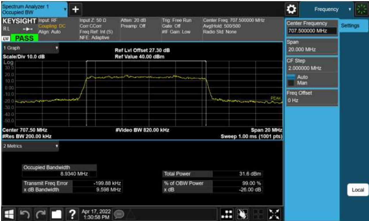
Sub6 n12. Occupied Bandwidth Plot (10M BW Ch.141500 QPSK_RB50_0)
