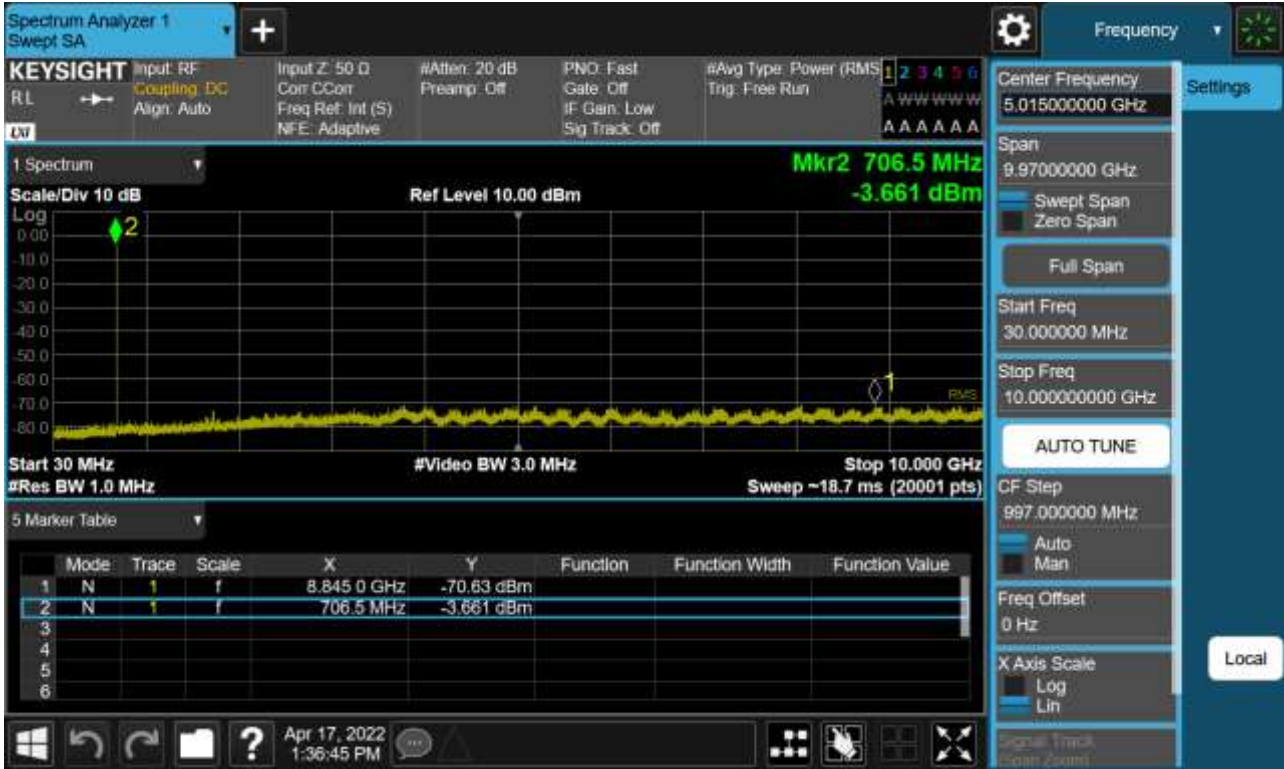
Sub6 n12. Conducted Spurious Plot _ (142200ch_10MHz_BPSK_RB 1_1)
