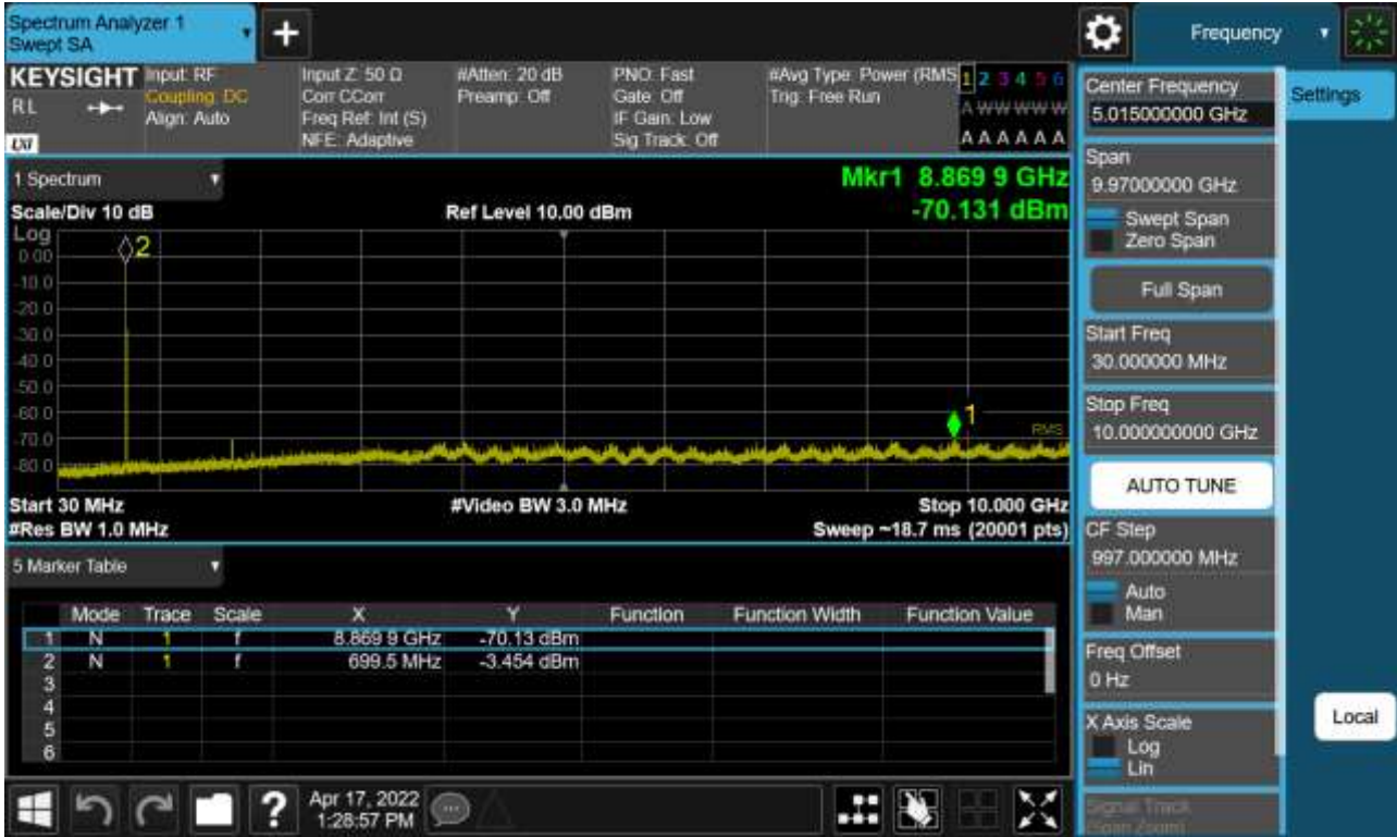
Sub6 n12. Conducted Spurious Plot _ (140800ch_10MHz_BPSK_RB 1_1)
