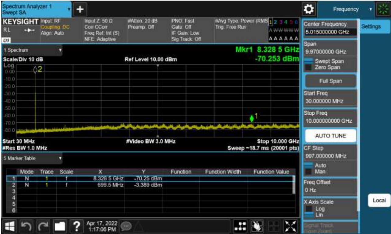
Sub6 n12. Conducted Spurious Plot _ (140300ch_5MHz_BPSK_RB 1_1)
