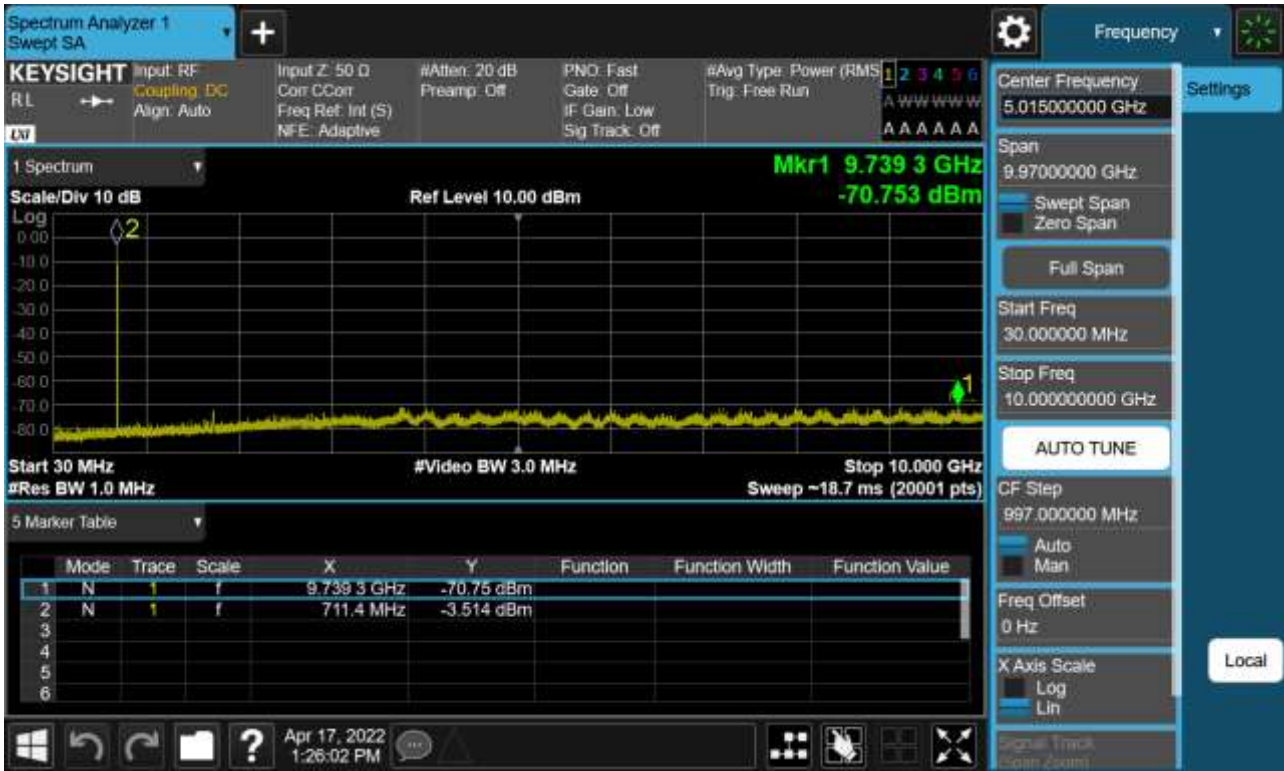
Sub6 n12. Conducted Spurious Plot _ (142700ch_5MHz_BPSK_RB 1_1)
