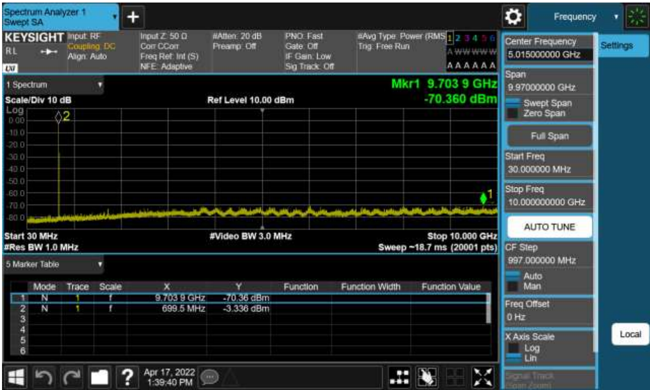
Sub6 n12. Conducted Spurious Plot _ (141300ch_15MHz_BPSK_RB 1_1)
