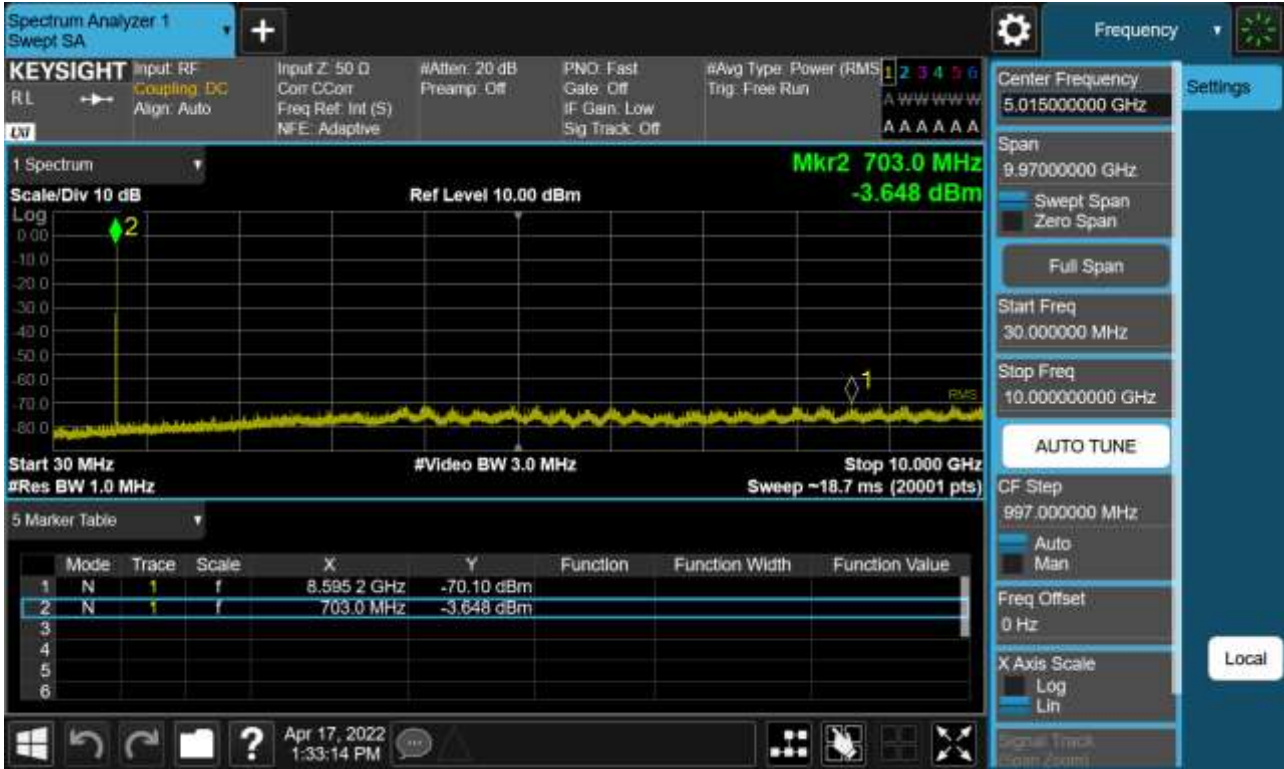
Sub6 n12. Conducted Spurious Plot _ (141500ch_10MHz_BPSK_RB 1_1)
