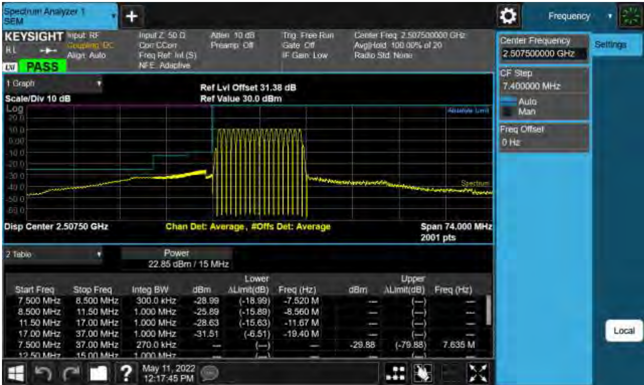
Low Channel Edge Plot (15 MHz Ch.39765 QPSK_RB75_Offset 0)-1 (POWER CLASS 3)
