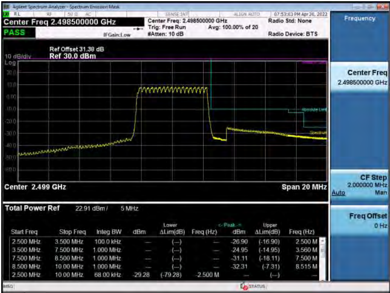
Low Channel Edge Plot (5 MHz Ch.39675 QPSK_RB25_Offset 0)-2 (POWER CLASS 2)
