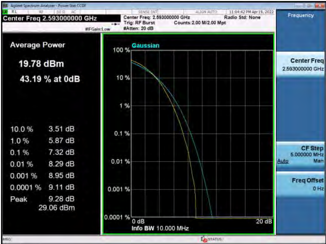
PAR Plot (10M BW_Ch.40620_64QAM_RB50_0) (POWER CLASS 3)
