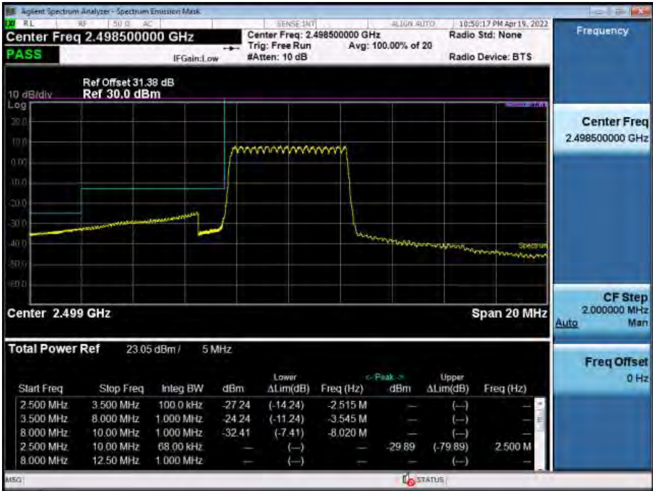
Low Channel Edge Plot (5 MHz Ch.39675 QPSK_RB25_Offset 0)-1 (POWER CLASS 3)
