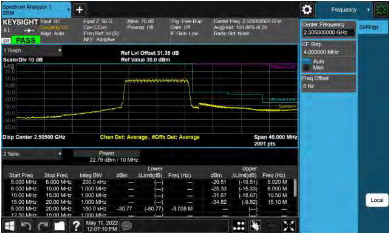
Low Channel Edge Plot (10 MHz Ch.39740 QPSK_RB50_Offset 0)-2 (POWER CLASS 3)
