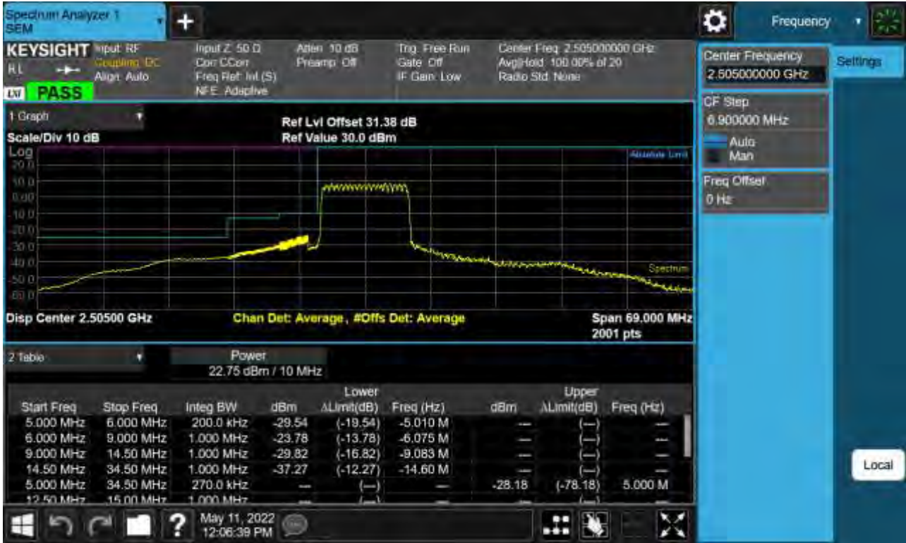
Low Channel Edge Plot (10 MHz Ch.39740 QPSK_RB50_Offset 0)-1 (POWER CLASS 3)
