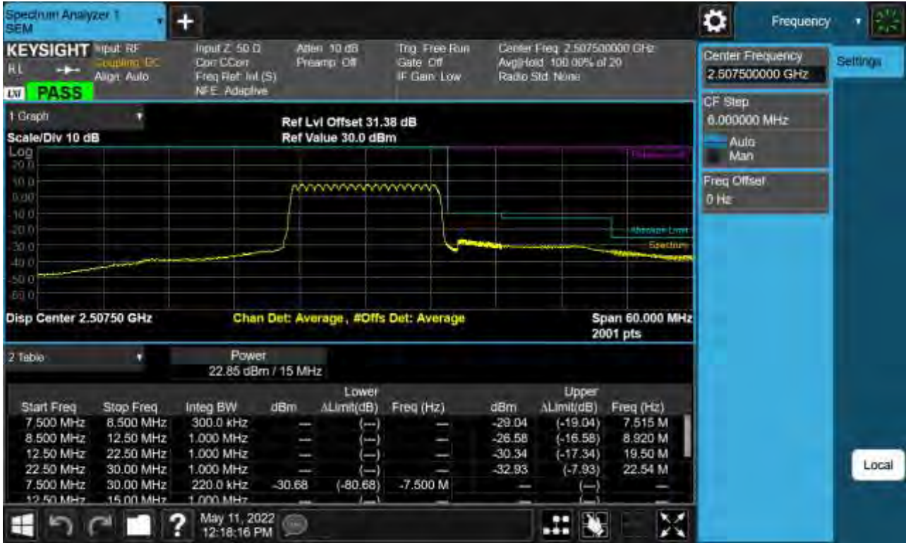
Low Channel Edge Plot (15 MHz Ch.39765 QPSK_RB75_Offset 0)-2 (POWER CLASS 3)
