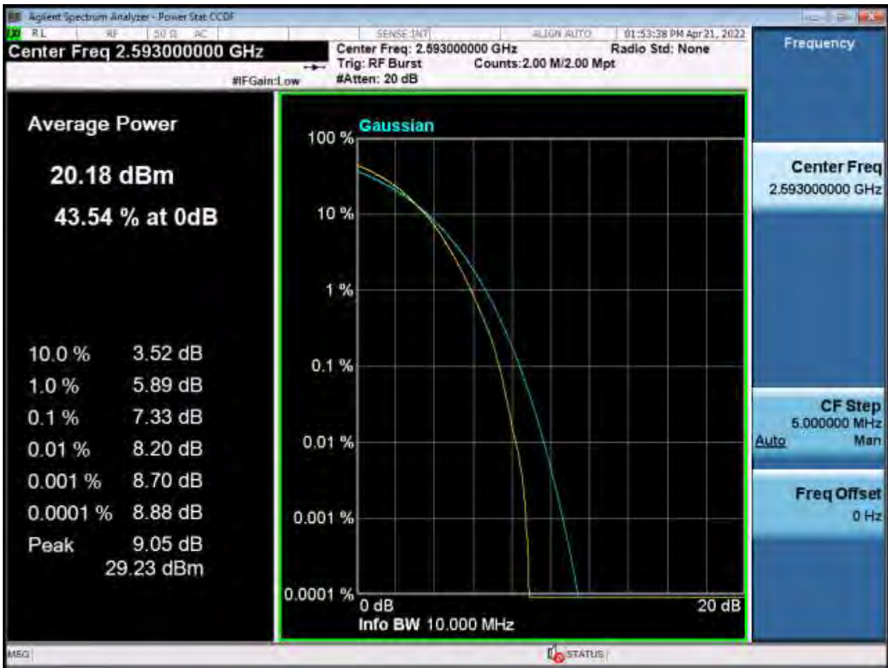
PAR Plot (10M BW_Ch.40620_256QAM_RB50_0) (POWER CLASS 2)
