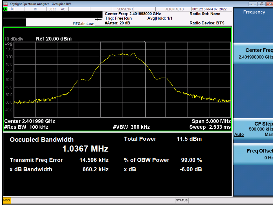
6 dB Bandwidth plot (Low-CH 0)
