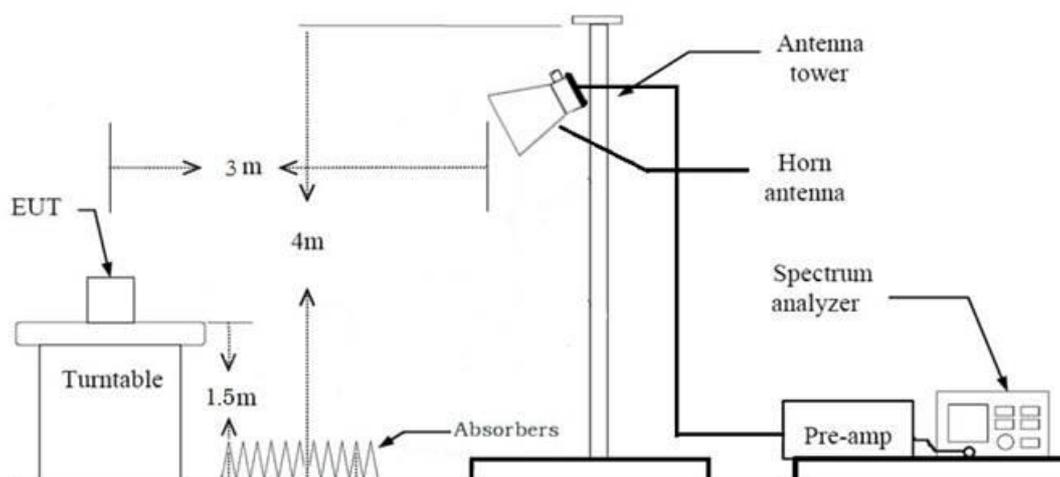
**Test Procedure of Radiated spurious emissions(Below30 MHz)**
