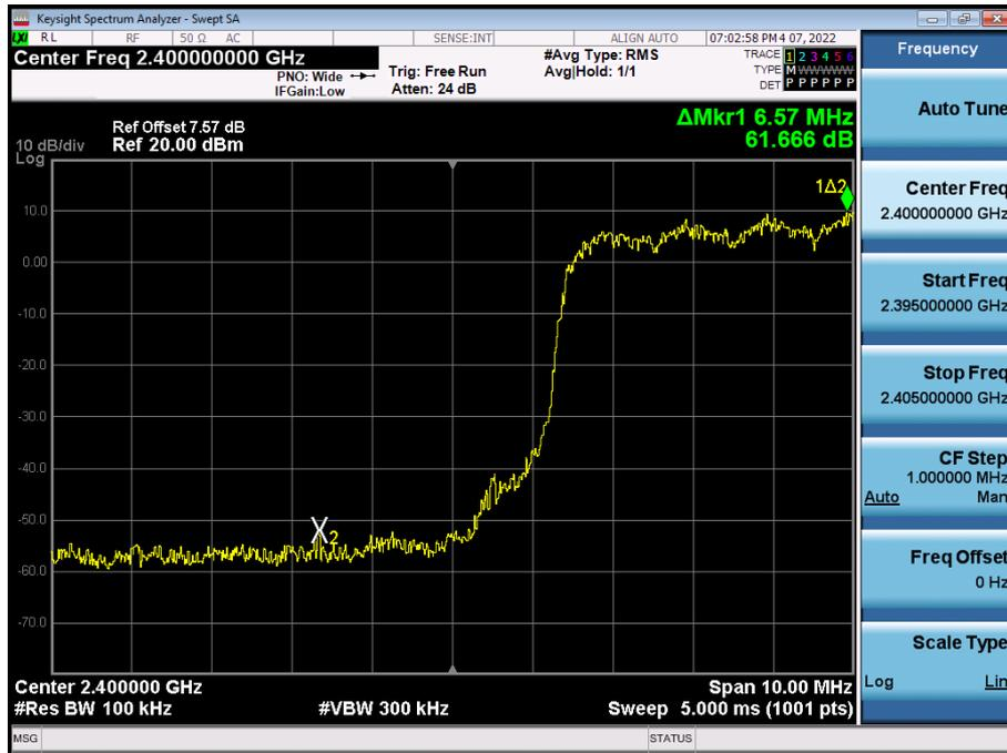
Test Plots with hopping (8DPSK)
