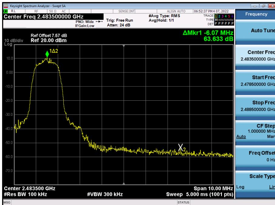
Test Plots with hopping (GFSK)
