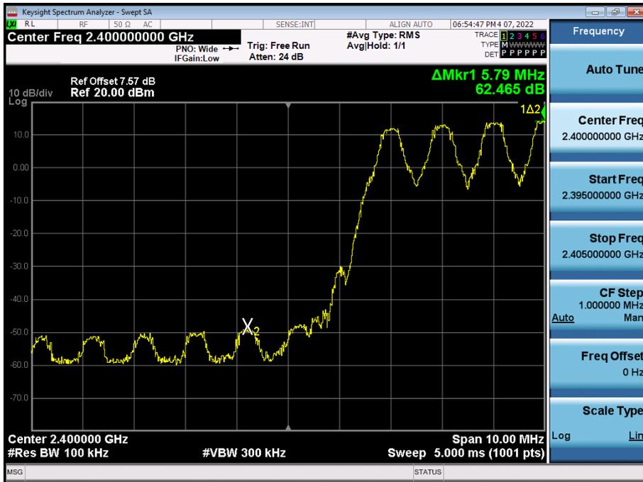
Test Plots with hopping (GFSK)
