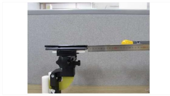
Edge 3:15 cm (The distance between the DUT and the center of the probe is 15 cm.)
