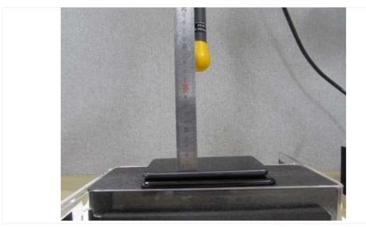
**Bottom : 15 cm** (The distance between the DUT and the center of the probe is 15 cm.)
