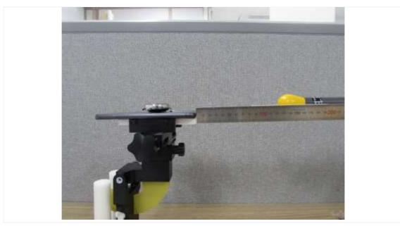
Edge 1:15 cm (The distance between the DUT and the center of the probe is 15 cm.)
