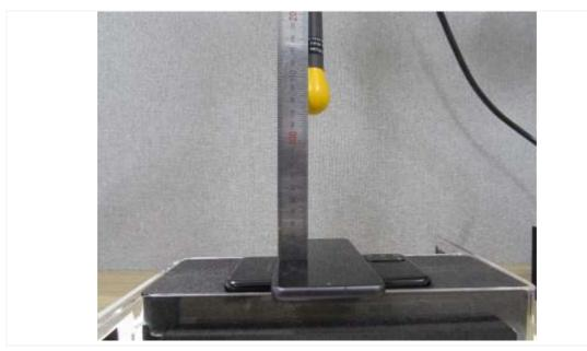
**Bottom : 15 cm** (The distance between the DUT and the center of the probe is 15 cm.)
