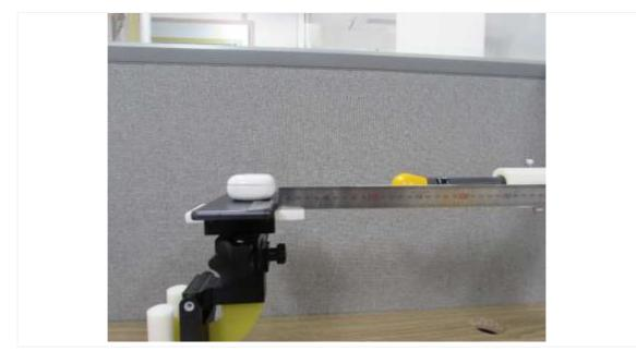
Edge 4:15 cm (The distance between the DUT and the center of the probe is 15 cm.)
