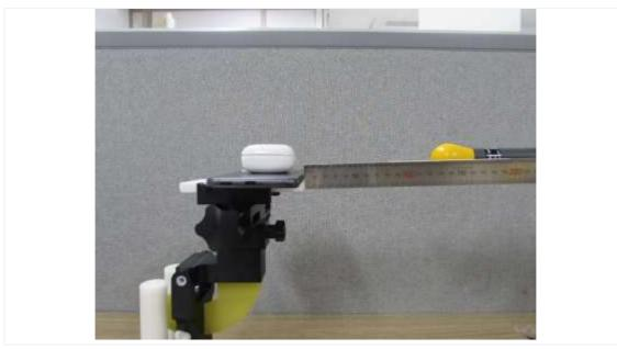
Edge 2: 15 cm (The distance between the DUT and the center of the probe is 15 cm.)
