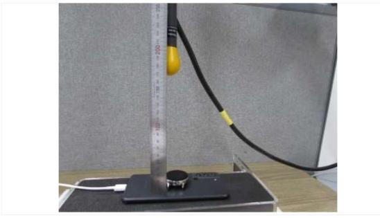
**Top + TA : 20 cm** (The distance between the DUT and the center of the probe is 20 cm.)
