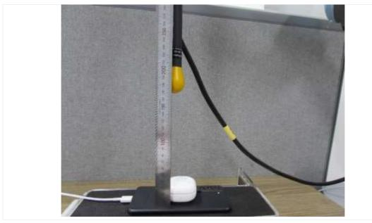
**Top + TA : 20 cm** (The distance between the DUT and the center of the probe is 20 cm.)
