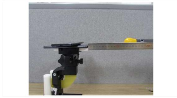
Edge 1:15 cm (The distance between the DUT and the center of the probe is 15 cm.)
