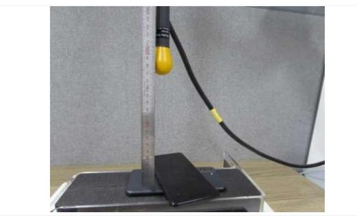
**Top : 20 cm** (The distance between the DUT and the center of the probe is 20 cm.)
