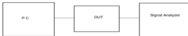
Power Measurement Setup – NR TDD
