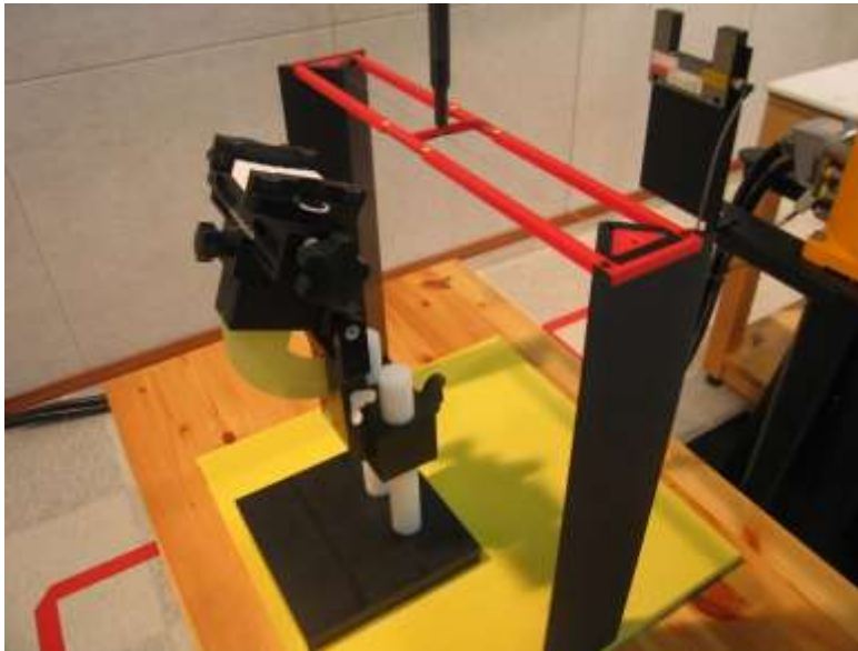
Figure 2. HAC Phantom & Device Holder
