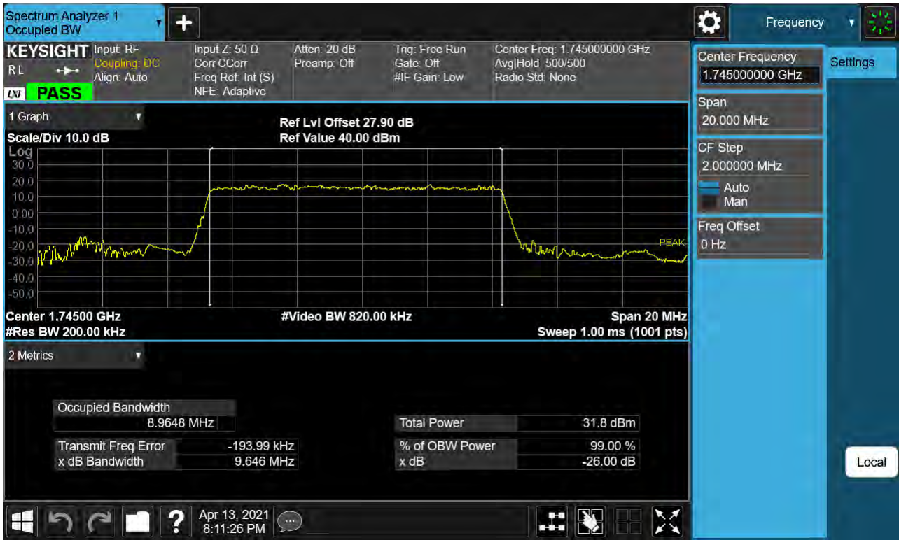
Sub6 n66. Occupied Bandwidth Plot (10M BW Ch.349000 BPSK RB 50)
