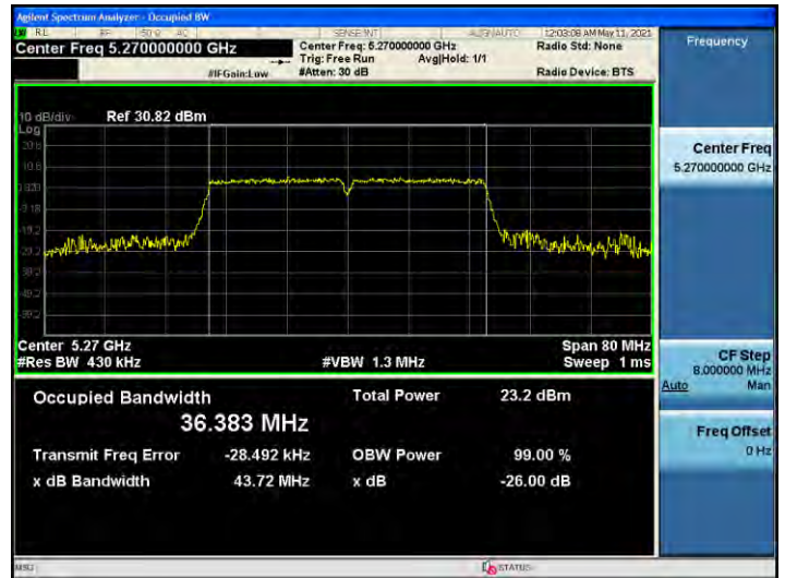
802.11n_HT40 UNII 3 BAND 26dB Bandwidth (CH 151)
