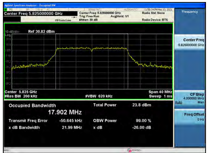
802.11n_HT20 UNII 3 BAND 26dB Bandwidth(CH 165)
