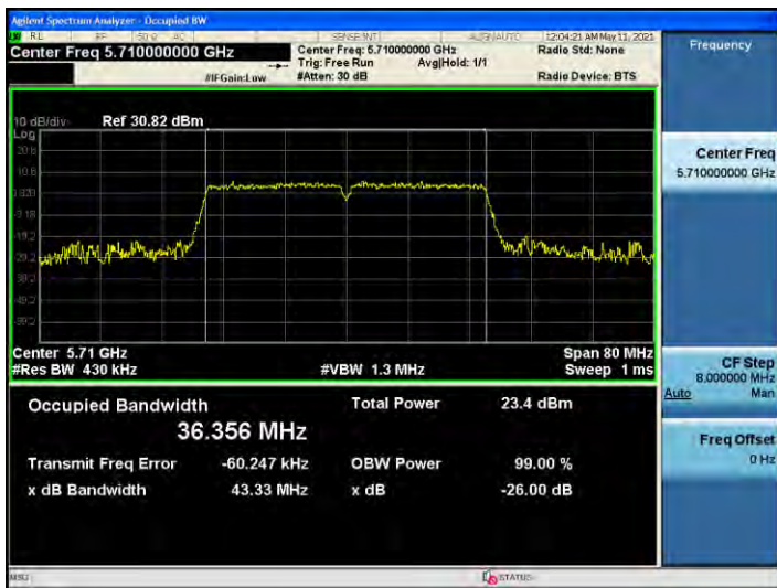
802.11n_HT40 UNII 2C BAND 26dB Bandwidth(CH 142)
