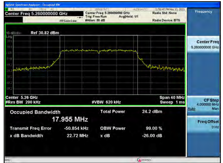
802.11ac_VHT20 UNII 3 BAND 26dB Bandwidth(CH 149)
