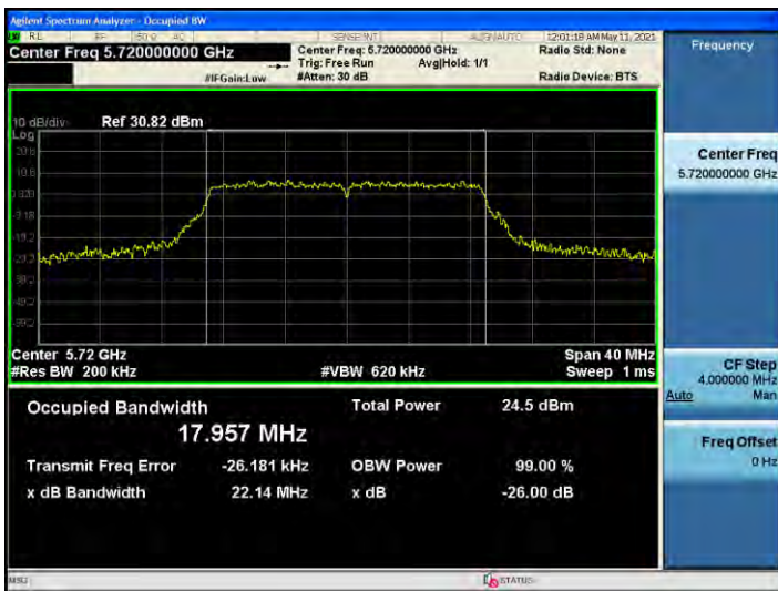
802.11ac_VHT20 UNII 2C BAND 26dB Bandwidth(CH 144)
