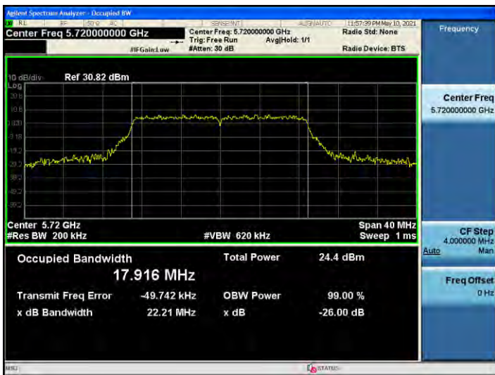
802.11n_HT20 UNII 2C BAND 26dB Bandwidth(CH 144)
