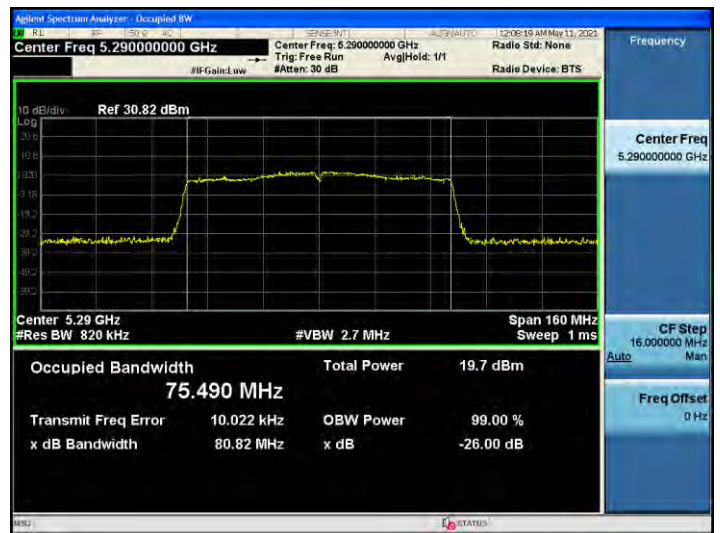
802.11ac_VHT80 UNII 3 BAND 26dB Bandwidth (CH 155)
