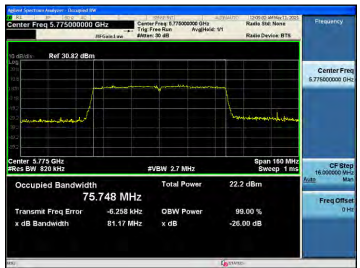
802.11ac_VHT80 UNII 3 BAND 26dB Bandwidth (CH 155)
