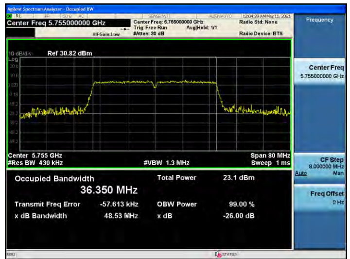
802.11n_HT40 UNII 3 BAND 26dB Bandwidth (CH 151)
