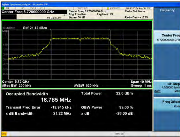
802.11a UNII 2C BAND 26 dB Bandwidth (CH 144)
