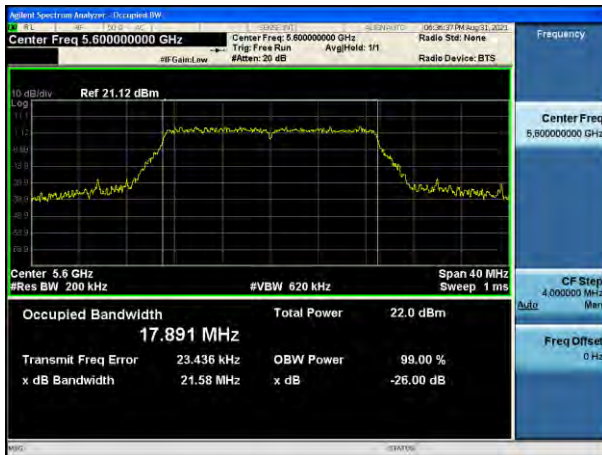
802.11n_HT20 UNII 2C BAND 26 dB Bandwidth(CH 120)
