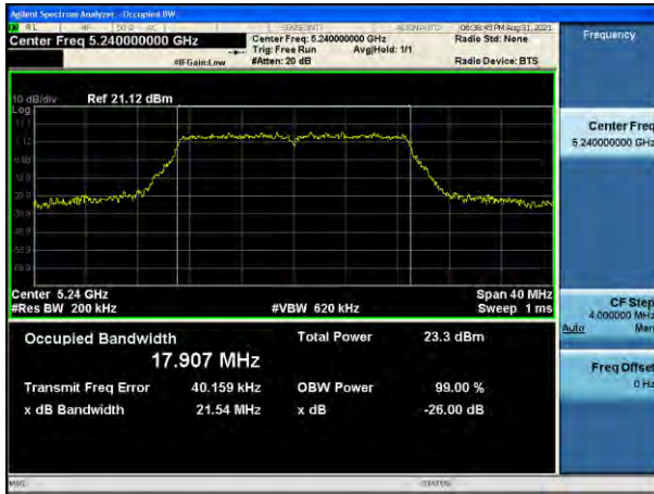
802.11ac_VHT20 UNII 2C BAND 26 dB Bandwidth(CH 144)
