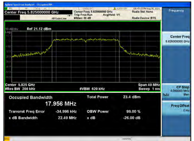
802.11n_HT20 UNII 3 BAND 26 dB Bandwidth(CH 165)
