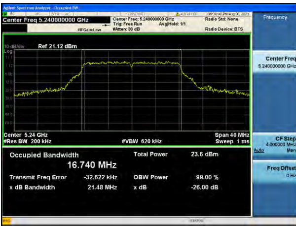
802.11a UNII 2C BAND 26 dB Bandwidth (CH 144)
