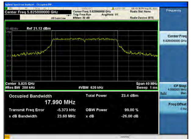
802.11ac_VHT20 UNII 3 BAND 26 dB Bandwidth(CH 165)
