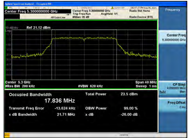
802.11ac_VHT20 UNII 3 BAND 26 dB Bandwidth(CH 165)
