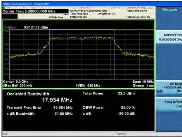
802.11n_HT20 UNII 2C BAND 26 dB Bandwidth(CH 120)
