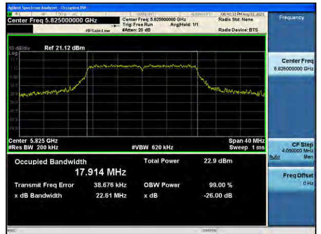
802.11ac_VHT20 UNII 3 BAND 26 dB Bandwidth(CH 165)
