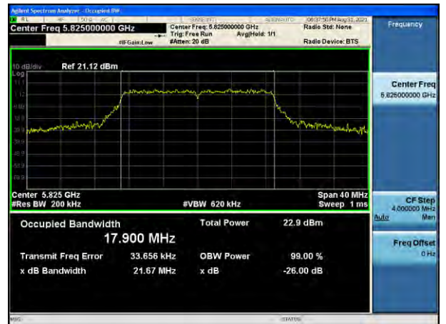
802.11n_HT20 UNII 3 BAND 26 dB Bandwidth(CH 165)
