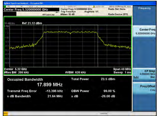
802.11n_HT20 UNII 3 BAND 26 dB Bandwidth(CH 165)
