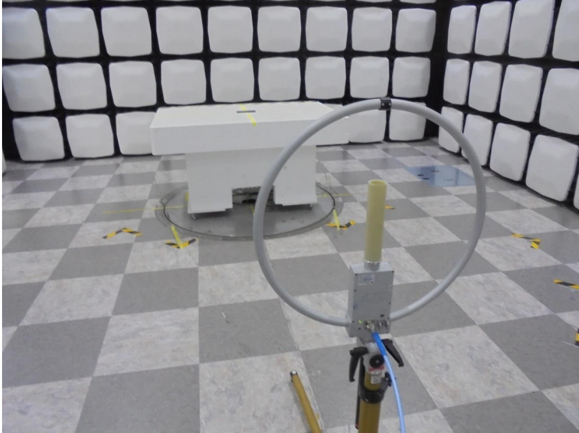
NFC Radiated Test Setup Photo for below 30 MHz:
