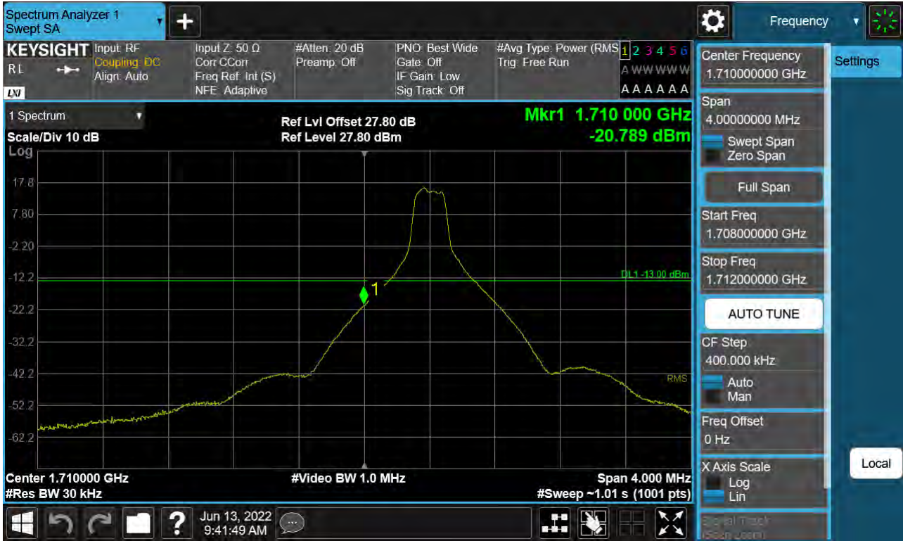
Sub6 n66. Lower Band Edge Plot (10 M BW Ch.343000 BPSK RB 1, Offset 0) -1
