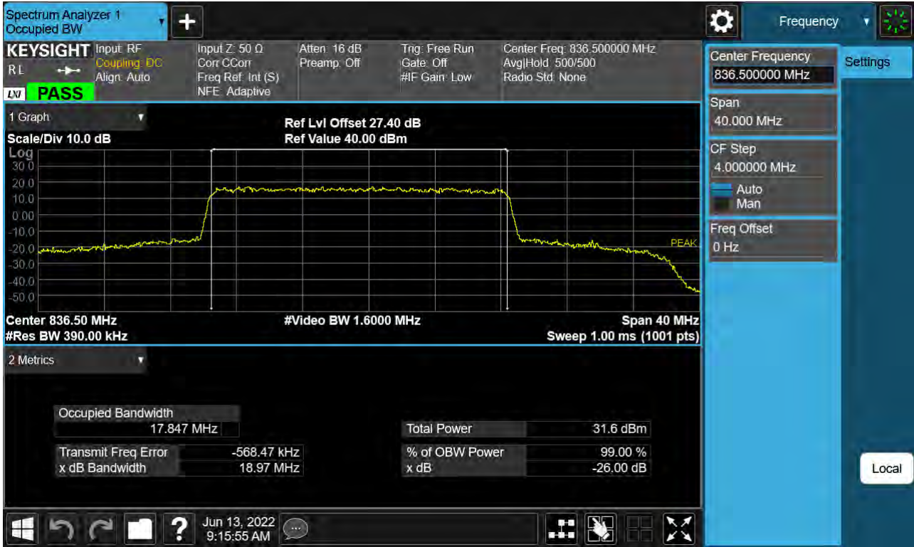
Sub6 n5. Occupied Bandwidth Plot (20 M BW Ch.167300 QPSK_ Full RB _0)
