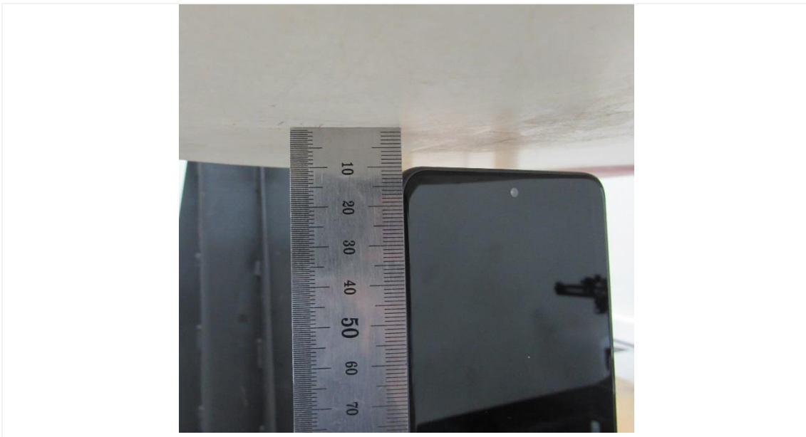
Distance of 10 mm from the EUT
