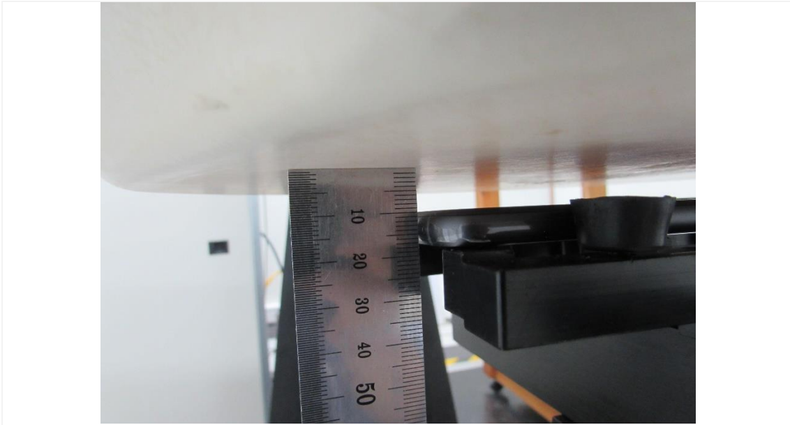
Distance of 10 mm from the EUT
