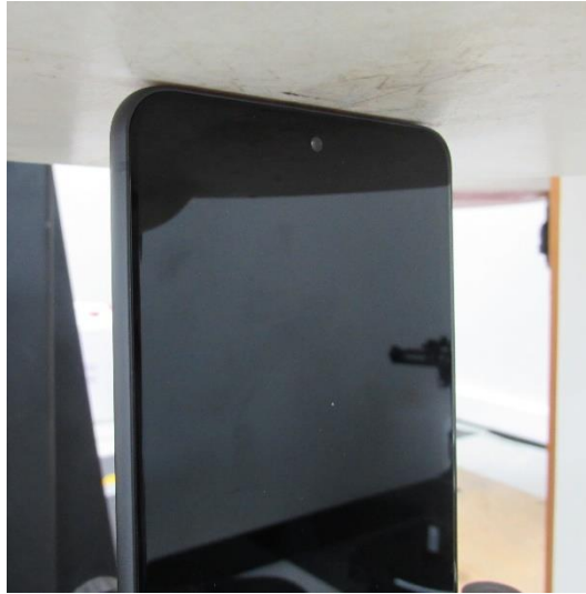
Distance of 0 mm from the EUT
