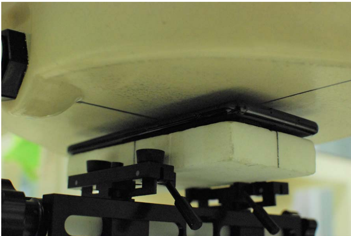
SAR Test Setup Photo 10 – Front Side at 6 mm
