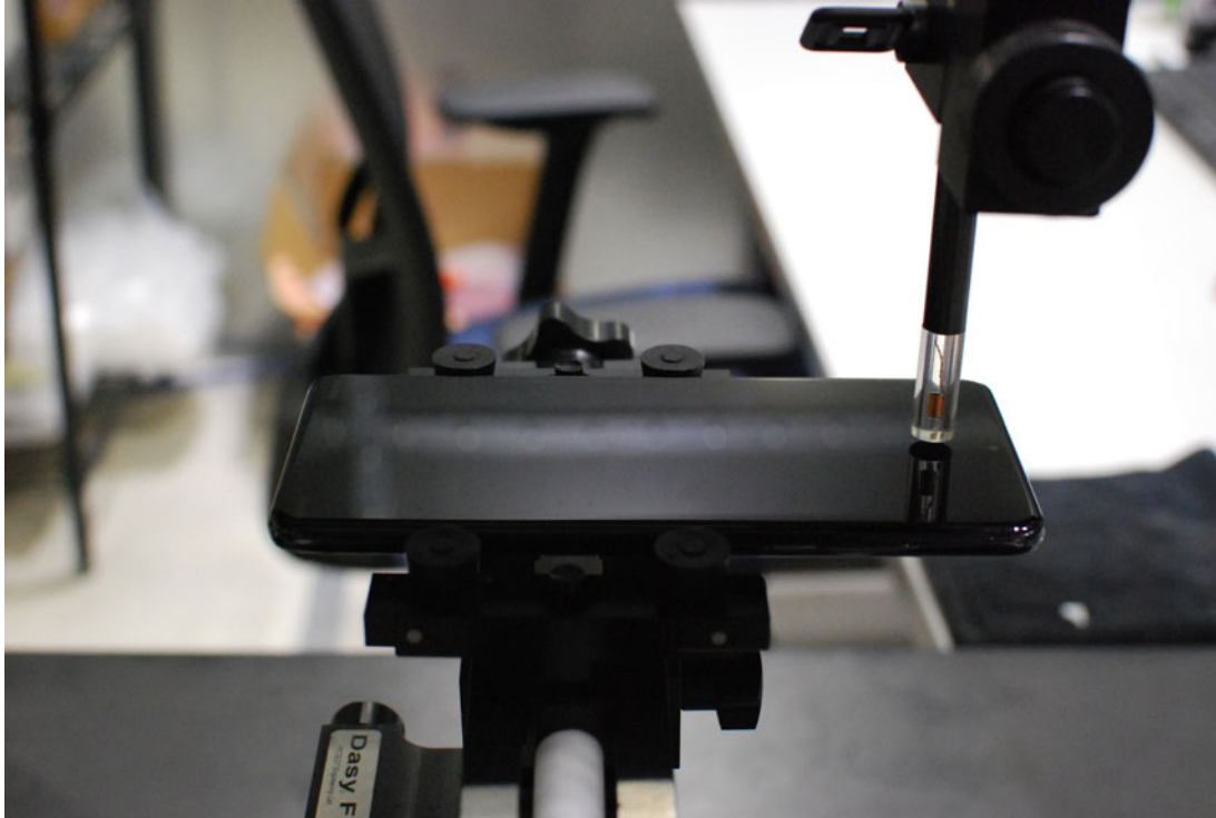
Figure 16-1 Test Setup for Wireless Device
