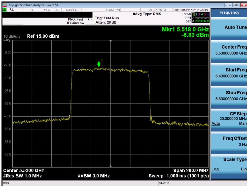
Plot 7-262. Power Spectral Density Plot MIMO ANT2 (80MHz BW 802.11ax – Full Tones (UNII Band 2C) – Ch. 106)
