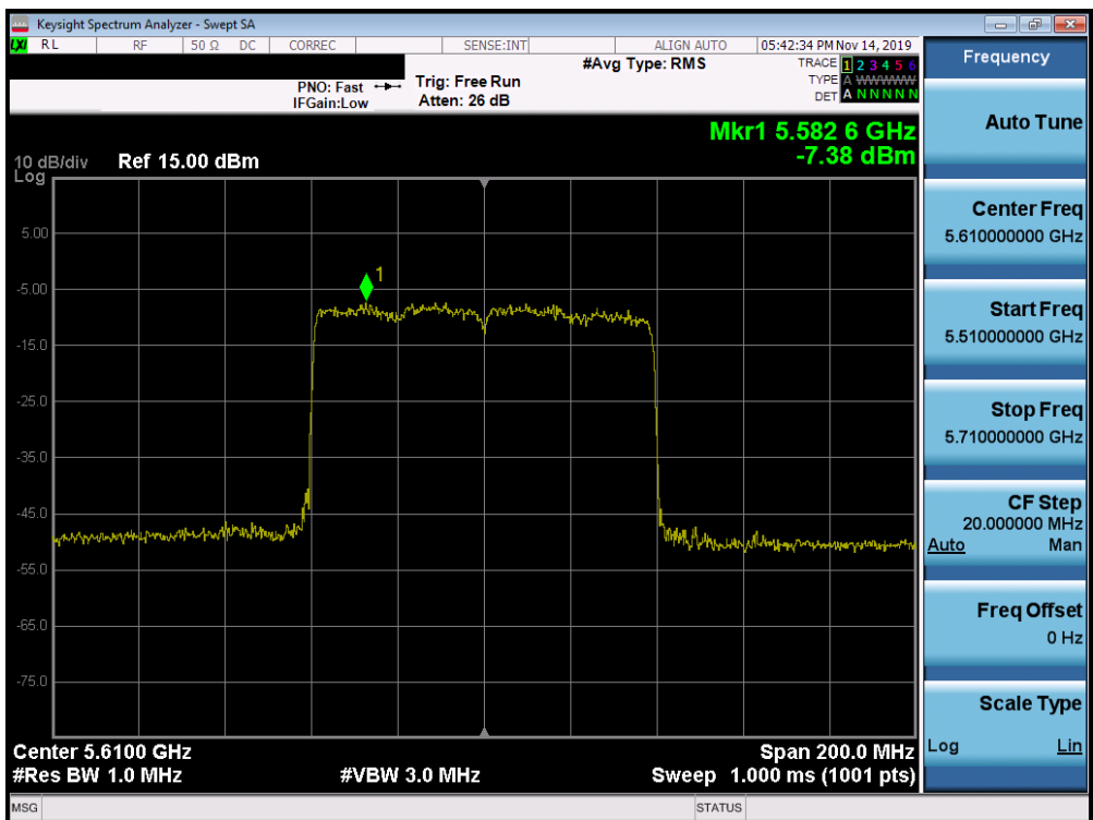
Plot 7-263. Power Spectral Density Plot MIMO ANT2 (80MHz BW 802.11ax - Full Tones (UNII Band 2C) - Ch. 122)
