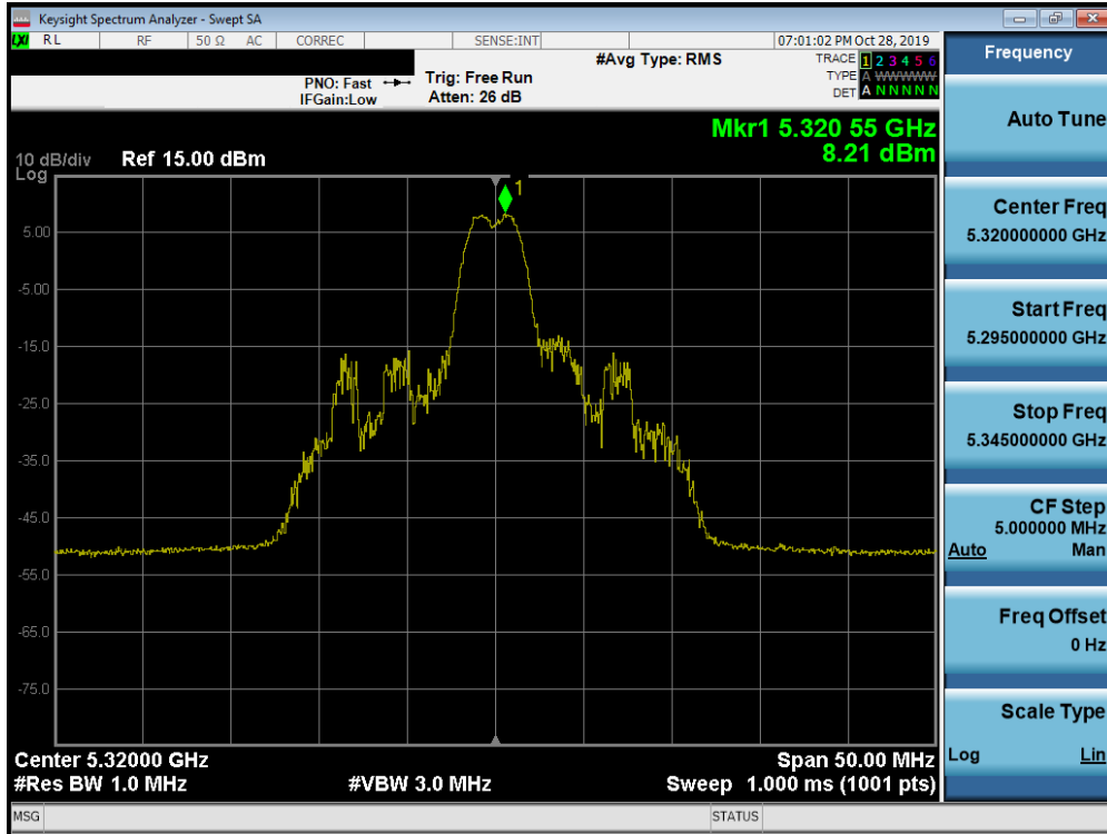
Plot 7-117. Power Spectral Density Plot SISO ANT2 (20MHz BW 802.11ax – 26 Tones (UNII Band 2A) – Ch. 64)
