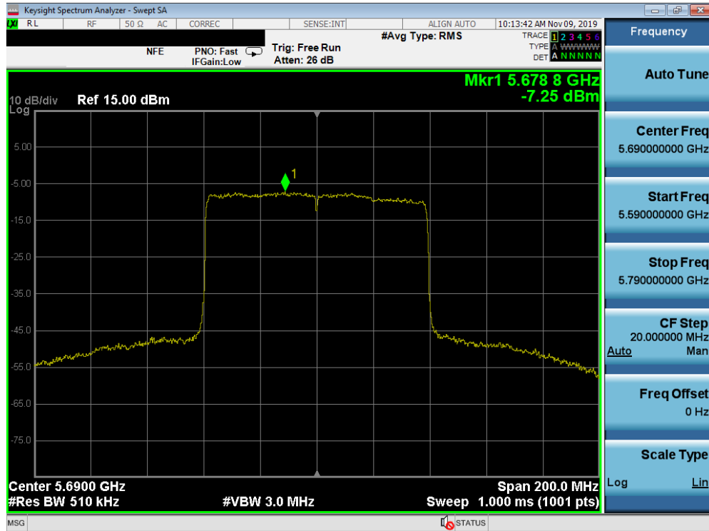
Plot 7-156. Power Spectral Density Plot SISO ANT2 (80MHz BW 802.11ax – Full Tones (UNII Band 2C) – Ch. 138)
