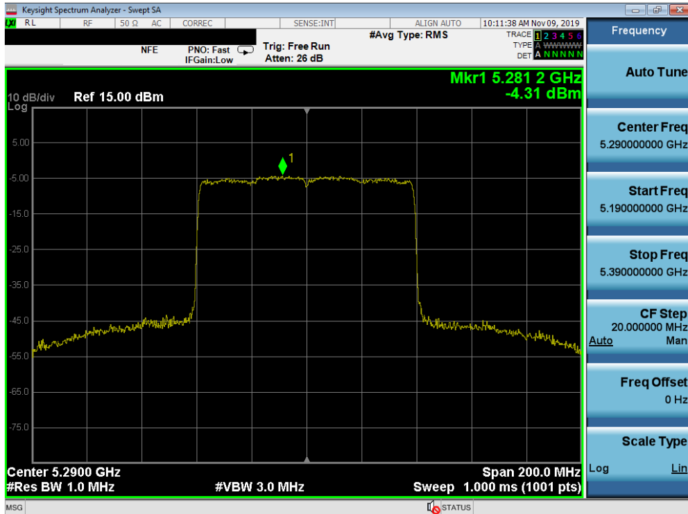
Plot 7-147. Power Spectral Density Plot SISO ANT2 (80MHz BW 802.11ax – Full Tones (UNII Band 2A) – Ch. 58)
