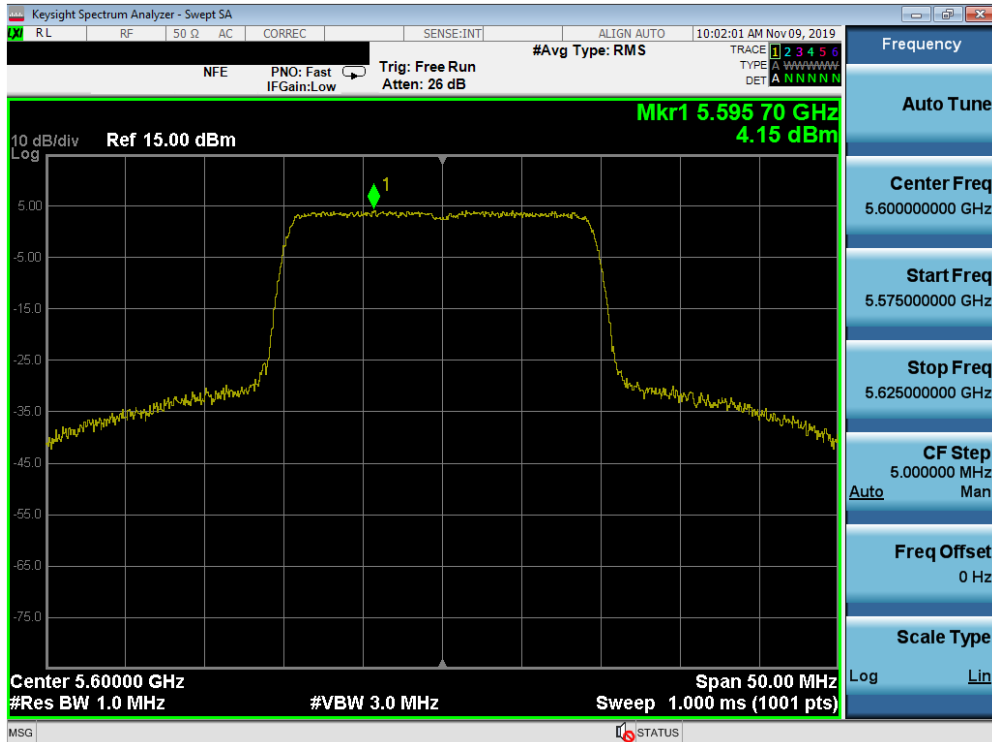
Plot 7-149. Power Spectral Density Plot SISO ANT2 (20MHz BW 802.11ax – Full Tones (UNII Band 2C) – Ch. 120)
