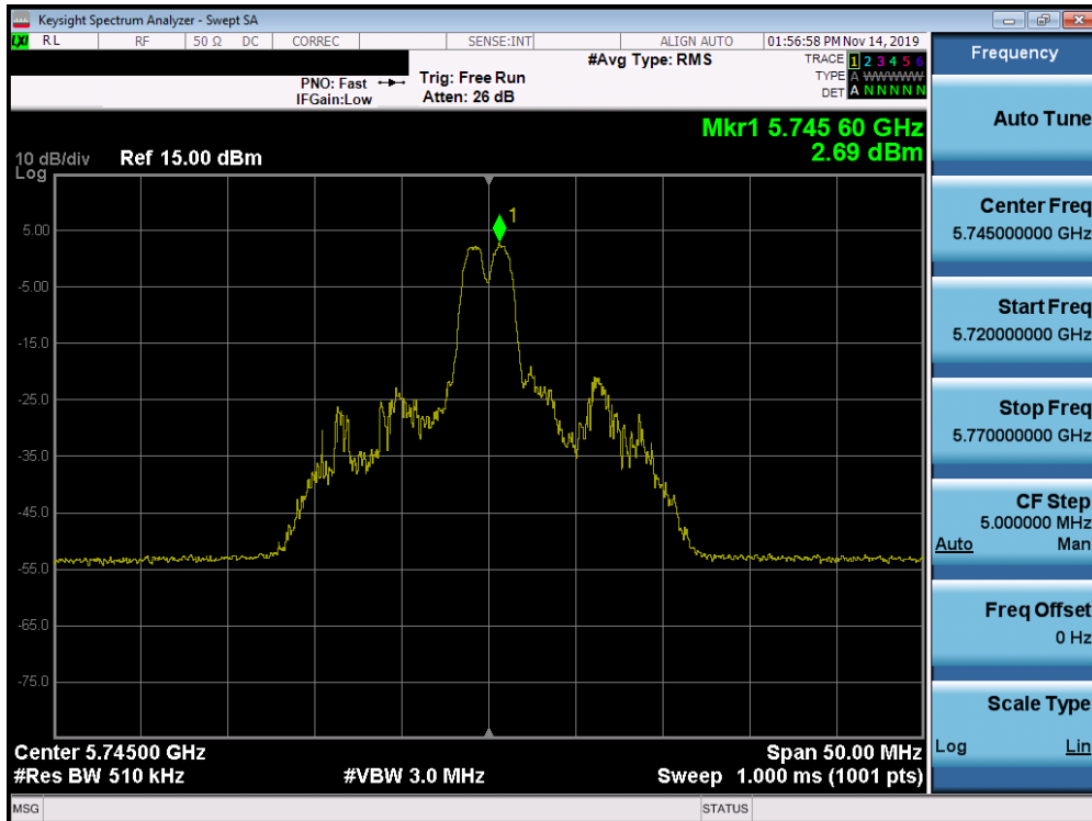
Plot 7-184. Power Spectral Density Plot MIMO ANT1 (20MHz BW 802.11ax – 26 Tones (UNII Band 3) – Ch. 149)
