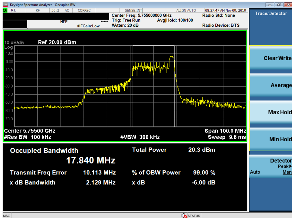
Plot 7-46. 6dB Bandwidth Plot SISO ANT1 (40MHz BW 802.11ax – 26 Tones (UNII Band 3) – Ch. 151)
