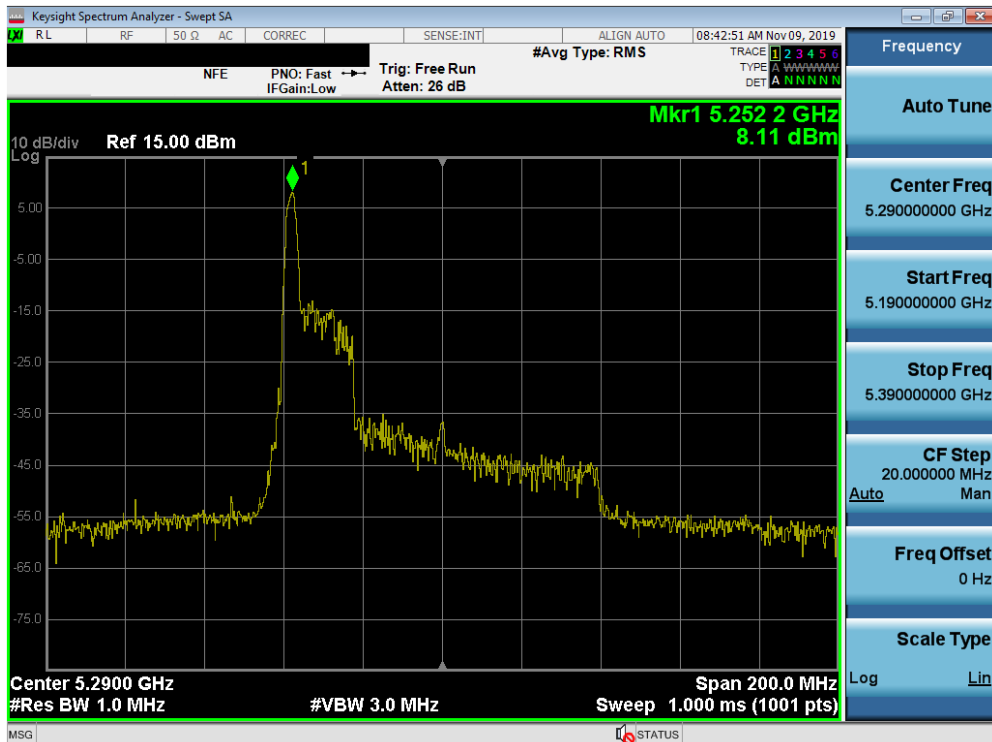
Plot 7-66. Power Spectral Density Plot SISO ANT1 (80MHz BW 802.11ax – 26 Tones (UNII Band 2A) – Ch. 58)
