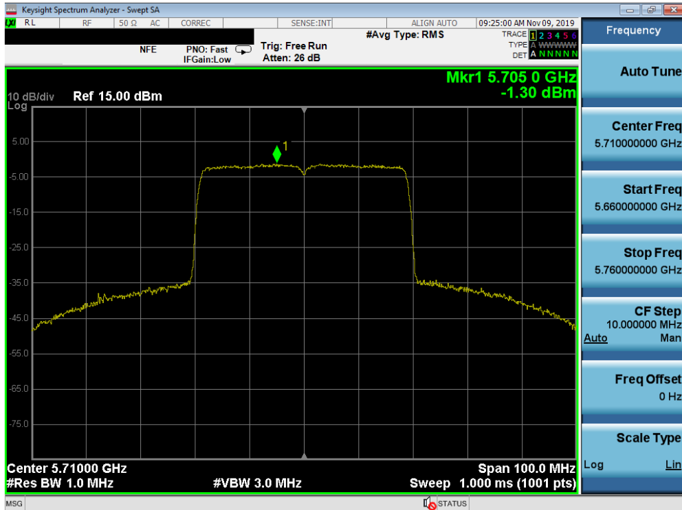
Plot 7-99. Power Spectral Density Plot SISO ANT1 (40MHz BW 802.11ax – Full Tones (UNII Band 2C) – Ch. 142)
