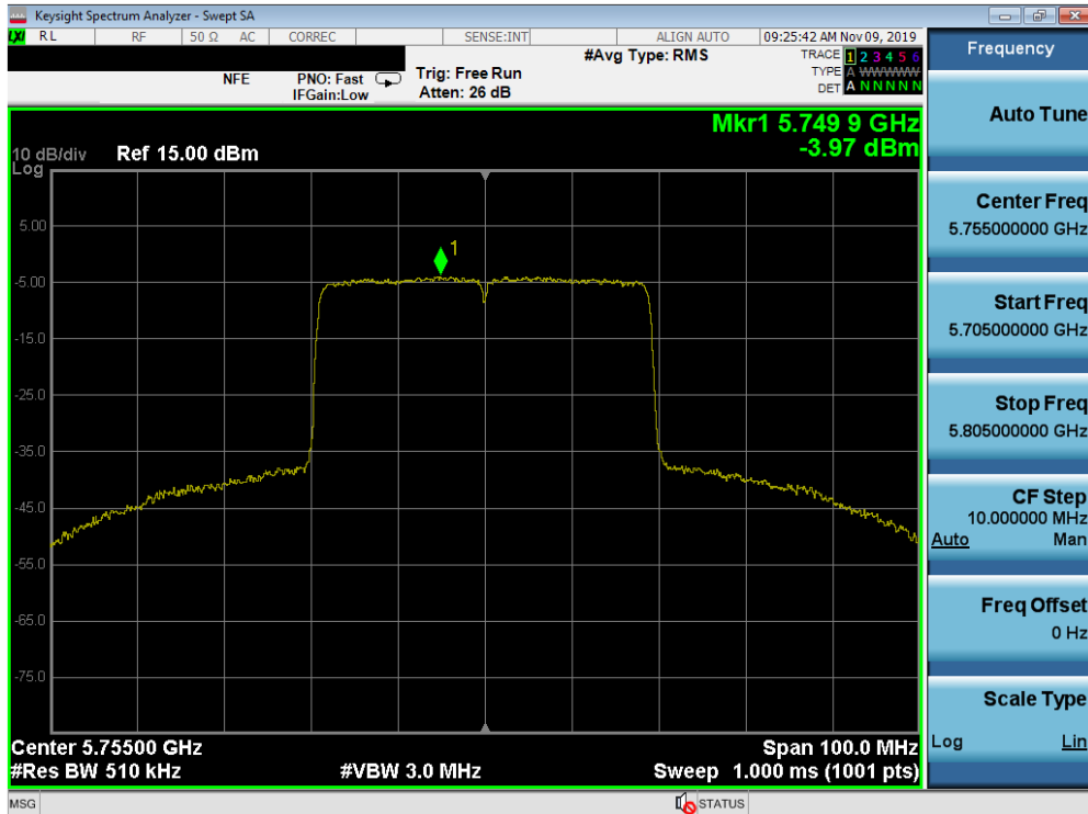
Plot 7-106. Power Spectral Density Plot SISO ANT1 (40MHz BW 802.11ax – Full Tones (UNII Band 3) – Ch. 151)
