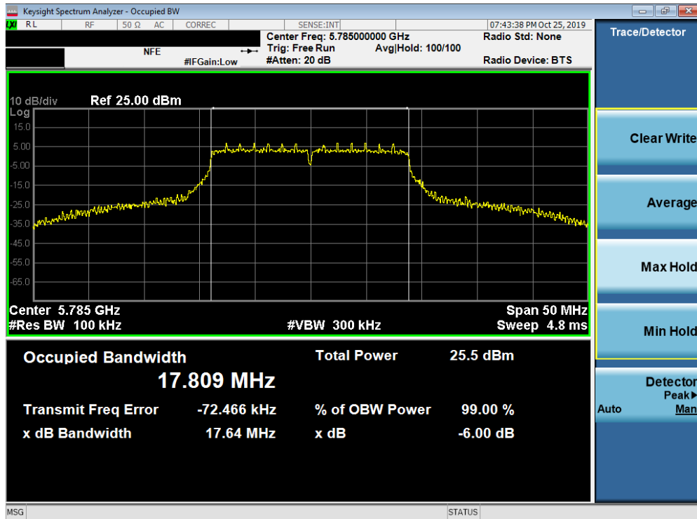
Plot 7-122. 6dB Bandwidth Plot SISO ANT2 (20MHz BW 802.11n (UNII Band 3) – Ch. 157)
