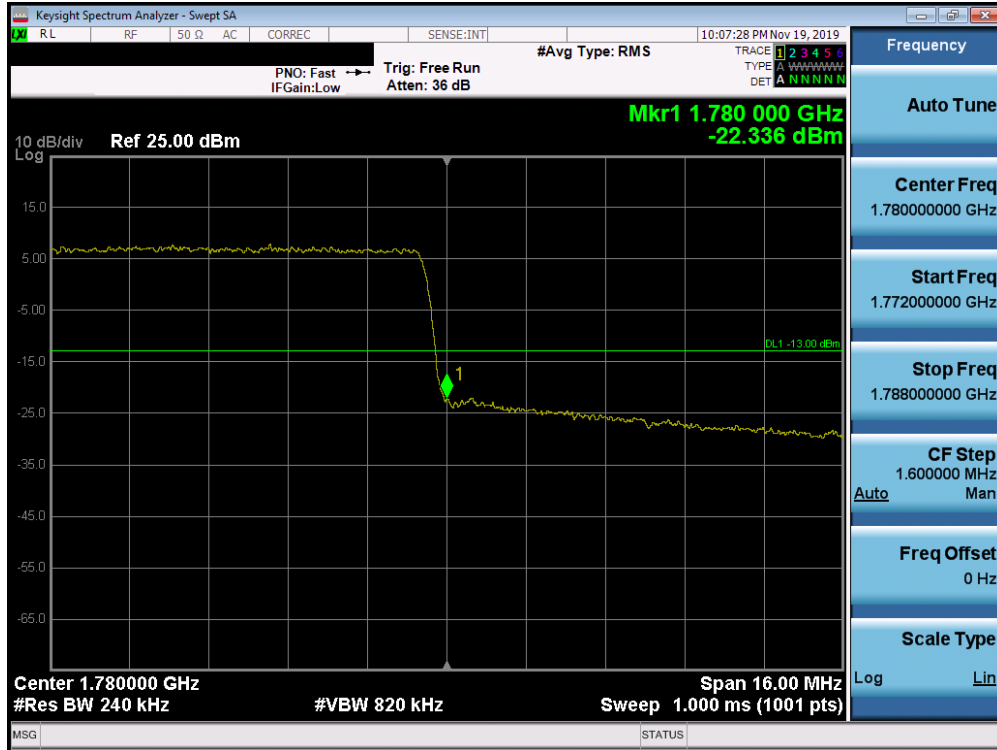
Plot 7-615. Upper Band Edge Plot (Band n66 - 20.0MHz CP-OFDM-QPSK - Full RB Configuration)
