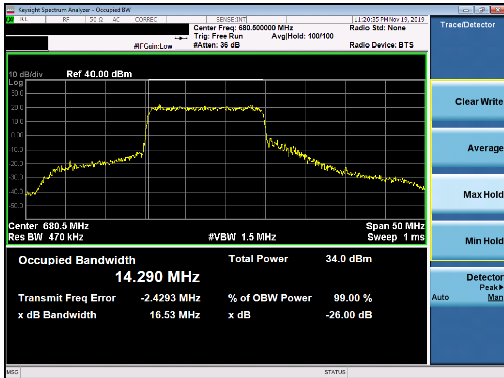
Plot 7-514. Occupied Bandwidth Plot (n71 15MHz QPSK-CP-OFDM - Full RB Configuration)
