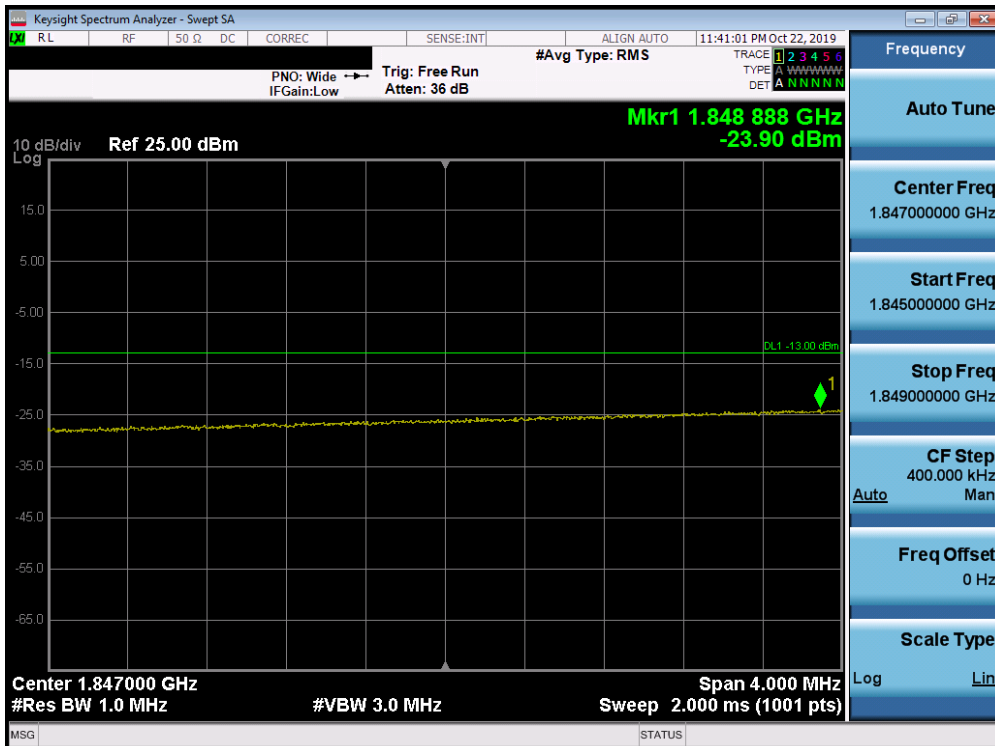
Plot 7-307. Lower Extended Band Edge Plot (Band 25/2 - 15.0MHz QPSK - Full RB Configuration)
