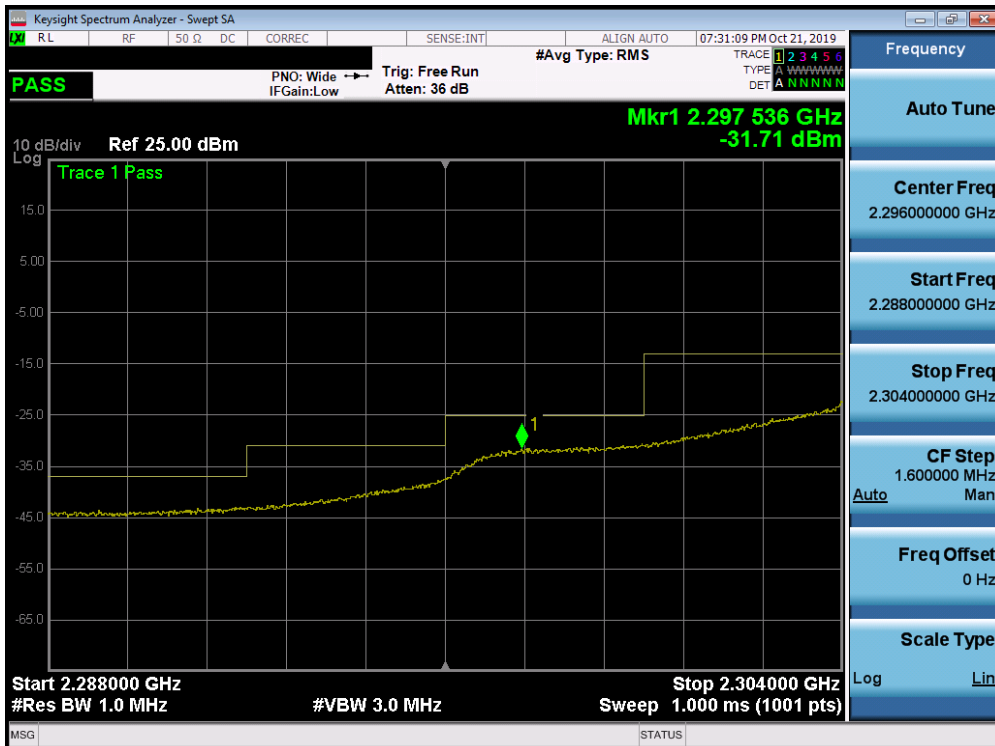
Plot 7-323. Lower Extended Band Edge Plot (Band 30 - 10.0MHz QPSK - Full RB Configuration)
