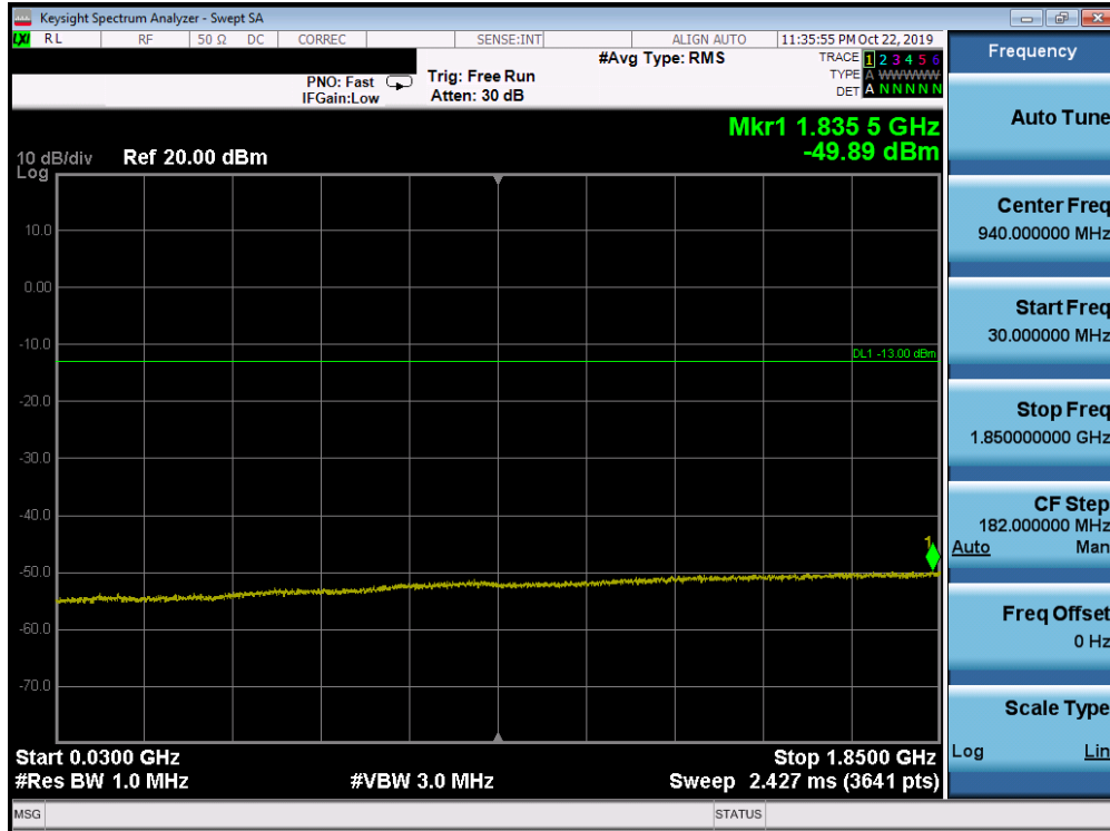
Plot 7-190. Conducted Spurious Plot (Band 25/2 - 20.0MHz QPSK - RB Size 1, RB Offset 0 - High Channel)
