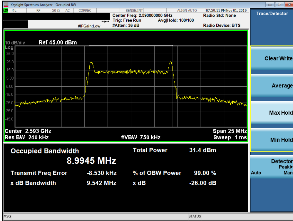
Plot 7-135. Occupied Bandwidth Plot (Band 41 (PC3) - 10.0MHz 64-QAM - Full RB Configuration)
