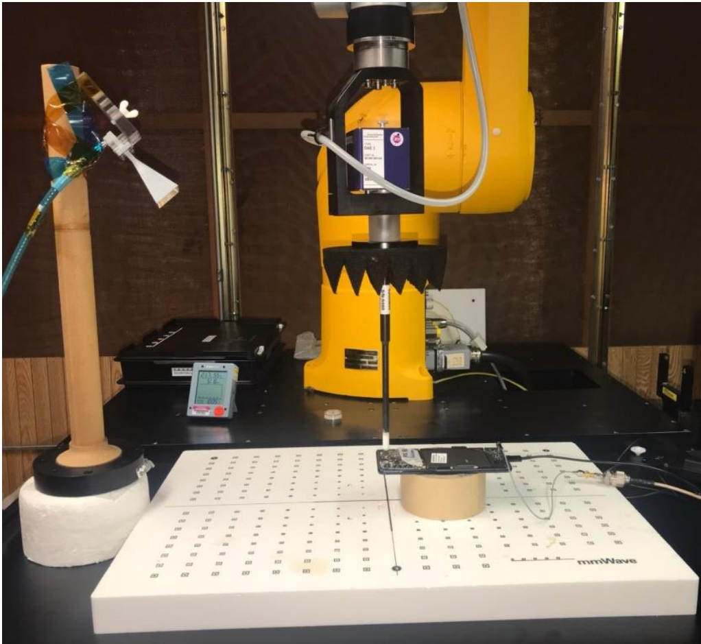
Figure 9-1 Worst-surface of EUT positioned facing up for the mmW beam being tested
