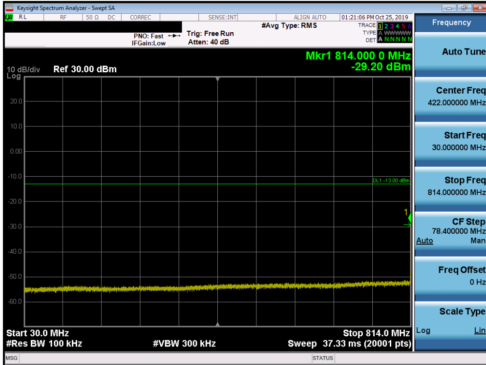
Plot 7-31. Conducted Spurious Plot (LTE Band 26 - 10MHz QPSK - RB Size 1, RB Offset 0 - Mid Channel)
