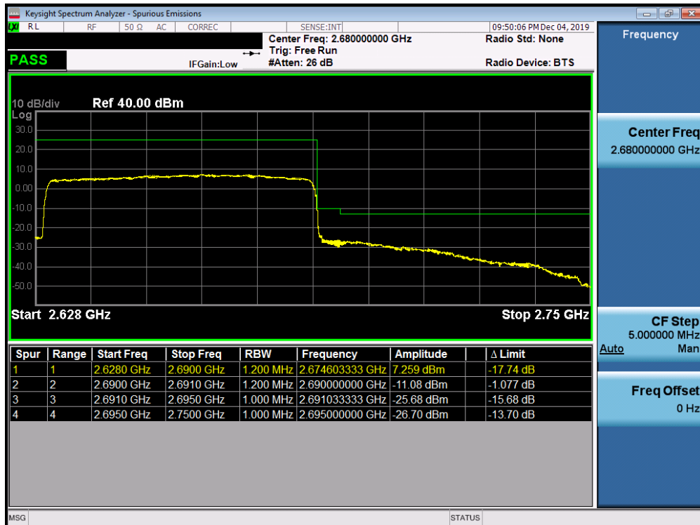
Plot 7-715. Upper ACP Plot (n41 - 60MHz CP-OFDM-QPSK - Full RB Configuration)
