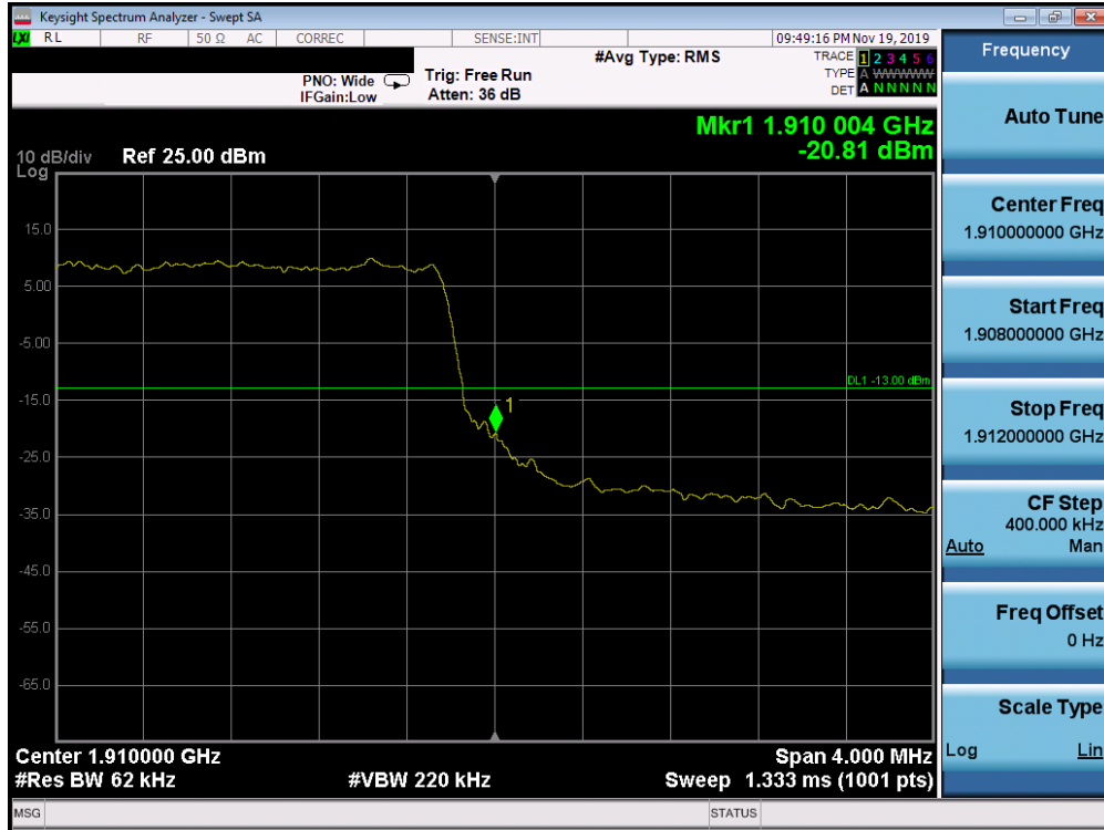
Plot 7-694. Upper Band Edge Plot (Band n2 - 5.0MHz CP-OFDM-QPSK - Full RB Configuration)
