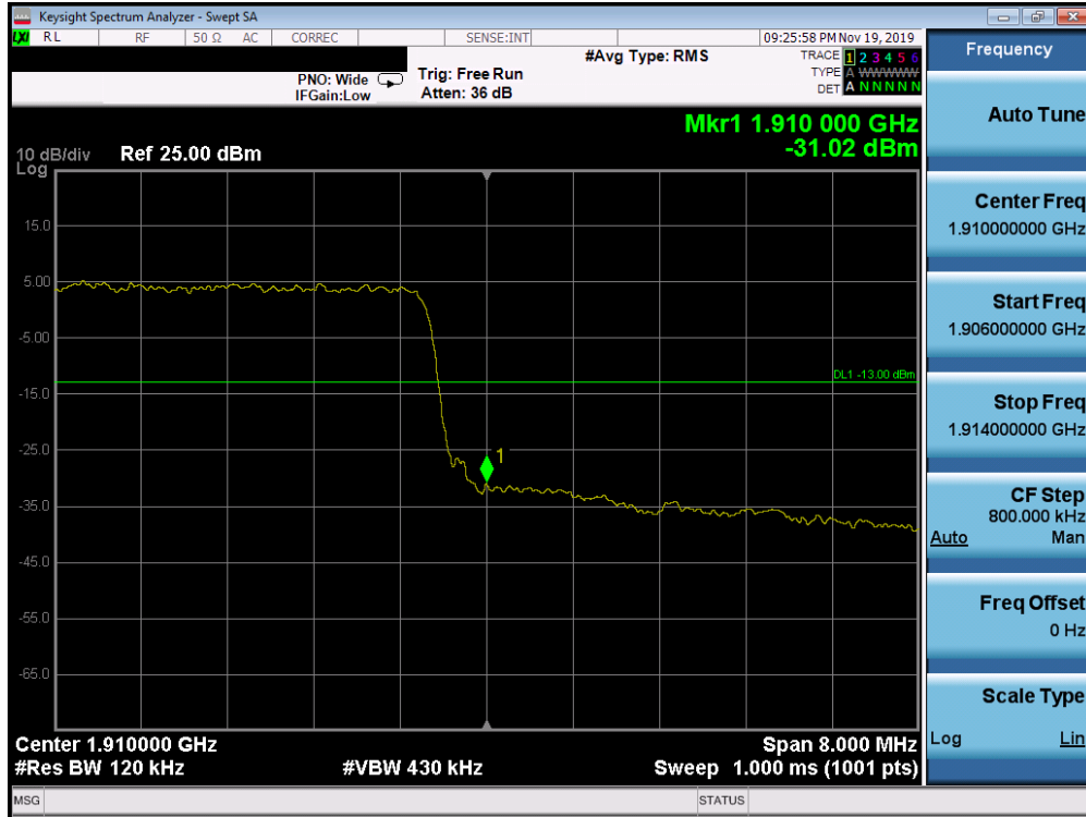
Plot 7-698. Upper Band Edge Plot (Band n2 - 10.0MHz CP-OFDM-QPSK - Full RB Configuration)
