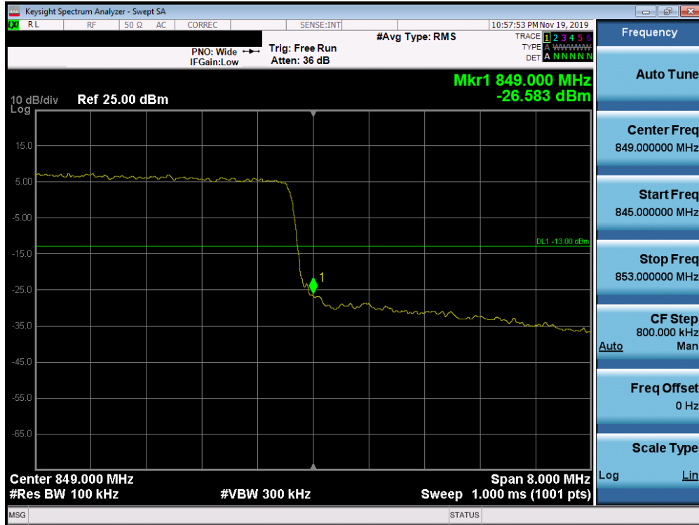
Plot 7-663. Upper Band Edge Plot (n5 - 10MHz CP-OFDM-QPSK - Full RB Configuration)
