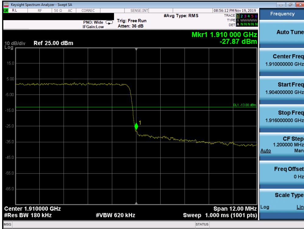
Plot 7-702. Upper Band Edge Plot (Band n2 - 15.0MHz CP-OFDM-QPSK - Full RB Configuration)
