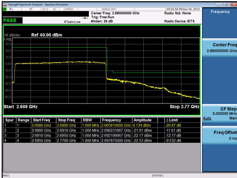
Plot 7-717. Upper ACP Plot (n41 - 80MHz CP-OFDM-QPSK - Full RB Configuration)
