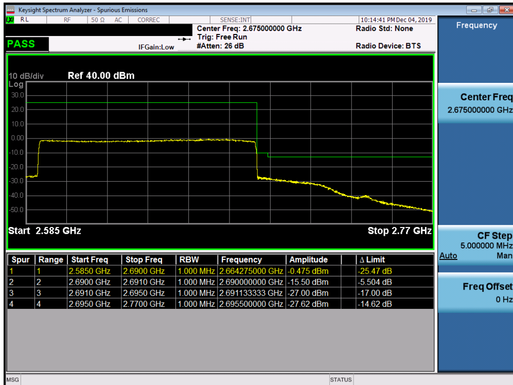
Plot 7-721. Upper ACP Plot (n41 - 100MHz CP-OFDM-QPSK - Full RB Configuration)
