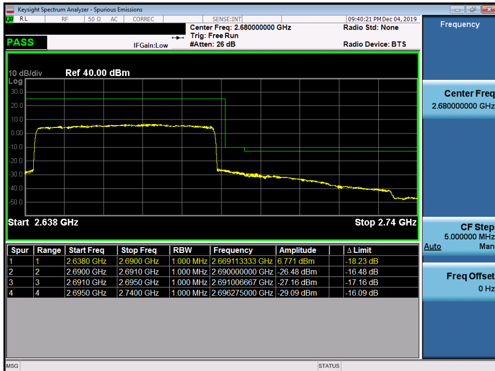
Plot 7-713. Upper ACP Plot (n41 - 50MHz CP-OFDM-QPSK - Full RB Configuration)
