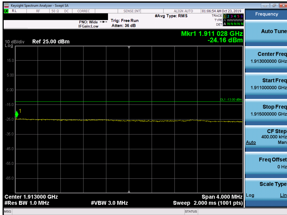
Plot 7-351. Upper Extended Band Edge Plot (Band 2 - 15.0MHz QPSK - Full RB Configuration)
