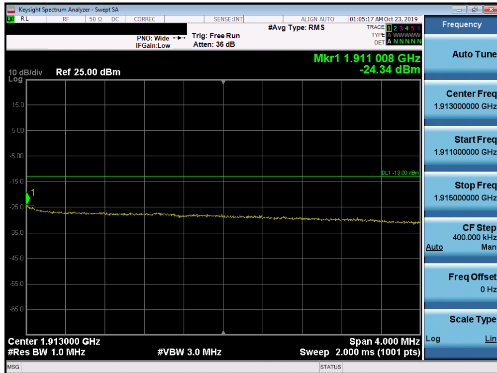
Plot 7-345. Upper Extended Band Edge Plot (Band 2 - 10.0MHz QPSK - Full RB Configuration)
