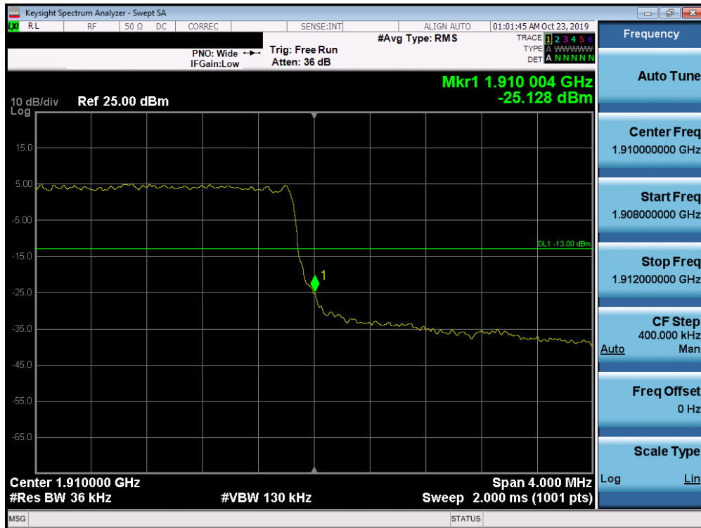
Plot 7-332. Upper Band Edge Plot (Band 2 – 3.0MHz QPSK - Full RB Configuration)
