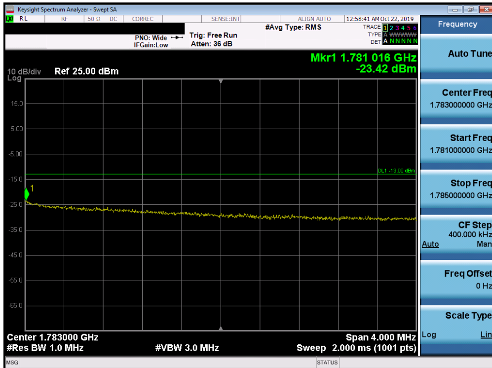
Plot 7-309. Upper Extended Band Edge Plot (Band 66 - 10.0MHz QPSK - Full RB Configuration)
