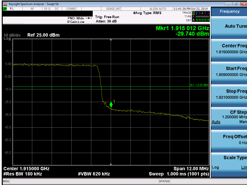
Plot 7-348. Upper Band Edge Plot (Band 25 - 15.0MHz QPSK - Full RB Configuration)
