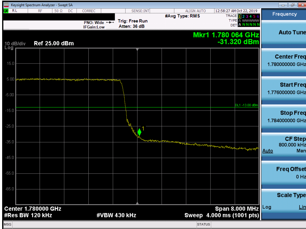
Plot 7-308. Upper Band Edge Plot (Band 66 - 10.0MHz QPSK - Full RB Configuration)
