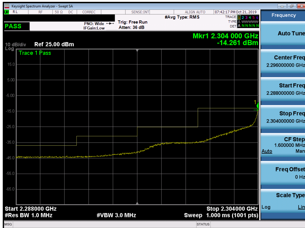
Plot 7-359. Lower Extended Band Edge Plot (Band 30 - 5.0MHz QPSK - Full RB Configuration)
