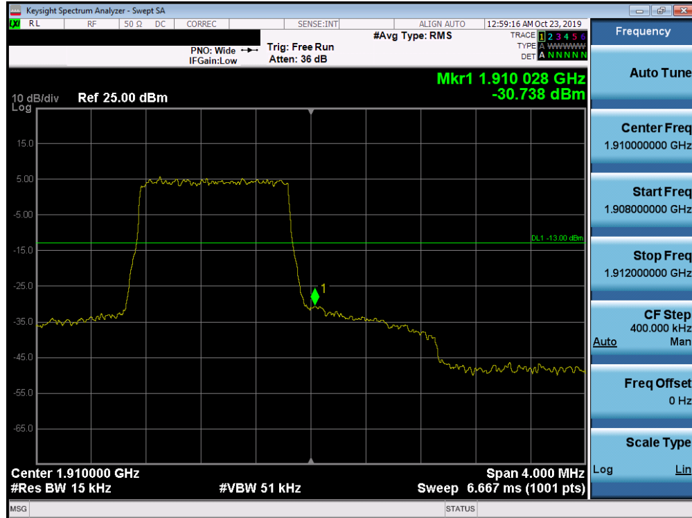
Plot 7-326. Upper Band Edge Plot (Band 2 - 1.4MHz QPSK - Full RB Configuration)
