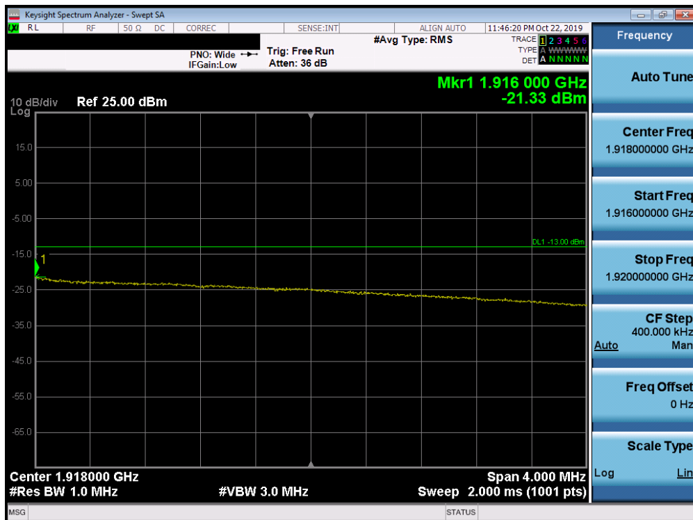
Plot 7-343. Upper Extended Band Edge Plot (Band 25 - 10.0MHz QPSK - Full RB Configuration)
