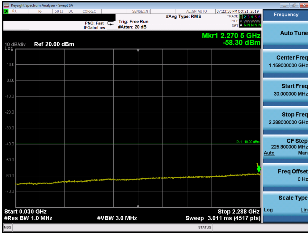
Plot 7-222. Conducted Spurious Plot (Band 30 - 10.0MHz QPSK - RB Size 1, RB Offset 0 - Mid Channel)
