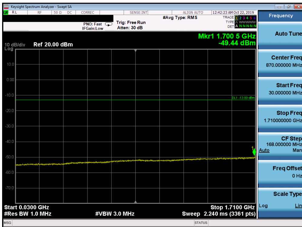
Plot 7-207. Conducted Spurious Plot (Band 66/4 - 20.0MHz QPSK - RB Size 1, RB Offset 0 - Mid Channel)
