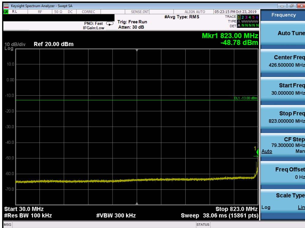
Plot 7-195. Conducted Spurious Plot (Band 26 - 15.0MHz QPSK - RB Size 1, RB Offset 0 - Low Channel)
