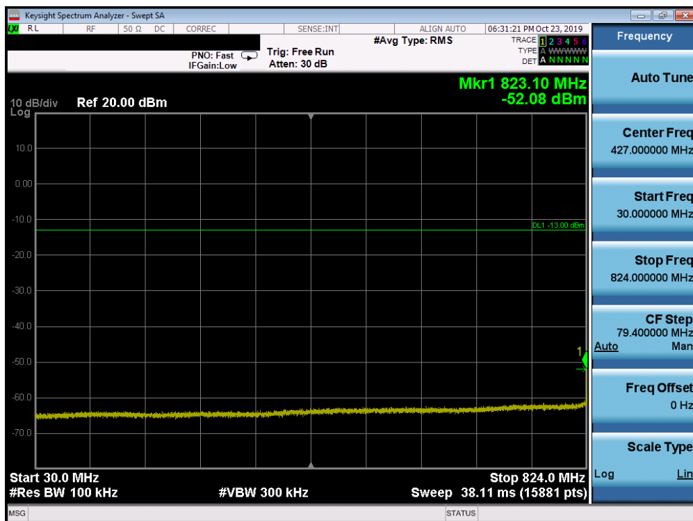
Plot 7-189. Conducted Spurious Plot (Band 26/5 - 10.0MHz QPSK - RB Size 1, RB Offset 0 - Mid Channel)
