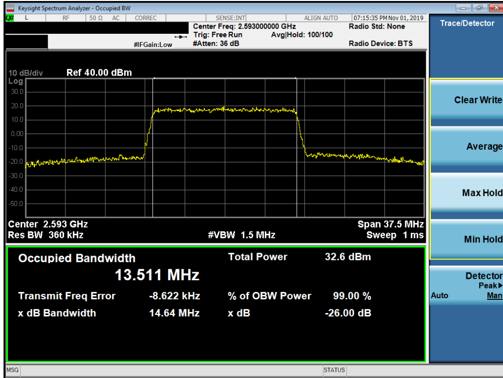
Plot 7-143. Occupied Bandwidth Plot (Band 41 (PC2) - 15.0MHz 64-QAM - Full RB Configuration)
