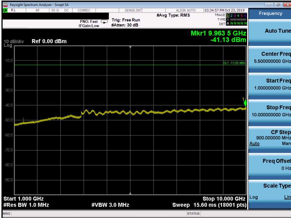
Plot 7-173. Conducted Spurious Plot (Band 71 - 20.0MHz QPSK - RB Size 1, RB Offset 0 - High Channel)
