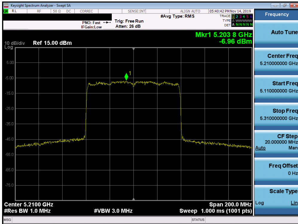
Plot 7-249. Power Spectral Density Plot MIMO ANT2 (80MHz BW 802.11ax – Full Tones (UNII Band 1) – Ch. 42)
