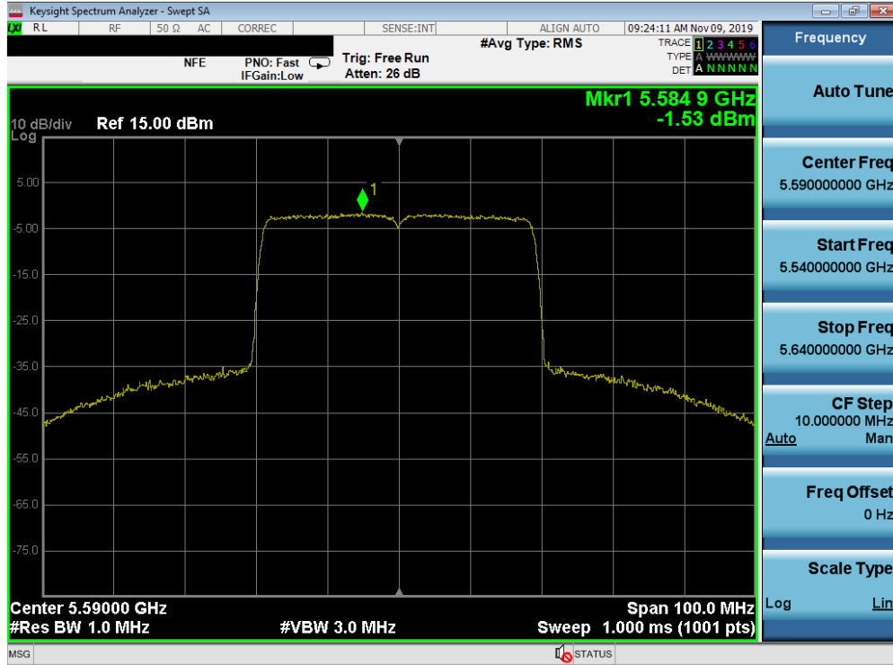
Plot 7-98. Power Spectral Density Plot SISO ANT1 (40MHz BW 802.11ax – Full Tones (UNII Band 2C) – Ch. 118)
