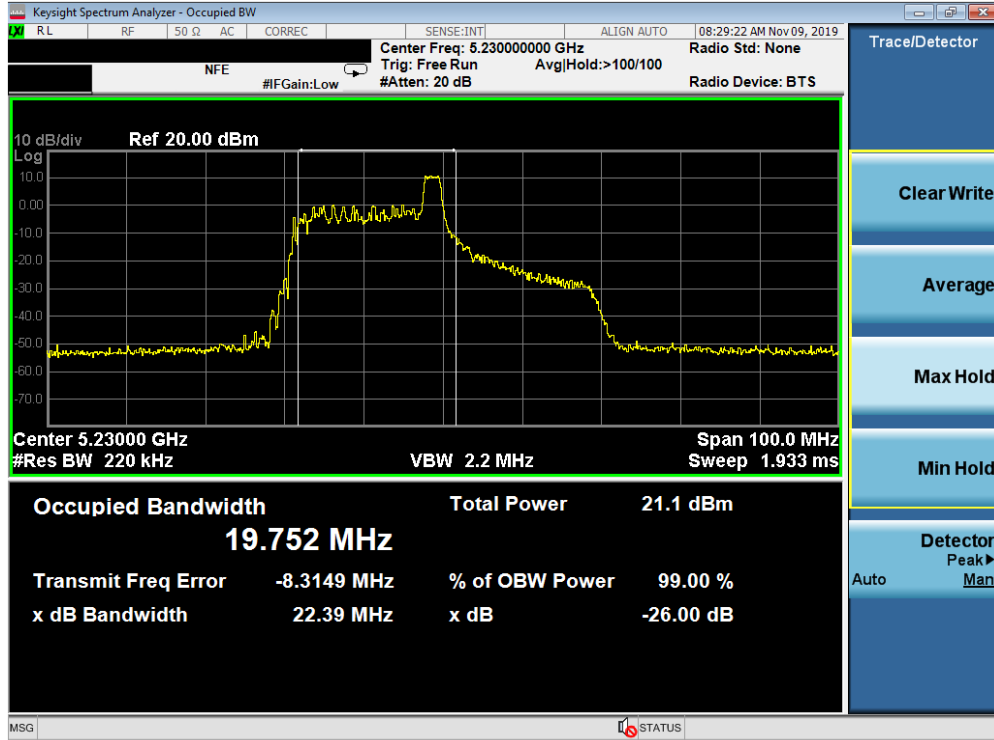
Plot 7-5. 26dB Bandwidth Plot SISO ANT1 (40MHz BW 802.11ax – 26 Tones (UNII Band 1) – Ch. 46)
