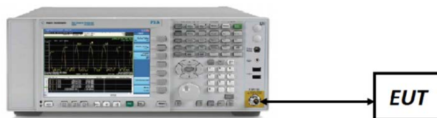
Figure 7-3. Test Instrument & Measurement Setup
