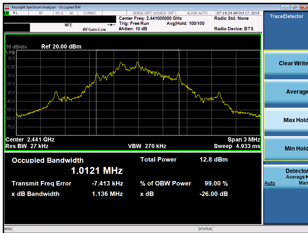
Plot 7-1. Occupied Bandwidth Plot (ANT+ – Ch. 39)
