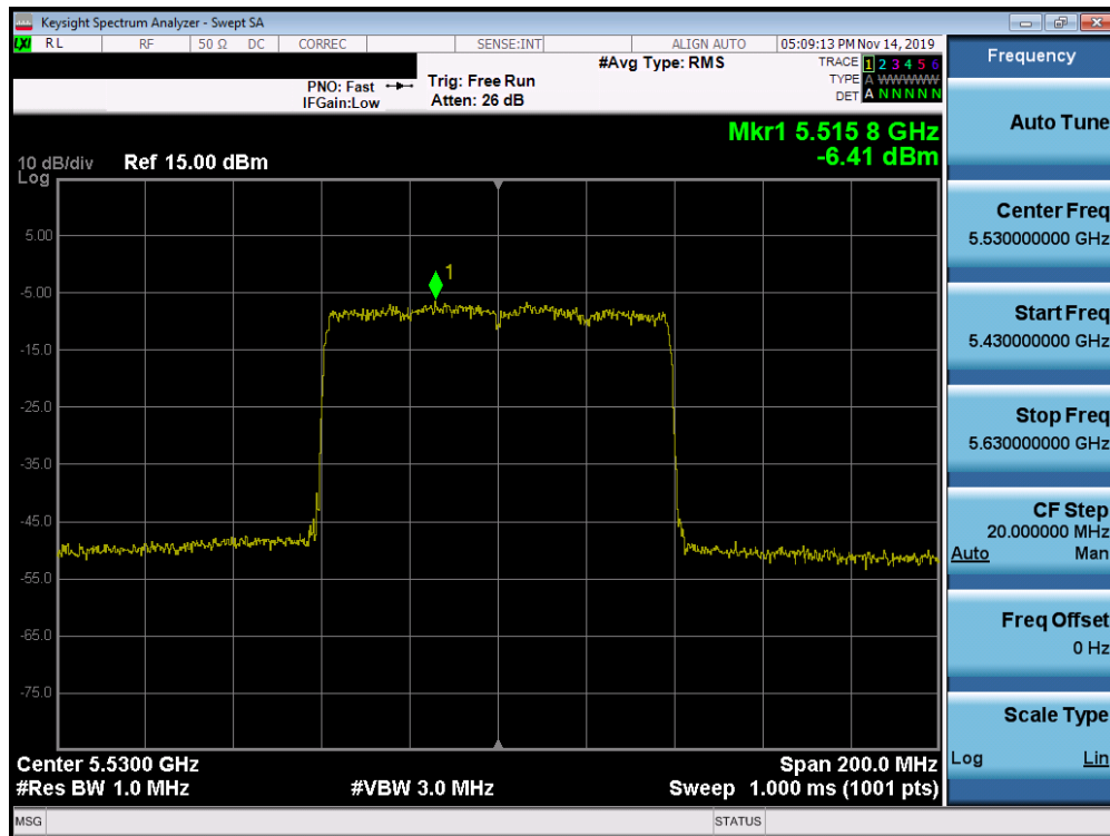
Plot 7-208. Power Spectral Density Plot MIMO ANT1 (80MHz BW 802.11ax – Full Tones (UNII Band 2C) – Ch. 106)
