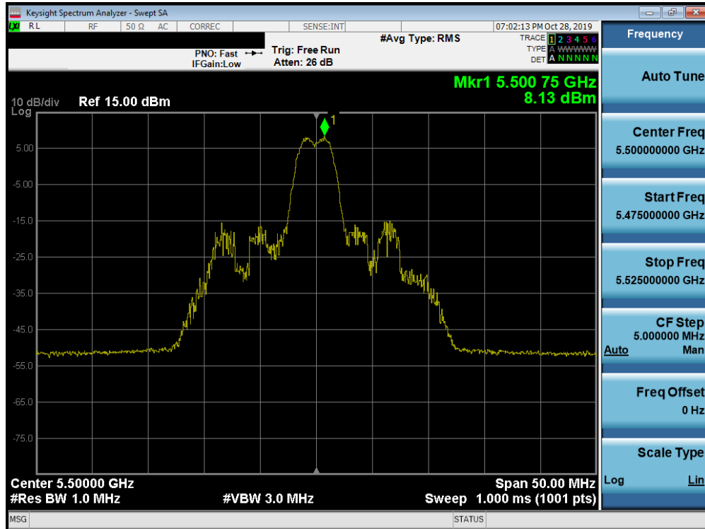
Plot 7-121. Power Spectral Density Plot SISO ANT2 (20MHz BW 802.11ax – 26 Tones (UNII Band 2C) – Ch. 100)
