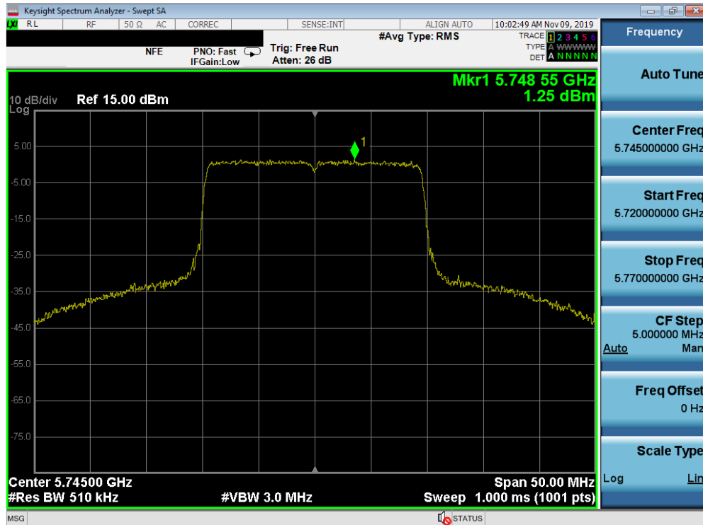
Plot 7-157. Power Spectral Density Plot SISO ANT2 (20MHz BW 802.11ax – Full Tones (UNII Band 3) – Ch. 149)
