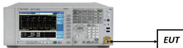
Figure 7-2. Test Instrument & Measurement Setup
