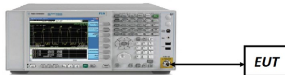
Figure 7-1. Test Instrument & Measurement Setup
