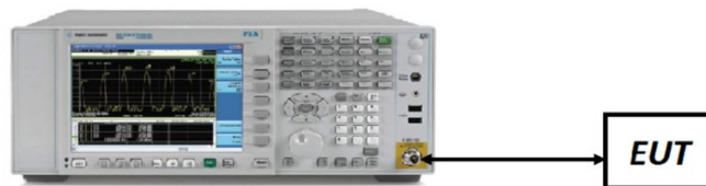
Figure 7-5. Test Instrument & Measurement Setup
