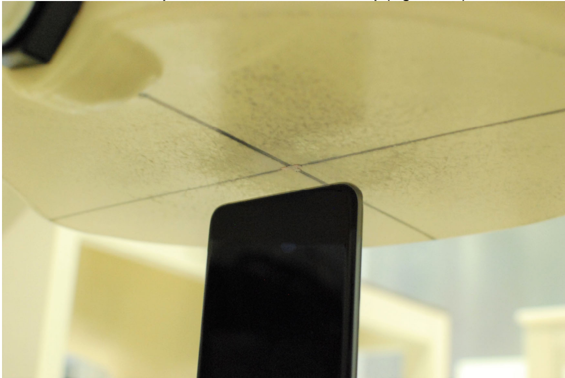
Test Setup Photo 4 – Bottom Edge SAR at 10 mm
