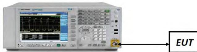
**Figure 7-2. Test Instrument & Measurement Setup**
