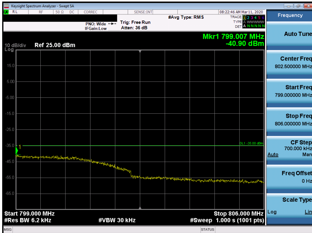
Plot 7-50. Upper Extended Band Edge Plot (Band 14 - 5MHz QPSK - Full RB Configuration)
