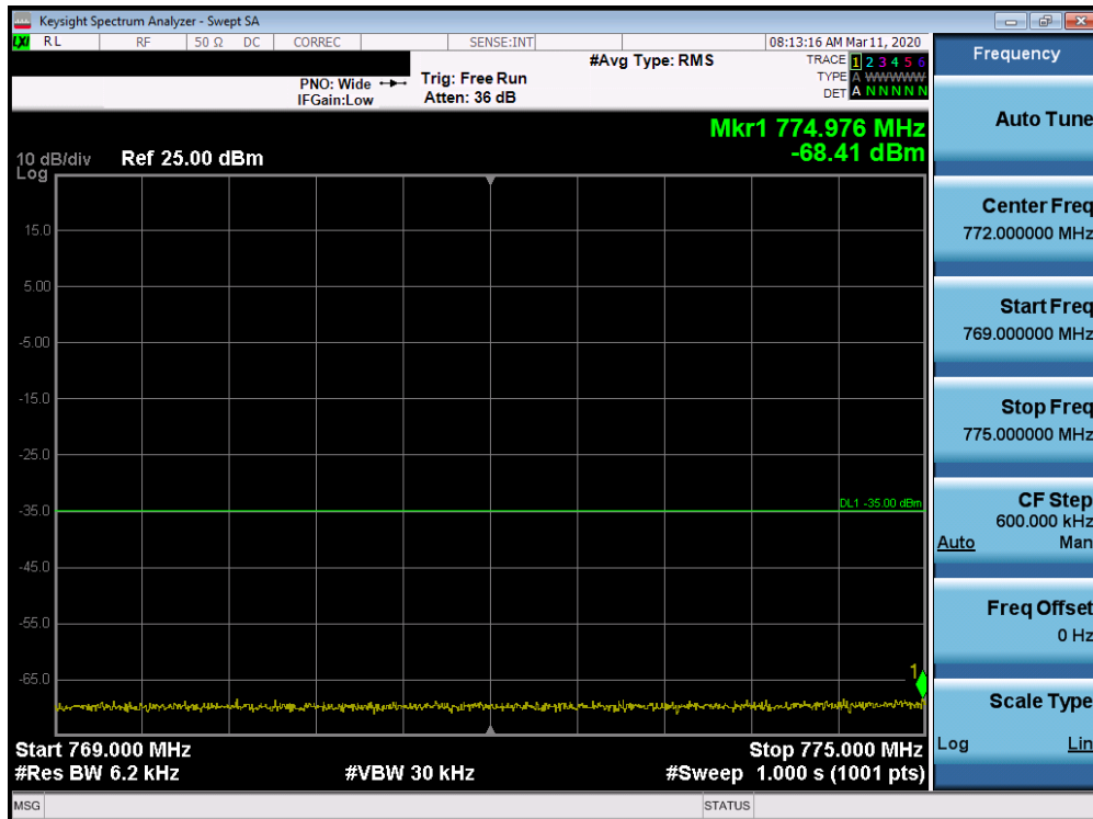
Plot 7-44. Lower Extended Band Edge Plot (Band 14 - 10MHz QPSK - Full RB Configuration)
