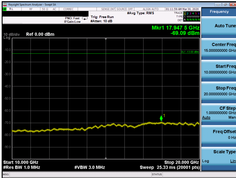
Plot 7-232. Conducted Spurious Plot (n66 - 20.0MHz DFT-s-OFDM BPSK - RB Size 1, RB Offset 0 - High Channel)
