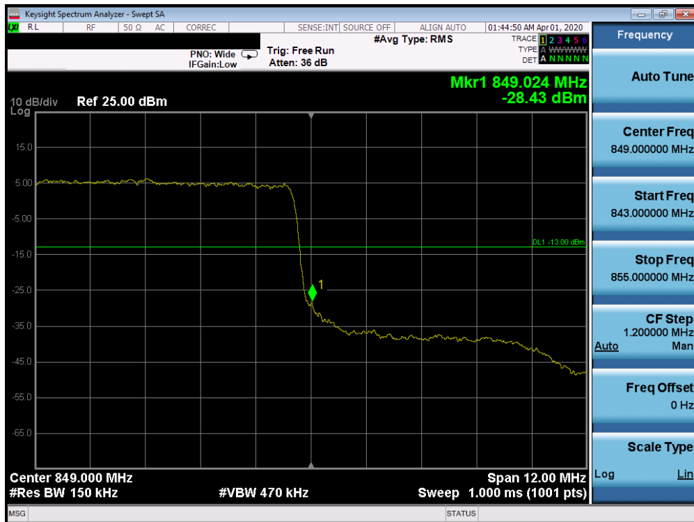
Plot 7-296. Upper Band Edge Plot (n5 – 15.0MHz DFT-s-OFDM BPSK - Full RB Configuration)
