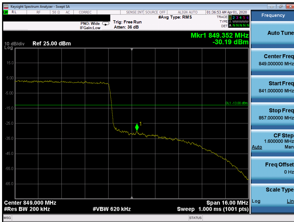
Plot 7-298. Upper Band Edge Plot (n5 – 20.0MHz DFT-s-OFDM BPSK - Full RB Configuration)
