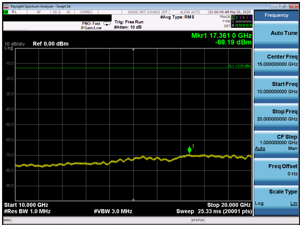
Plot 7-226. Conducted Spurious Plot (n66 - 20.0MHz DFT-s-OFDM BPSK - RB Size 1, RB Offset 0 - Low Channel)
