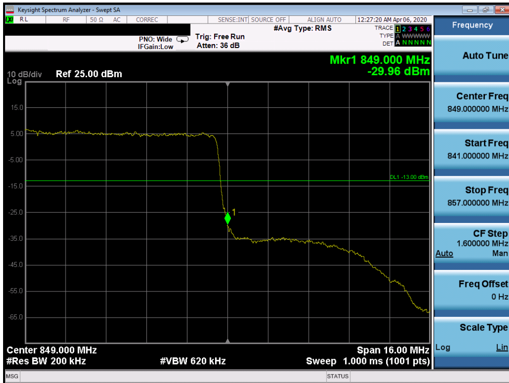
Plot 7-72. Upper Band Edge Plot (n5 - 20.0MHz DFT-s OFDM \pi/2 BPSK - Full RB Configuration)
