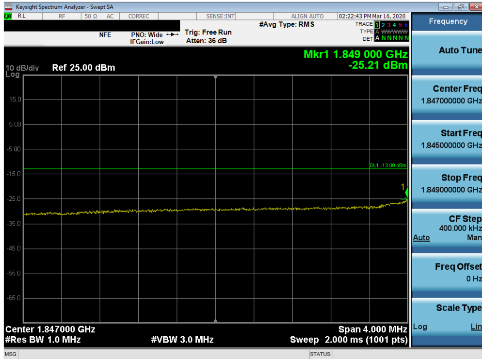
Plot 7-78. Lower Extended Band Edge Plot (n2 - 20.0MHz DFT-s OFDM \pi/2 BPSK - Full RB Configuration)
