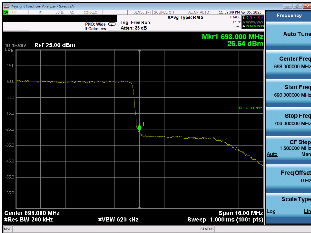
Plot 7-70. Upper Band Edge Plot (n71 - 20.0MHz DFT-s OFDM \pi/2 BPSK - Full RB Configuration)
