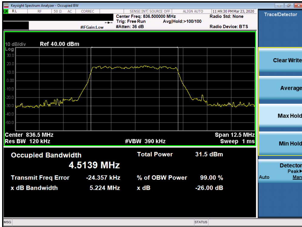
Plot 7-5. Occupied Bandwidth Plot (n5 - 5.0MHz DFT-s OFDM \pi/2 BPSK - Full RB Configuration)
