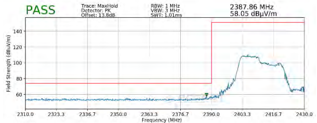
Plot 7-86. Radiated Restricted Lower Band Edge Measurement SISO ANT2 (Peak – 106 Tones)
