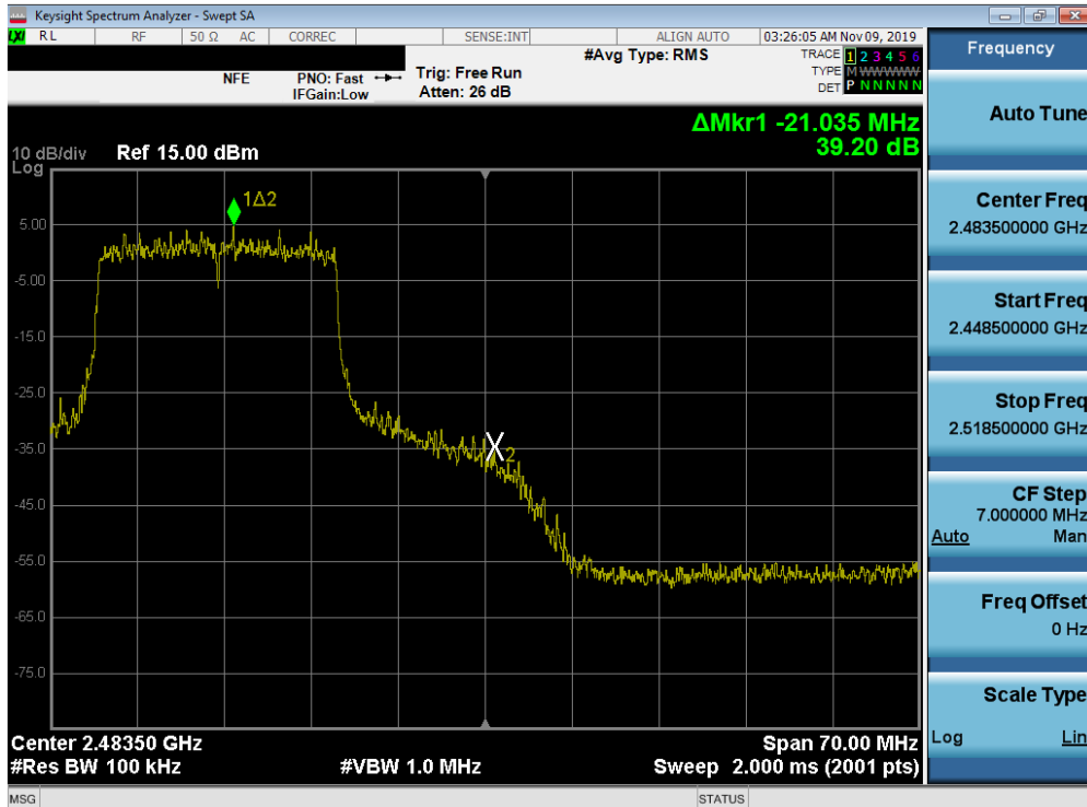
Plot 7-26. Band Edge Plot SISO ANT1 (802.11ax OFDMA – 242 Tones – Ch. 11)
