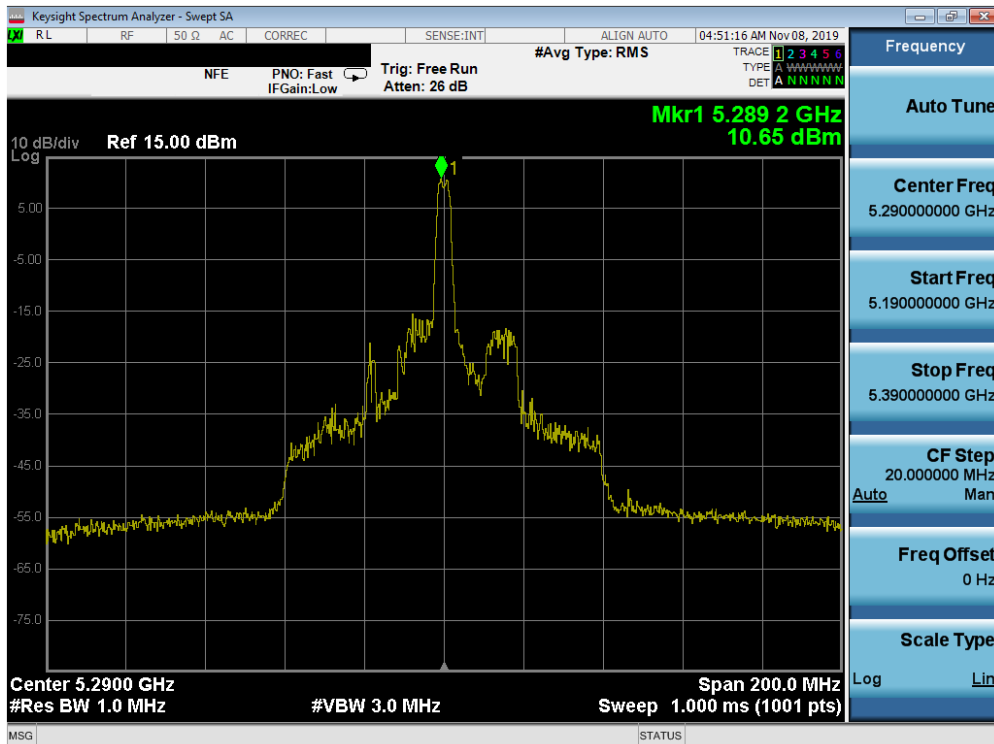
Plot 7-120. Power Spectral Density Plot SISO ANT2 (80MHz BW 802.11ax – 26 Tones (UNII Band 2A) – Ch. 58)
