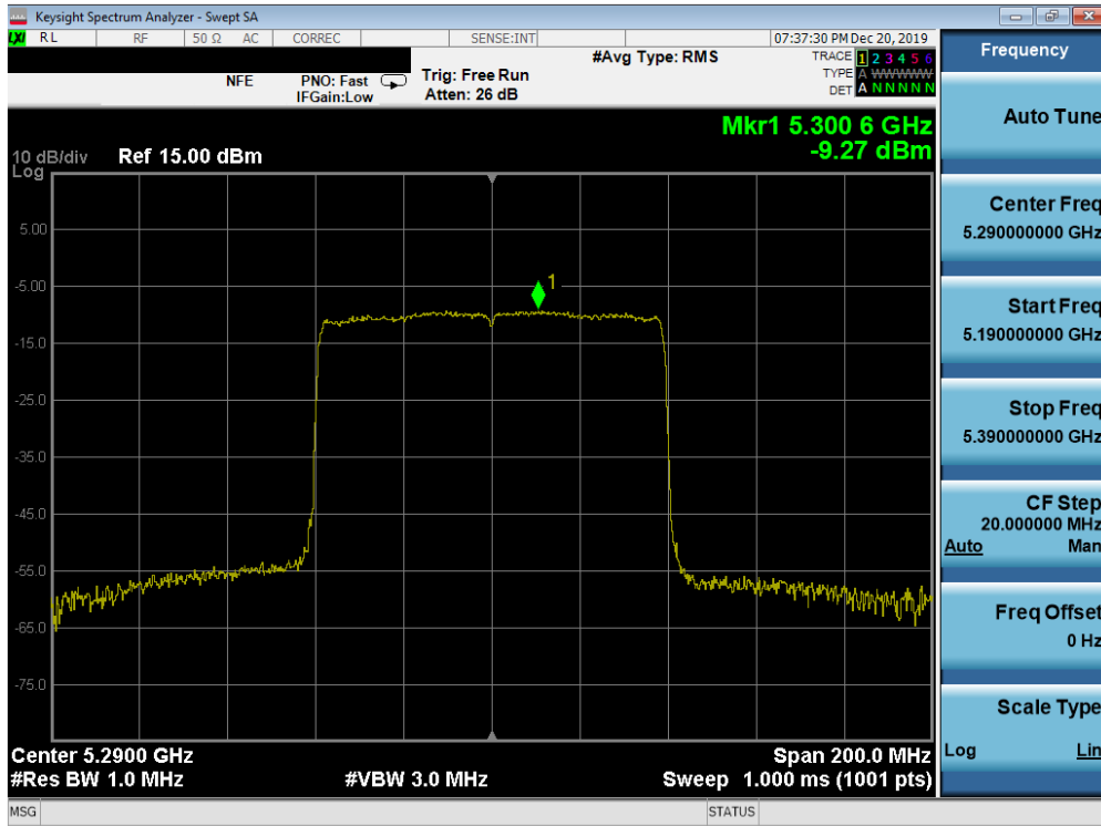
Plot 7-201. Power Spectral Density Plot MIMO ANT1 (80MHz BW 802.11ax – Full Tones (UNII Band 2A) – Ch. 58)
