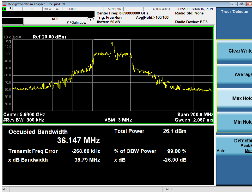
Plot 7-36. 26dB Bandwidth Plot SISO ANT2 (20MHz BW 802.11ax – 26 Tones (UNII Band 2C) – Ch. 144)
