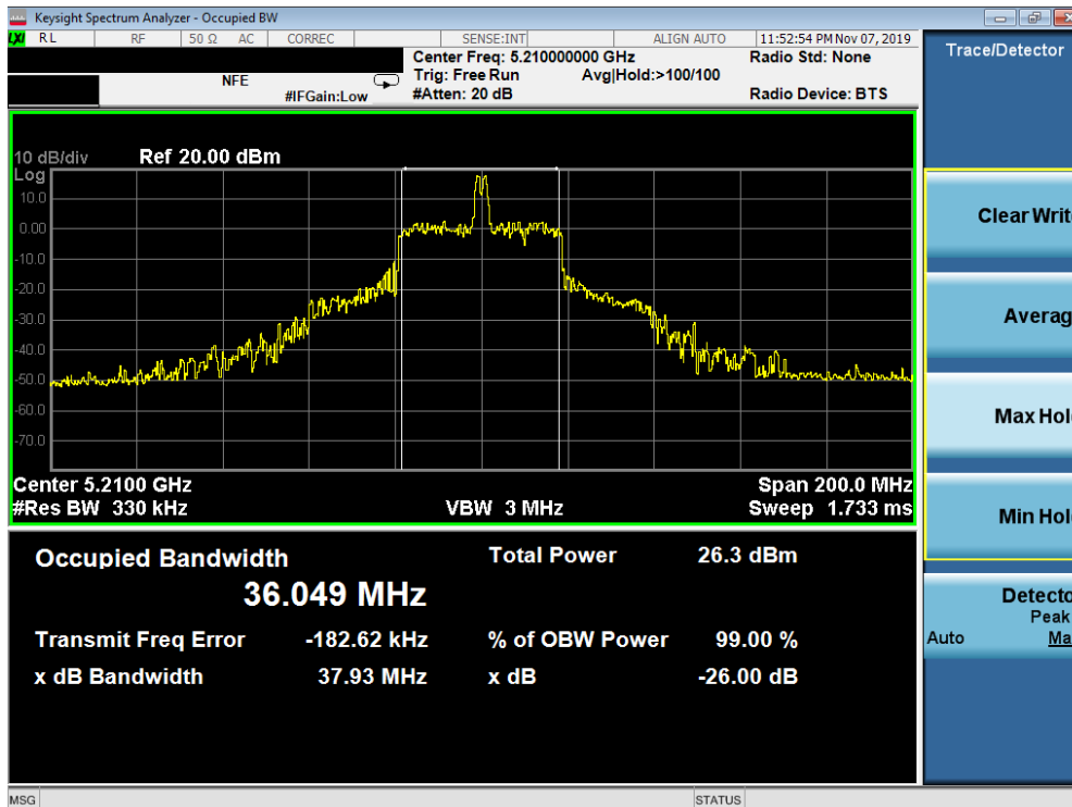
Plot 7-27. 26dB Bandwidth Plot SISO ANT2 (80MHz BW 802.11ax – 26 Tones (UNII Band 1) – Ch. 42)
