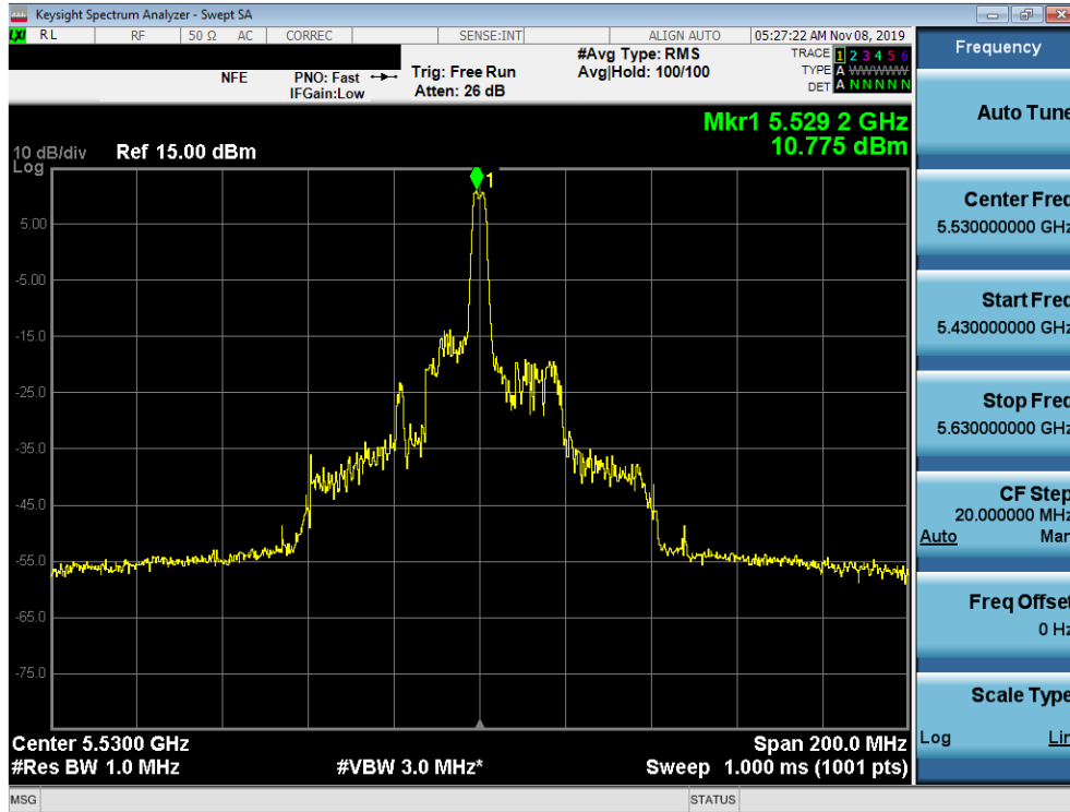
Plot 7-73. Power Spectral Density Plot SISO ANT1 (80MHz BW 802.11ax – 26 Tones (UNII Band 2C) – Ch. 106)
