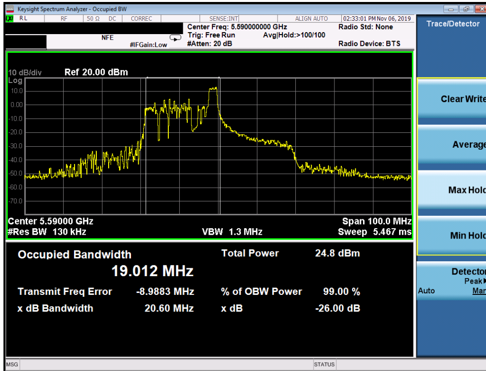
Plot 7-17. 26dB Bandwidth Plot SISO ANT1 (40MHz BW 802.11ax – 26 Tones (UNII Band 2C) – Ch. 118)
