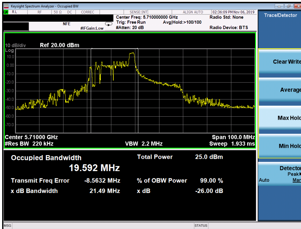
Plot 7-18. 26dB Bandwidth Plot SISO ANT1 (40MHz BW 802.11ax – 26 Tones (UNII Band 2C) – Ch. 142)
