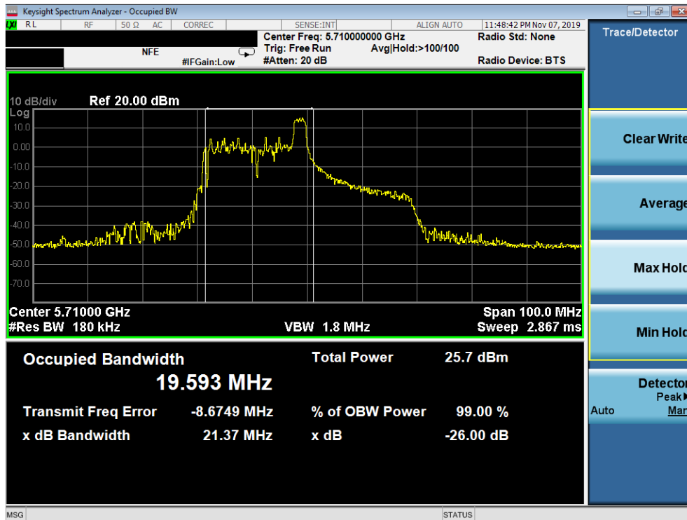
Plot 7-39. 26dB Bandwidth Plot SISO ANT2 (40MHz BW 802.11ax – 26 Tones (UNII Band 2C) – Ch. 142)
