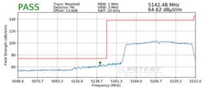
Plot 7-353. Radiated Lower Band Edge Plot MIMO (Peak – UNII Band 1)
