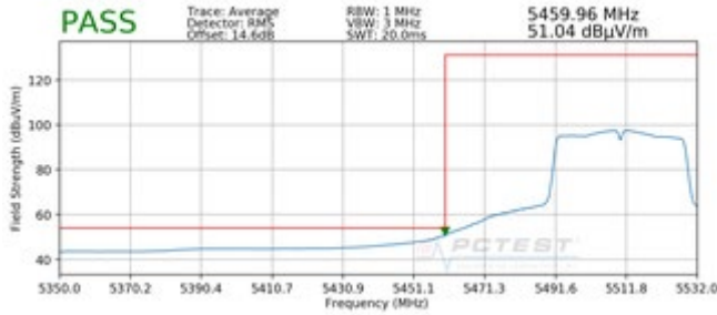
Plot 7-324. Radiated Lower Band Edge Plot SISO ANT2 (Average – UNII Band 2C)
