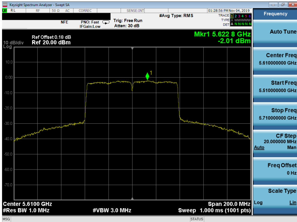
Plot 7-179. Power Spectral Density Plot SISO ANT1 (80MHz BW 802.11ac (UNII Band 2C) – Ch. 122)
