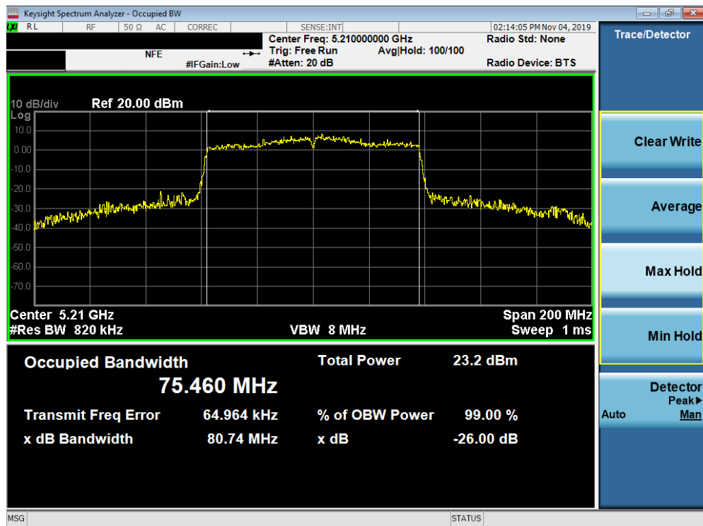
Plot 7-65. 26dB Bandwidth Plot SISO ANT2 (80MHz BW 802.11ac (UNII Band 1) – Ch. 42)
